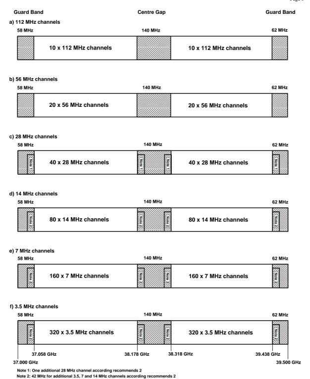
Figure 1: Occupied spectrum 37.0 - 39.5 GHz band
