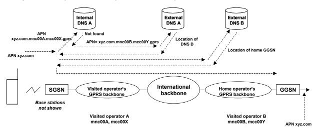
The sequence of interrogations for a roaming mobile is shown in Figure 9.
