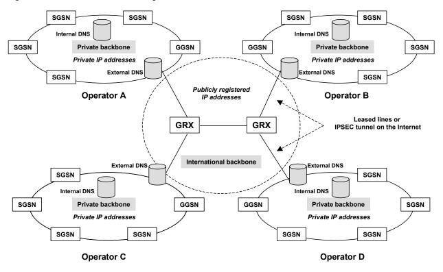
Figure 7 shows the GPRS backbone arrangements.
