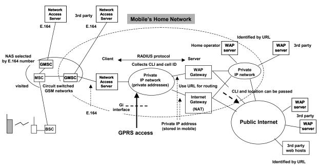
Figure 2: GSM circuit switched access connection
