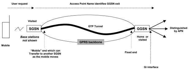
Figure 3: The GPRS access connection
