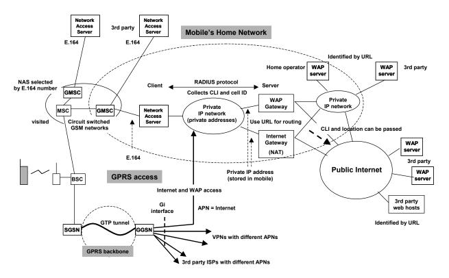
Figure 6: GPRS (non-roaming) and dial-up access to the home network
