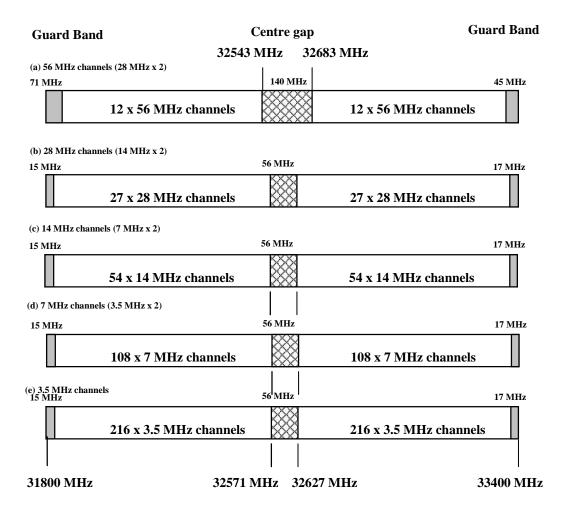
Figure 1: Occupied spectrum: 31.8 to 33.4 GHz Band
