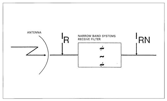
Figure 1. Points where received interference is calculated.
