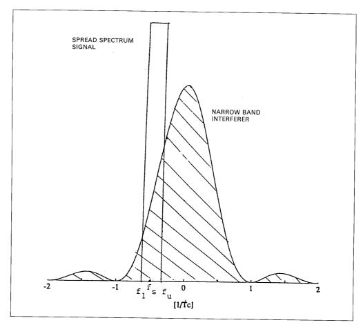
Figure 4. The output from the spread spectrum demodulator.
