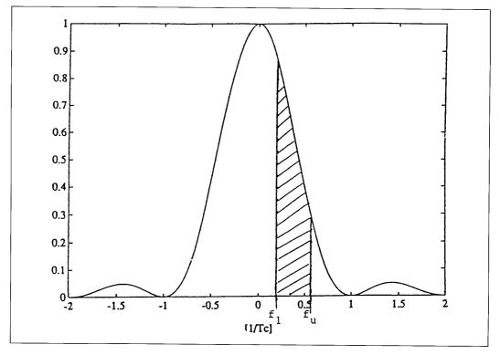
Figure 2. The ideal normalized spectrum of a direct sequence spread spectrum signal.
