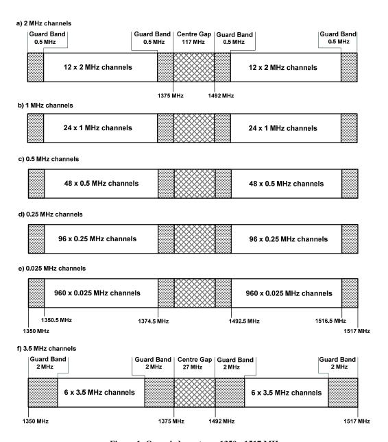
Figure 1: Occupied spectrum 1350 - 1517 MHz
