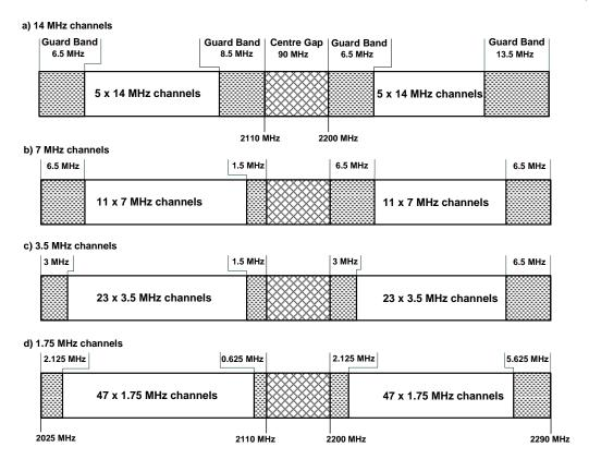
Figure 3: Occupied spectrum 2025 - 2290 MHz
