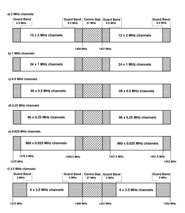
Figure 2: Occupied spectrum 1375 - 1452 MHz
