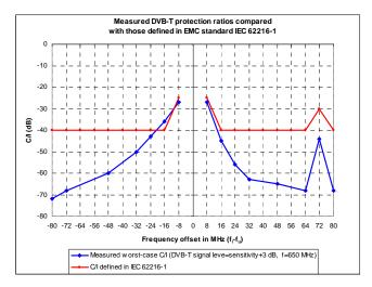
Figure 3: Measured DVB-T protection ratios with a DVB-H interferer compared with those defined in EMC standard IEC 62216-1 [5]
