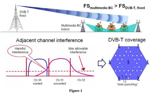
Adjacent channel interference from multimedia broadcasting network into DVB-T service.
