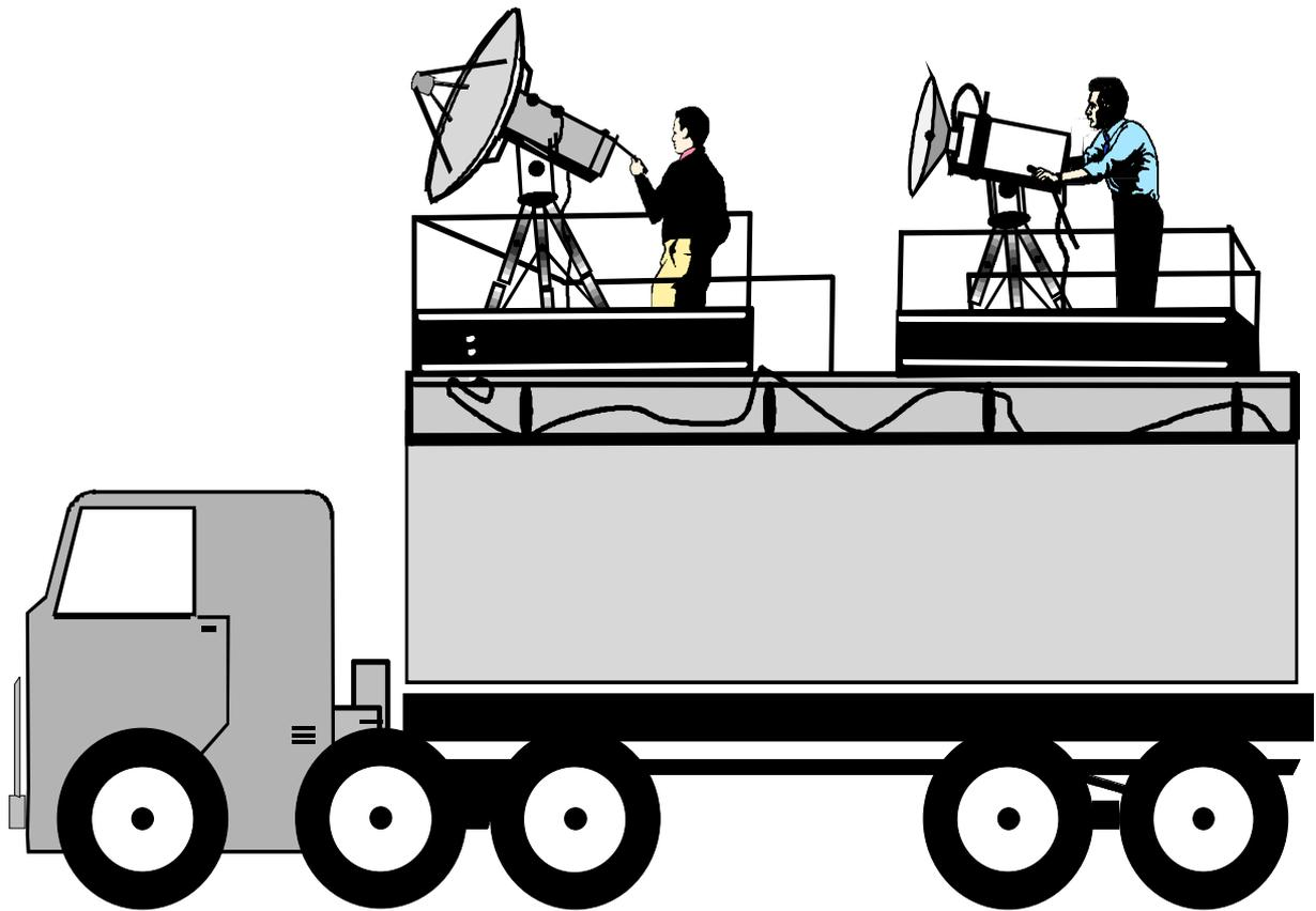
Description: Roof of communications vehicle, a environmentally safe platform with convenient access, so manually tracked antennas are often located here.
