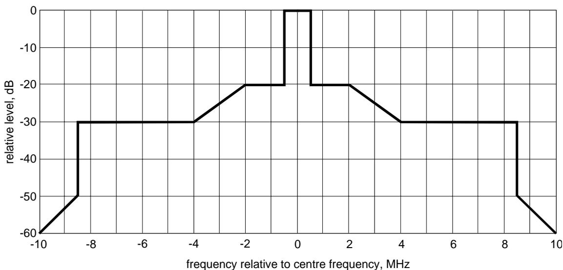
Although the true sense of the spectrum mask is to show relative spectral density (for which a measurement bandwidth of one Hz. is implicit) versus frequency spacing; for all practical purposes a measurement bandwidth of up to 30 kHz is satisfactory.
