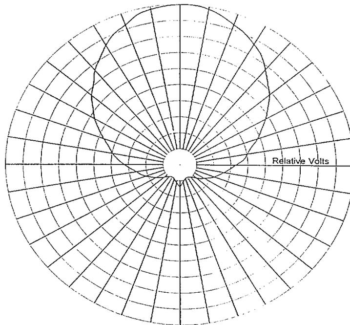
Figures 3 & 4: Radiation Pattern of Low Profile Antenna
