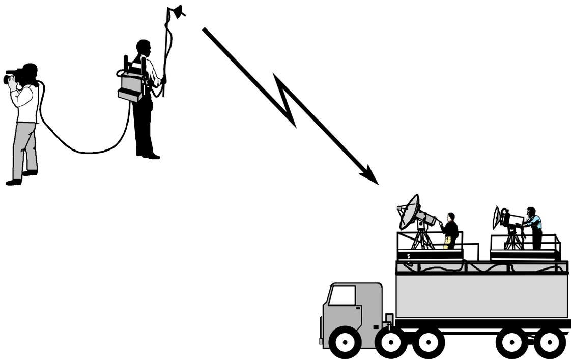
Description: Two man radio camera to roof of communications vehicle
