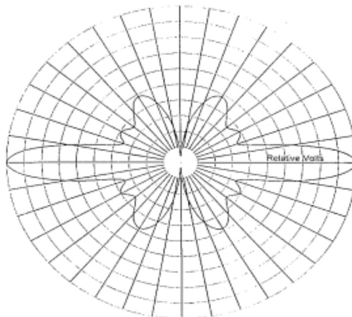
Figures 5 & 6: Radiation Pattern of Franklin Antenna
