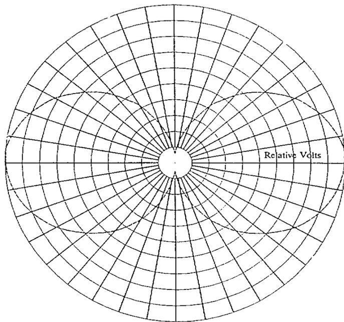
Figures 7 & 8: Radiation Pattern of Bicone Antenna
