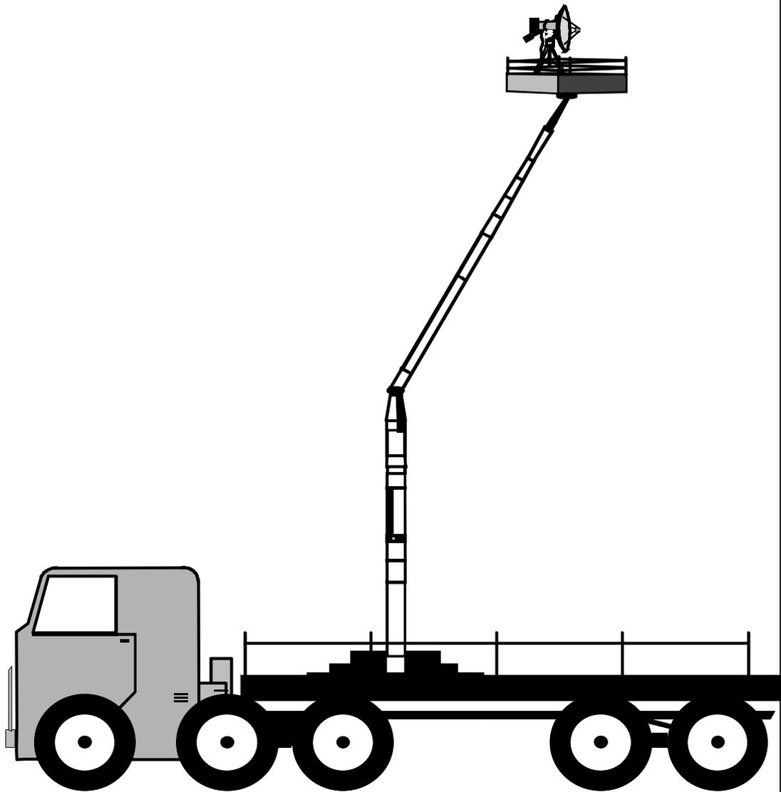
Description: Hydraulically elevated antenna platform
