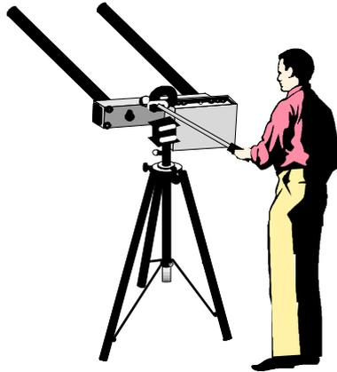
Description: Manually tracked receiving antenna located at any convenient point at ENG/OB site
