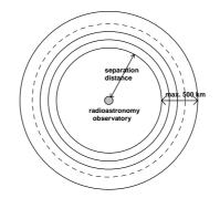
The required separation distance is calculated for 10% of the time of interference.
