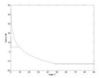
Figure 8: Antenna pattern for cross-polarisation
