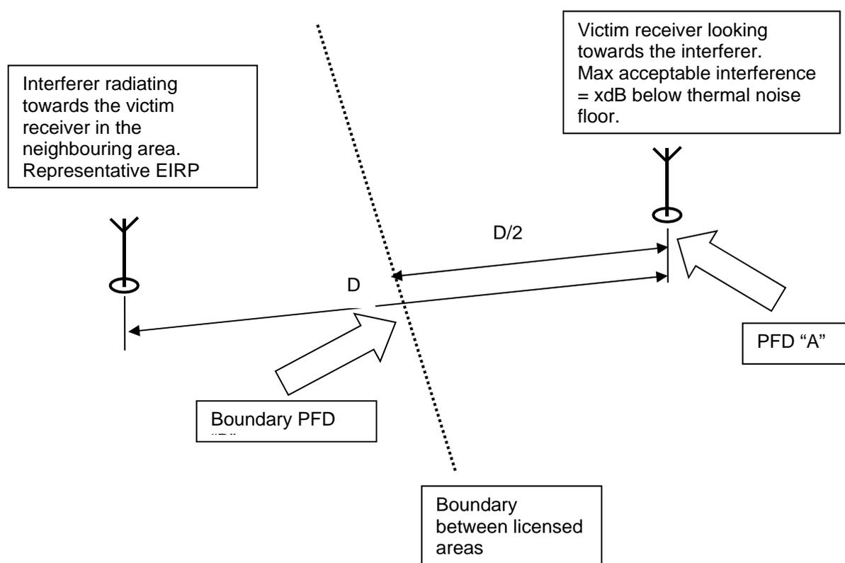
**Figure 10: Example of PFD boundary limit**
