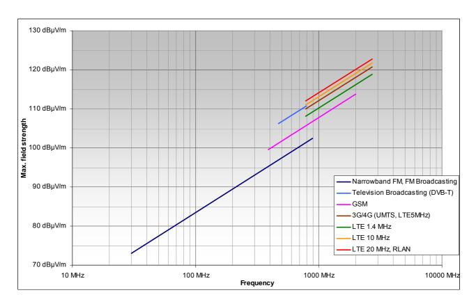
Figure 1: Maximum permissible field strengths when using typical parameter values
