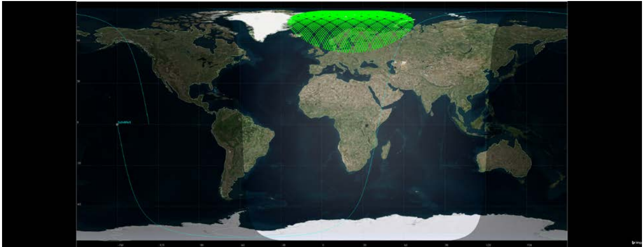
Figure 11: Visibility of the EESS satellite from a given earth station
