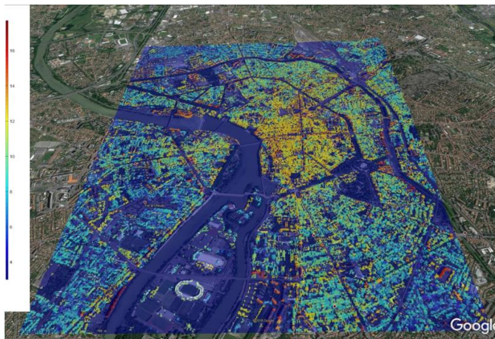
Figure 16: Example of Building Levels in the centre of the City of Toulouse
