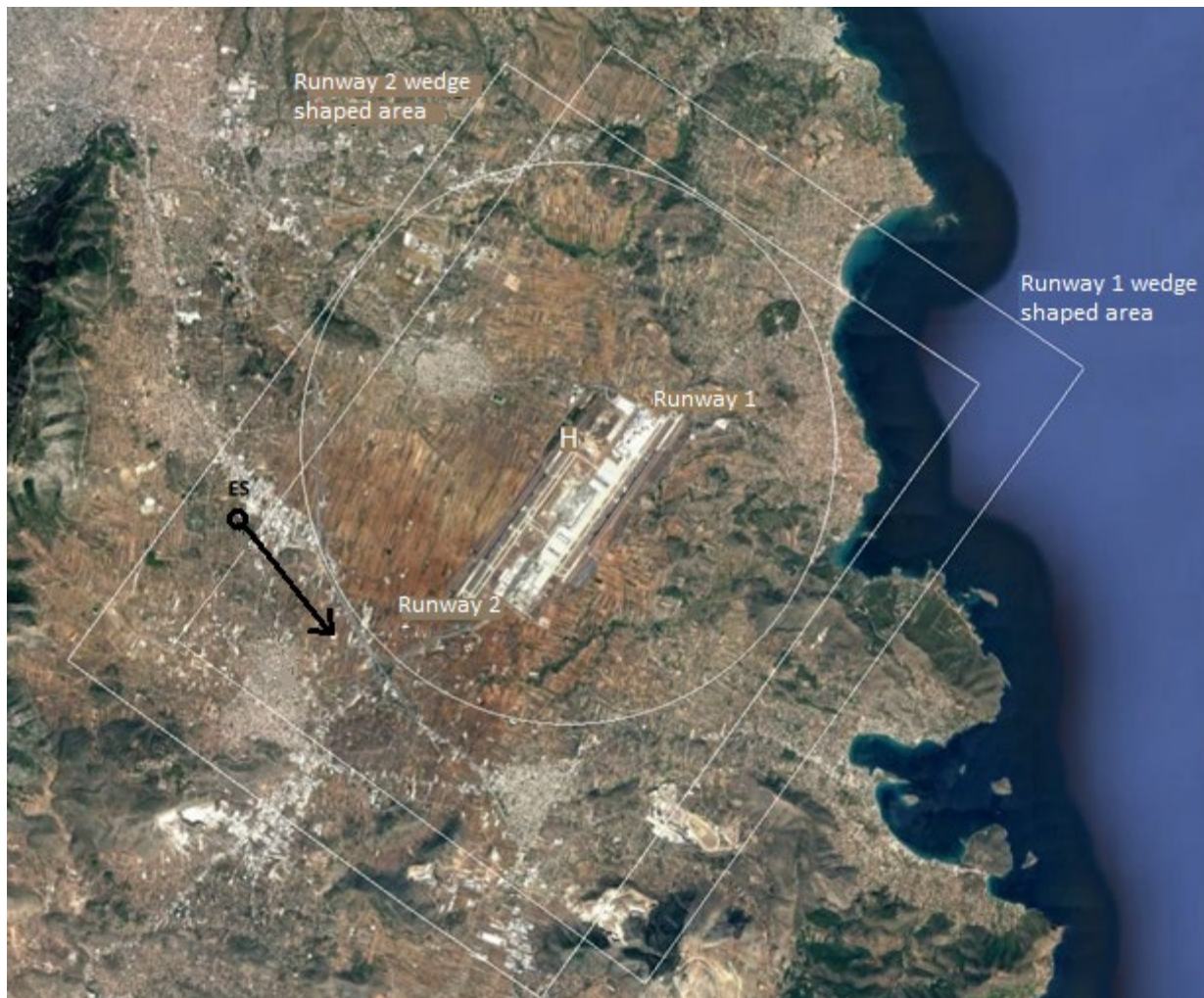
Figure 3: Example location of an earth station within a wedge shaped area of an airfield 6 (depicted as “o” in the figure – the arrow is the direction of the main beam)
