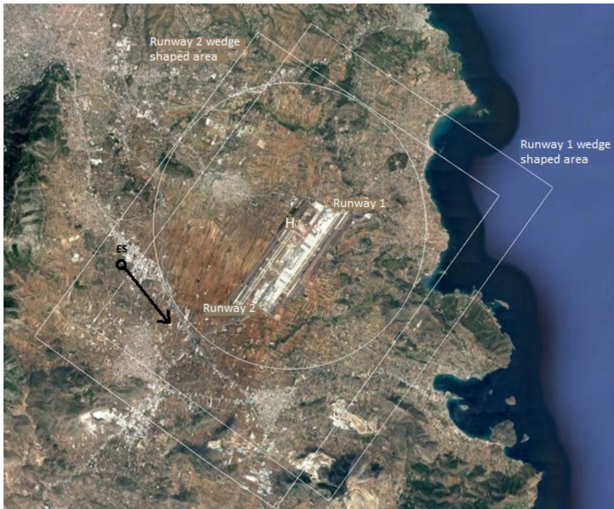
Figure 4: Example location of an earth station within the wedge shaped area of an airfield 7 (depicted as “o” in the figure – the arrow is the direction of the main beam)
