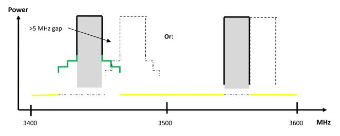
Figure 3: Combined BEM elements for adjacent blocks with unsynchronised and semi-synchronised TDD networks
