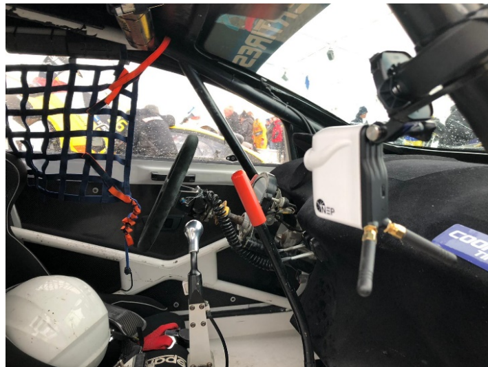
Figure 12: On-board camera mounted inside a car, Porsche Cup
