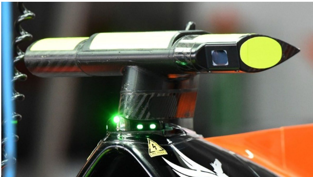
Figure 14: On-board camera, mounted above F1 car's cockpit
