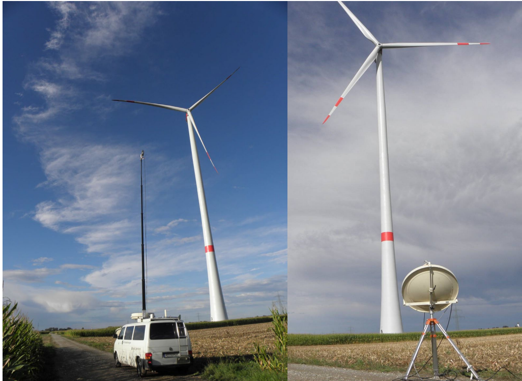
Figure 14: Measurement of wind turbine emission levels (left: at 611 MHz, right: at 1413 MHz)
