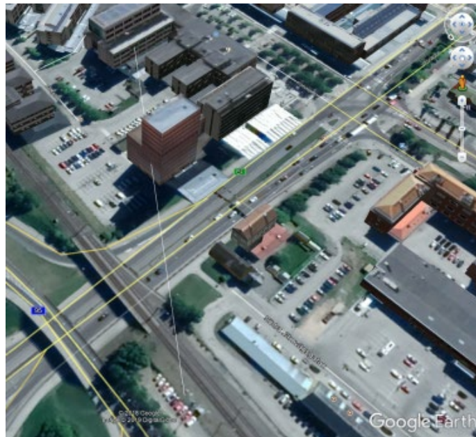
Figure 53: Example of building obstruction between a RMR and a MFCN site in Sweden
