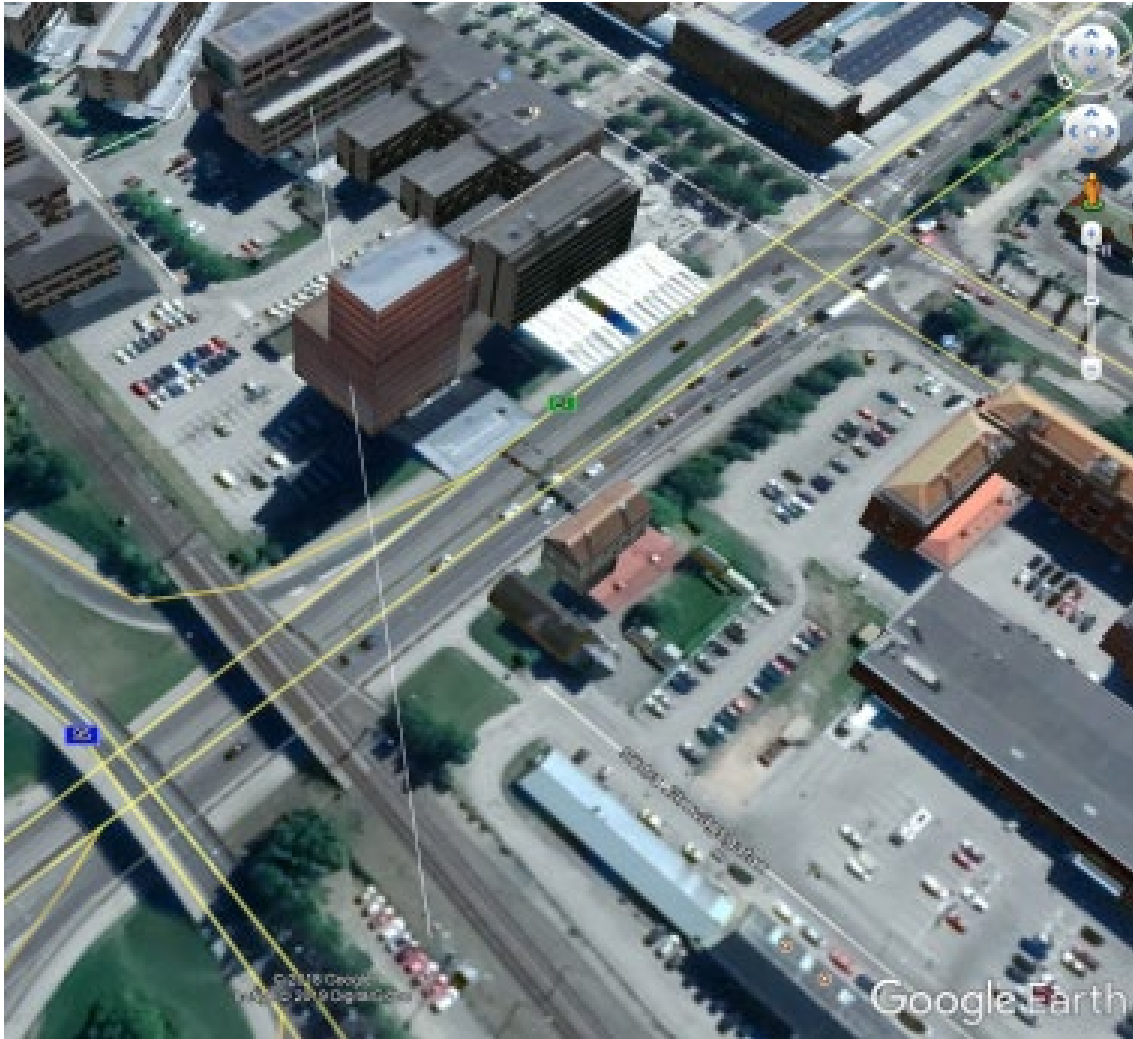
Figure 16: Example of building obstruction between a RMR and a MFCN site in Sweden
