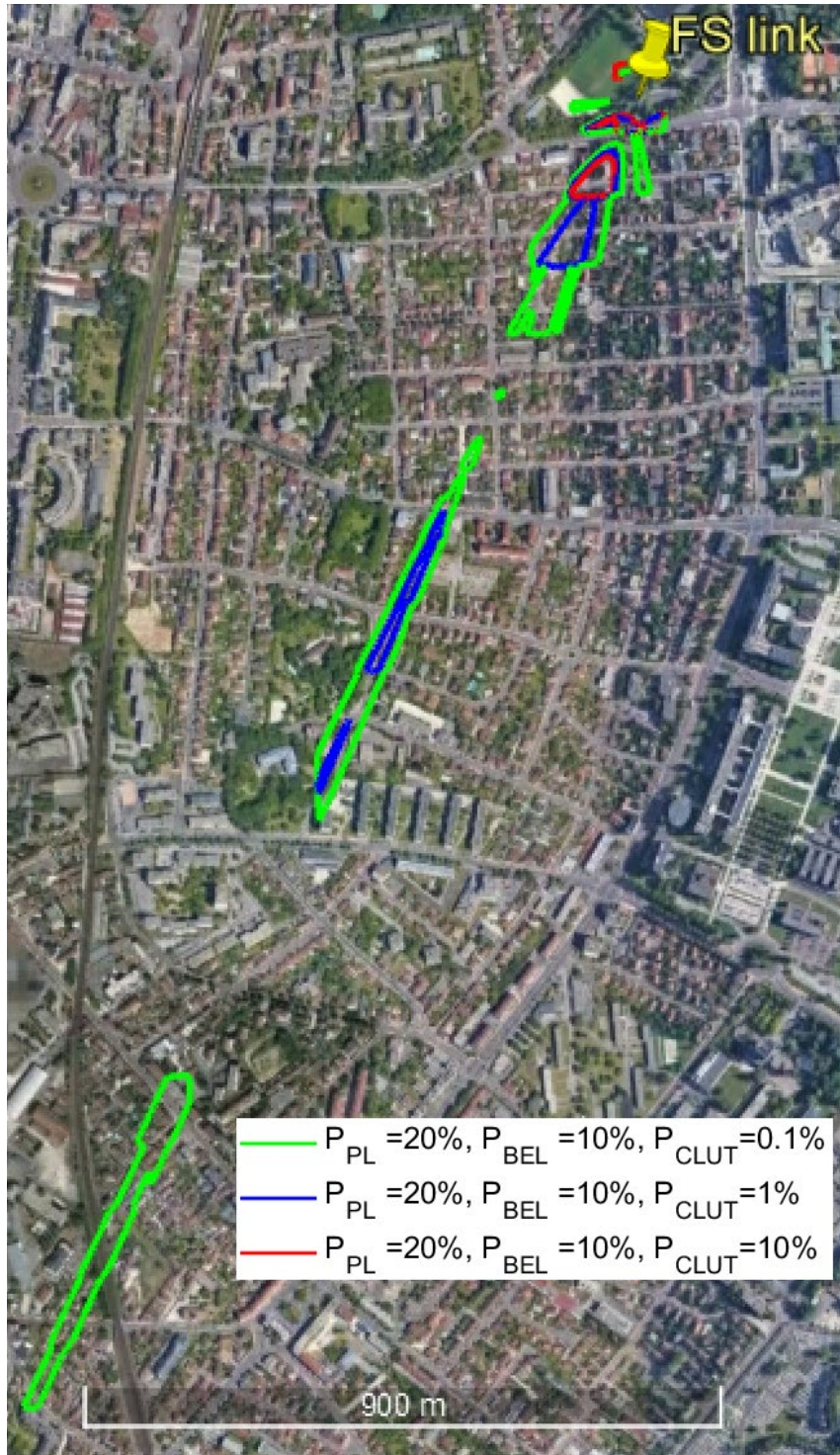
Figure 12: I/N contour for 19 dB value and higher for different clutter loss values. BEL weighted: 70 % Traditional, 30% Thermally efficient. WAS/RLAN power =200 mW, WAS/RLAN height =1.5 m.
