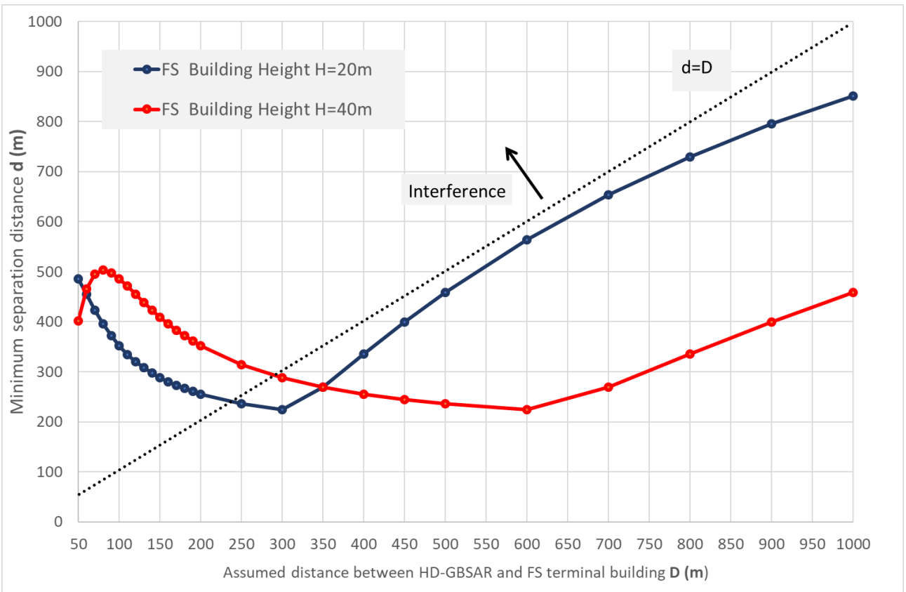
Figure 67: Minimum separation distance in case of horizontal misalignment of \phi_R 18^\circ (case C)
