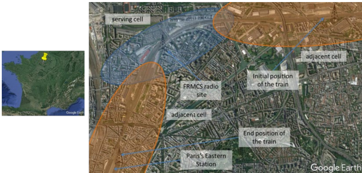
Figure 10: Representative example of a high-density line (Paris's Eastern station in Paris city centre)
