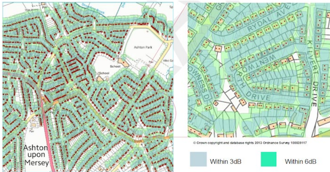
Figure 2: Sample suburban area mapping with 3 dB and 6 dB minimum coupling footprints overlaid
