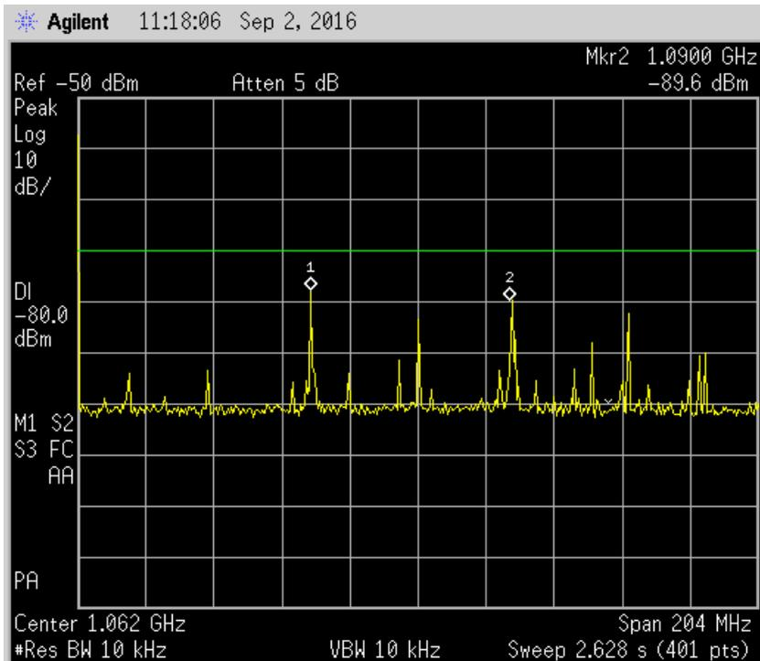
Figure 57: Spectrum scan of the DME band
