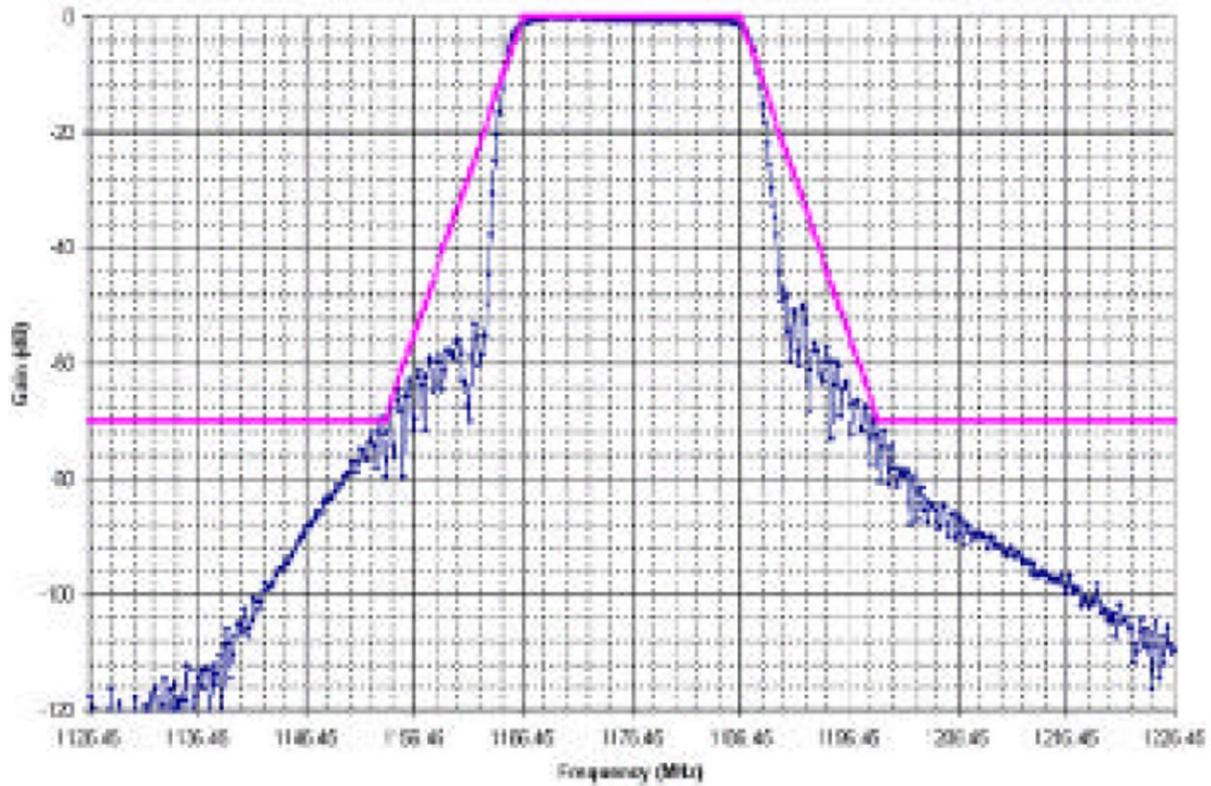
Figure 76: Characterisation of L5 Receiver Performance Using Digital Pulse Blanking [99]
