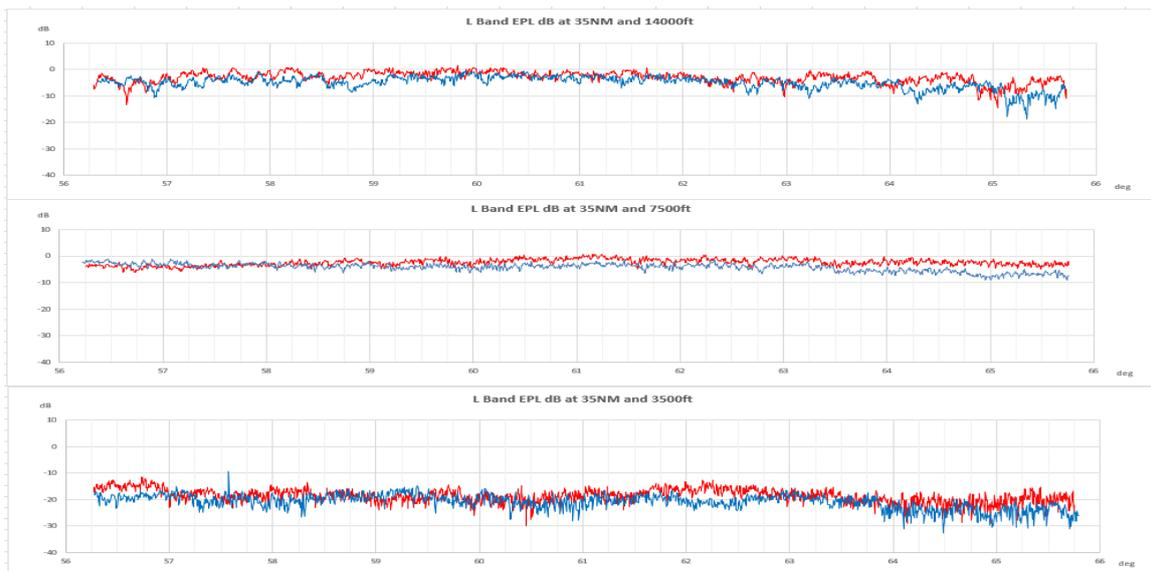
**Figure 11: Excess path loss (dB) test results at 35 NM distance with flight levels of 3500 feet, 7500 feet and 14000 feet**
