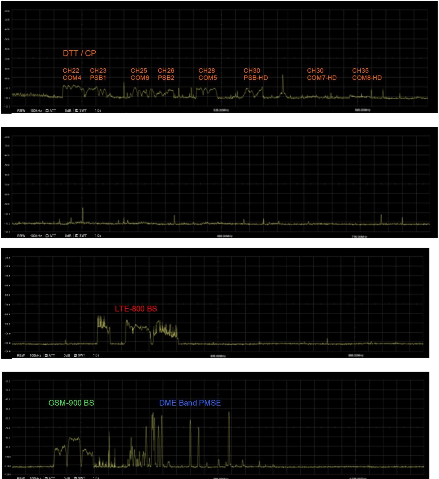
Figure 38: Spectrum scans for the TV, cellular and DME bands
