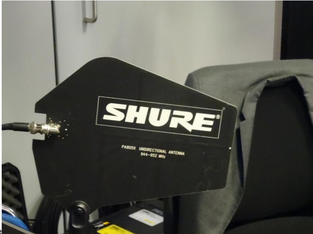
**Figure 12: Directional receive antenna**
