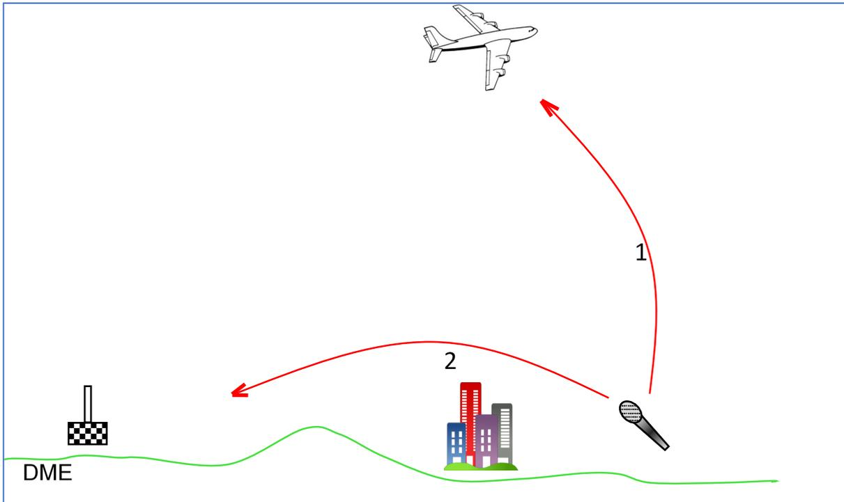
**Figure 77: Audio PMSE sharing radio spectrum with DME systems**
