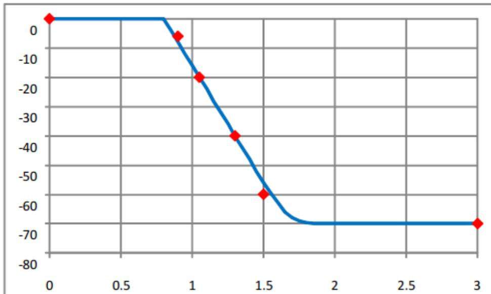
**Figure 78: Airborne selectivity of a 442 DME receiver (Bandwidth of 1.8 MHz at 3 dB)**
