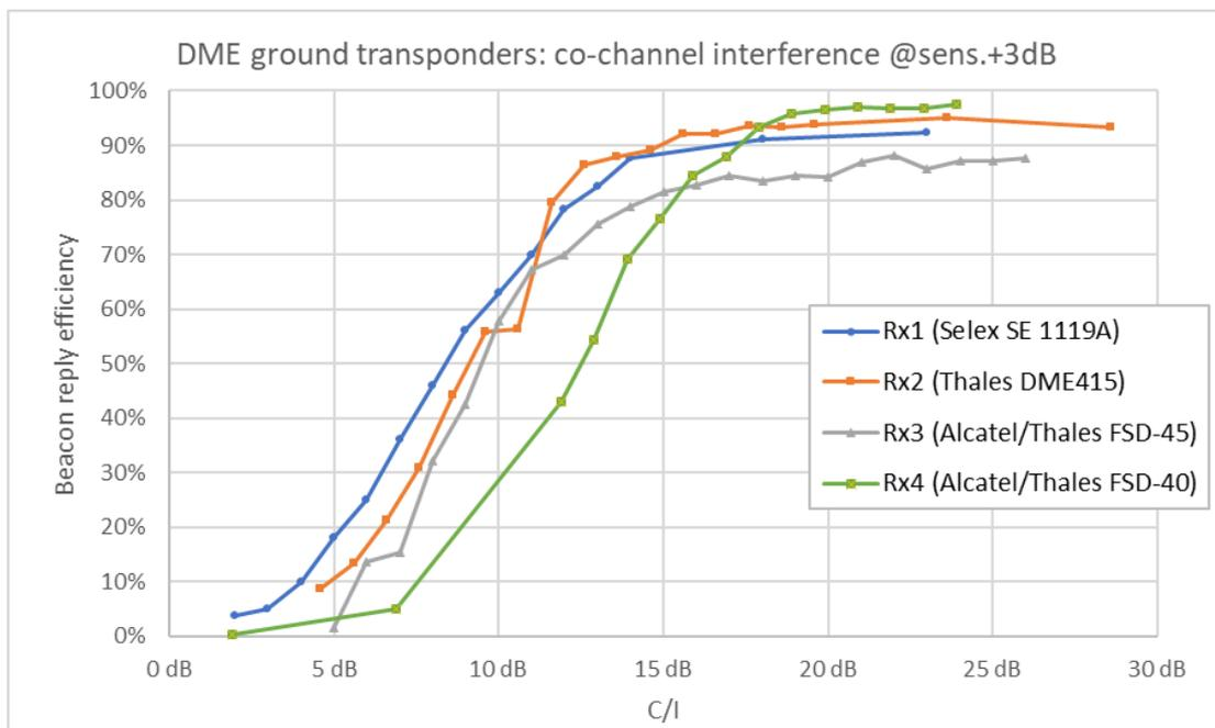
**Figure 128: BRE at different co-channel C/I**
