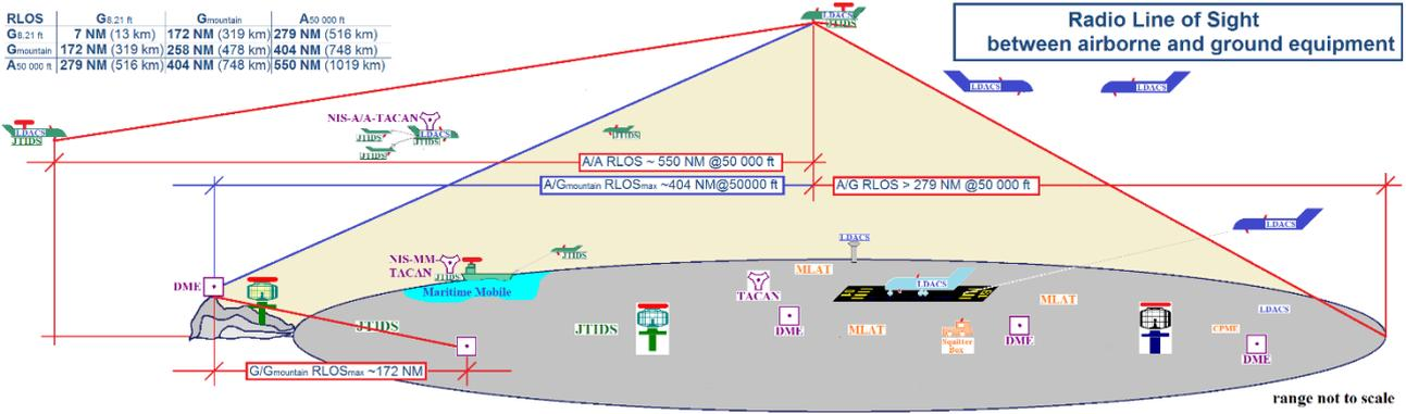
**Figure 9: Airborne and Ground RLOS of aeronautical equipment in operation [2]**
