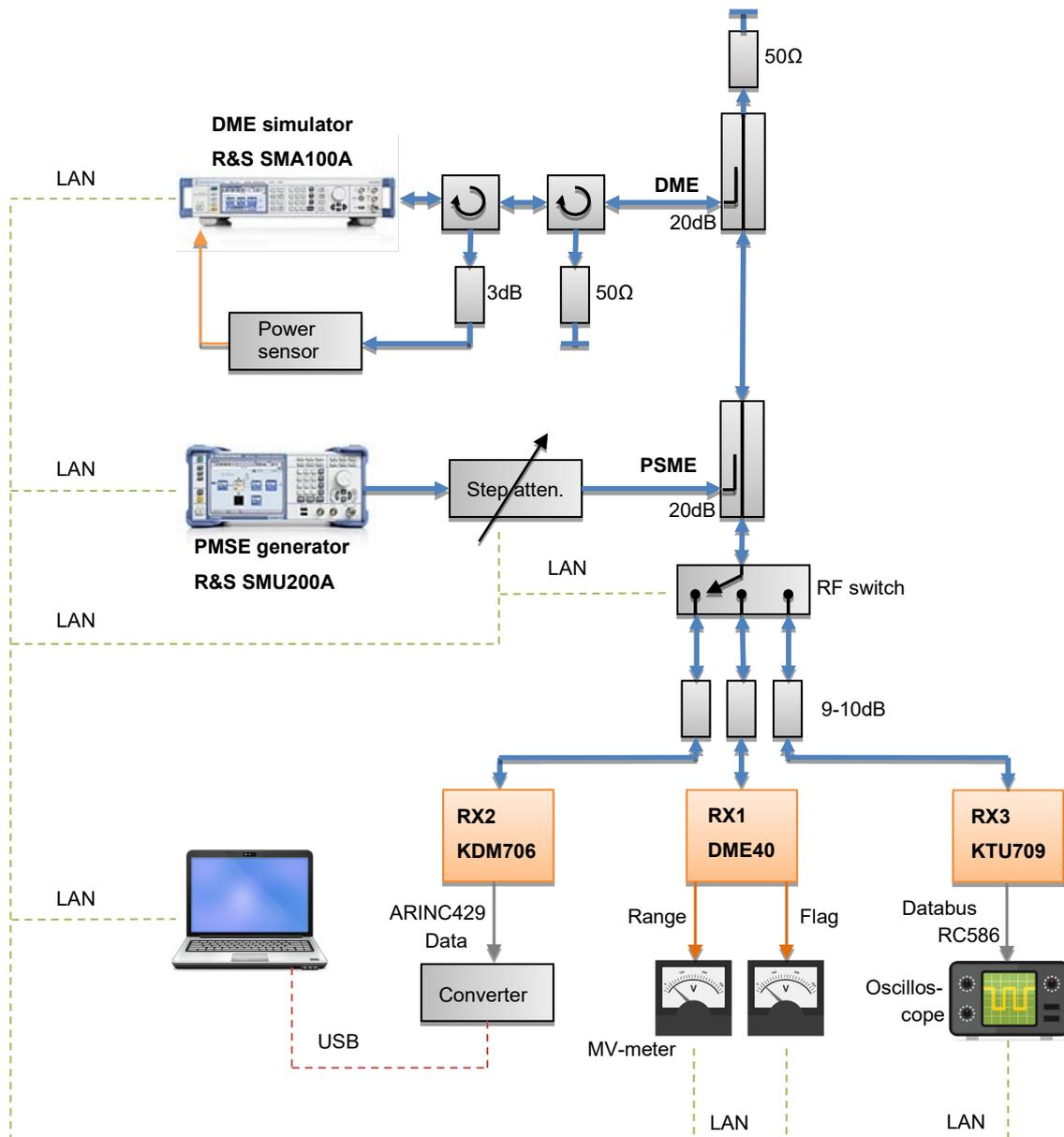
**Figure 115: Measurement setup for on-board interrogators as EUT**
