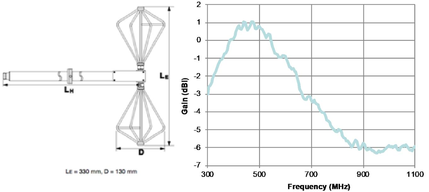
**Figure 50: Broadband bi-cone antenna and its gain used in the test**
