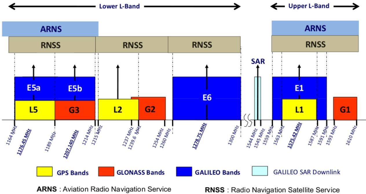
**Figure 99: RNSS Use of Frequency bands above 1164 MHz**
