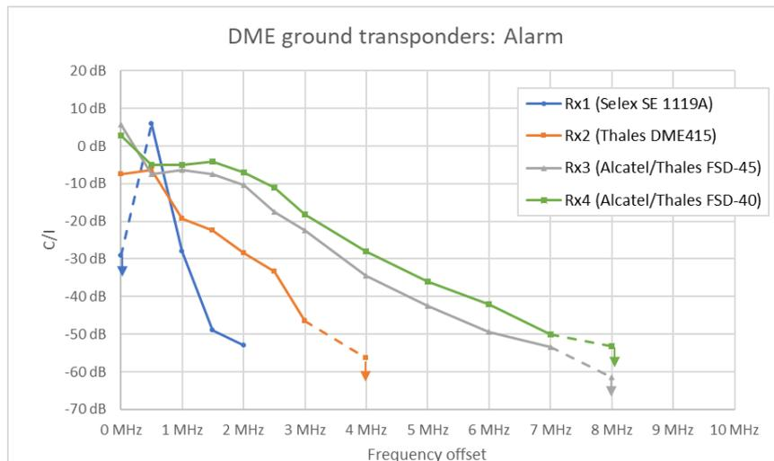
**Figure 130: Required C/I to ensure no alarm or warning is triggered**
