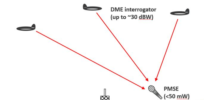
**Figure 3: Geometries for airborne interference into PMSE receivers**
