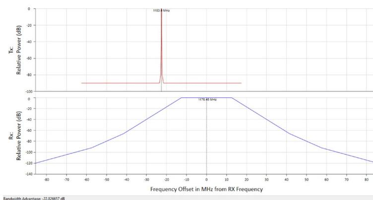
**Figure 73: GNSS receiver mask (Figure 9 of Report ITU-R M.2235)**
