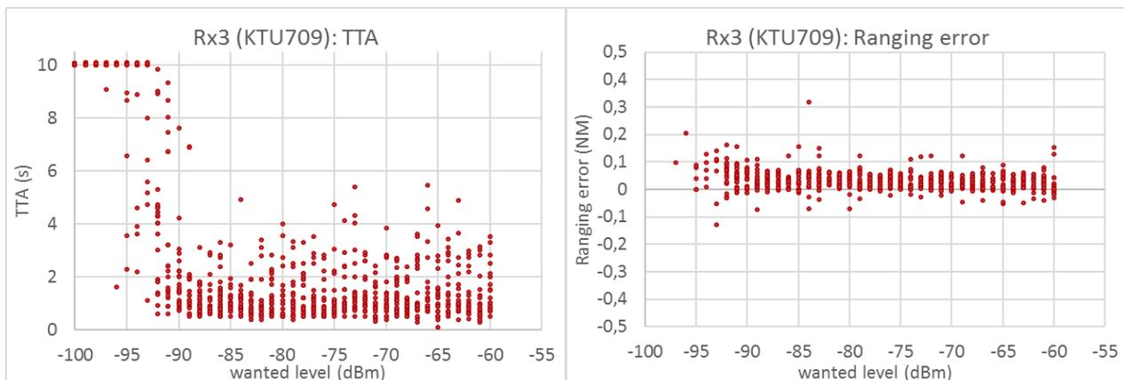
**Figure 118: TTA and ranging error for the non-distorted Rx3 (measurement timeout was 10 s)**
