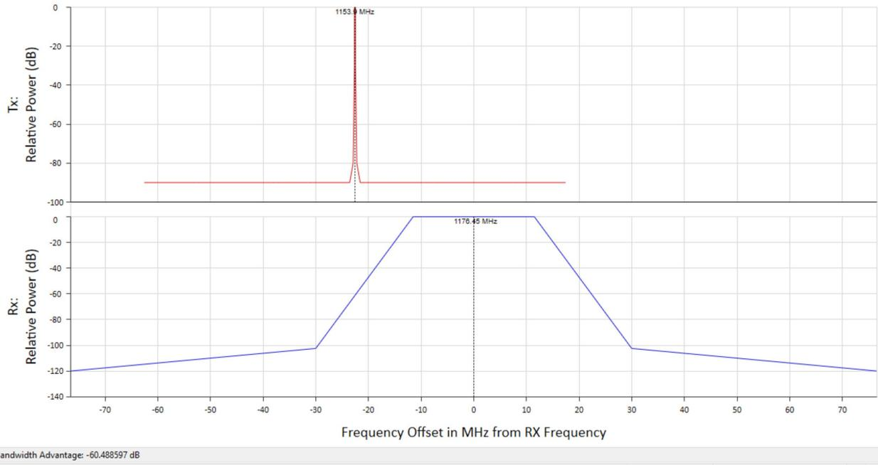
**Figure 74: GNSS receiver mask (Figure 8 of Report ITU-R M.2235)**
