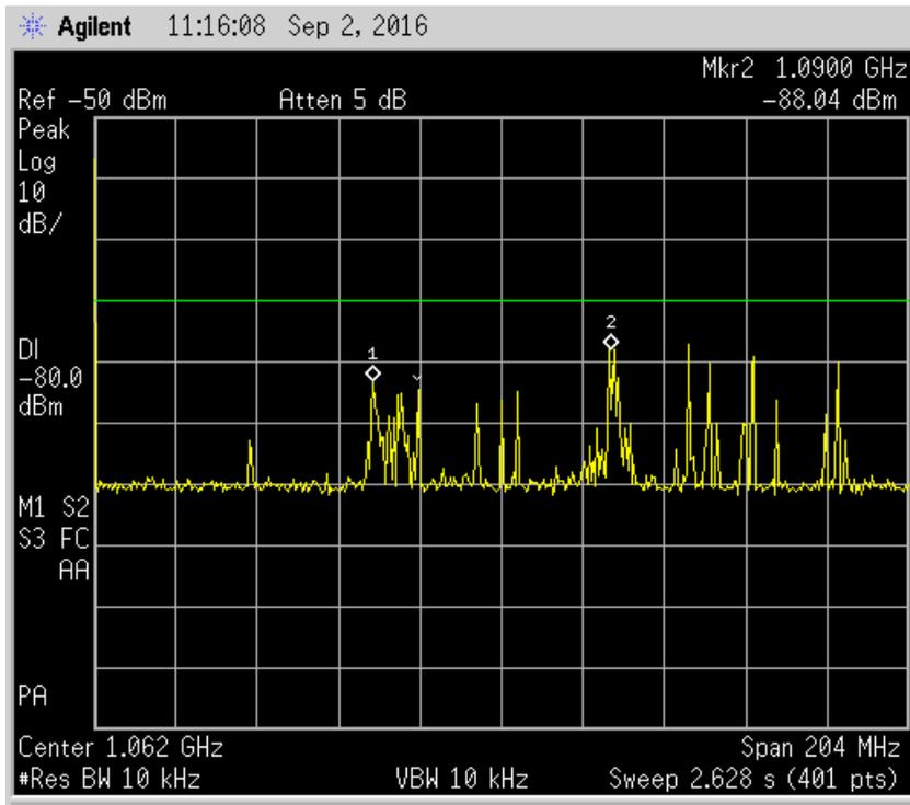
Figure 56: Spectrum scan of the DME band
