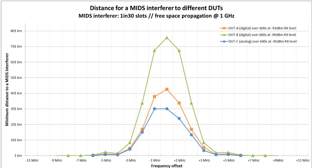
**Figure 96: Distance between a JTIDS/MIDS interferer and DUTs corresponding to the interferer levels the above figure**
