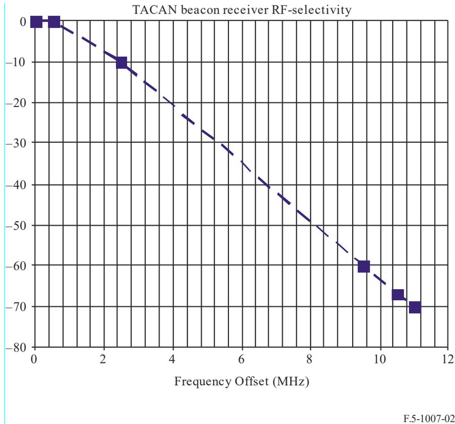
**Figure 70: Ground station (beacon) receiver RF selectivity curves**
