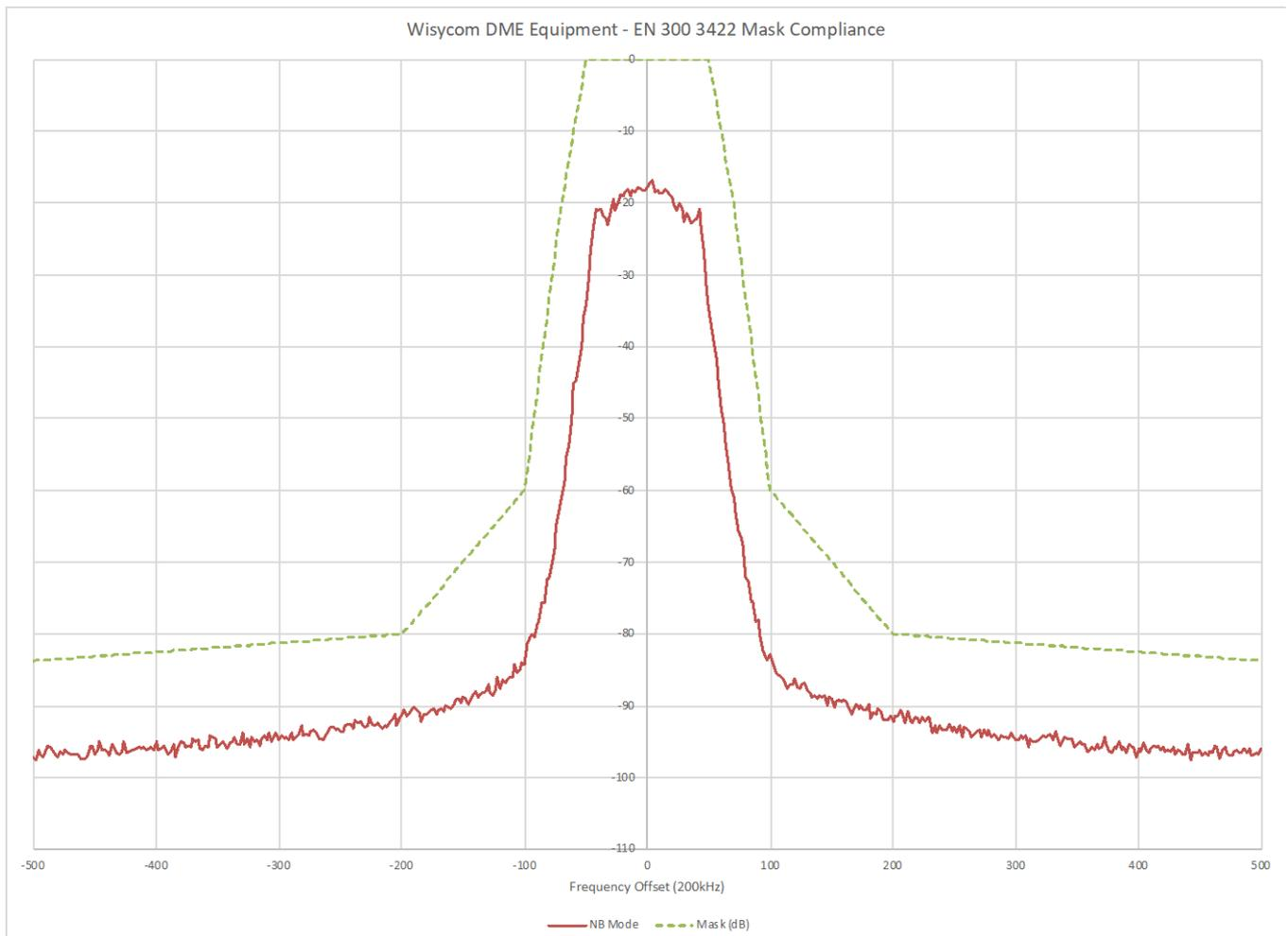
**Figure 62: Wisycom microphone transmitter mask (horizontal axis is in kHz) (in dB)**
