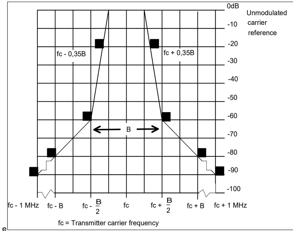
**Figure 65: Spectrum mask for analogue systems in all bands (measurement bandwidth is 1 kHz)**
