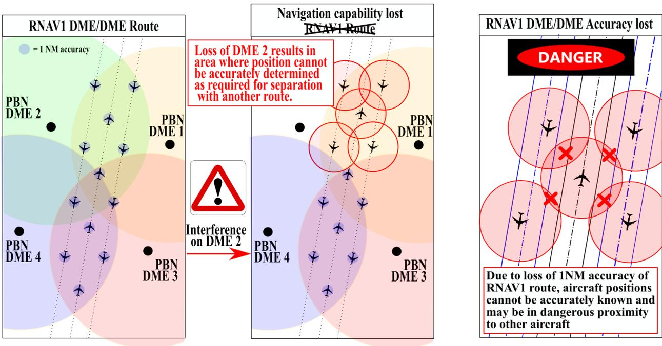
**Figure 1: Safety impact on DME in case of interference in 960-1164 MHz band**
