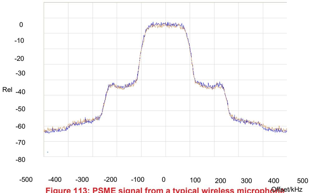
**Figure 113: PSME signal from a typical wireless microphone**
