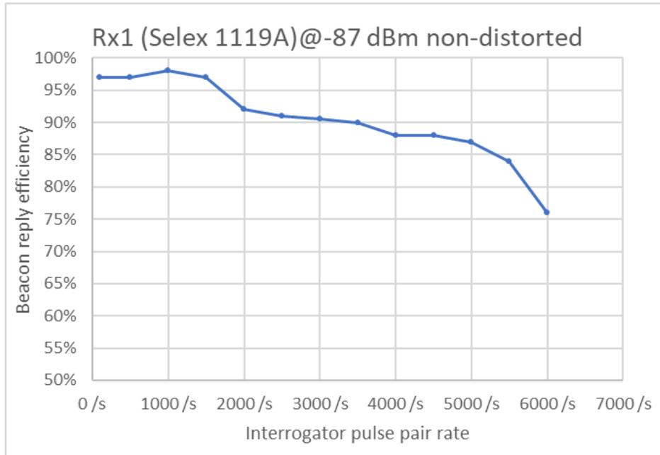
**Figure 127: Ground transponder performance depending on the number of interrogator pulse pairs per second**
