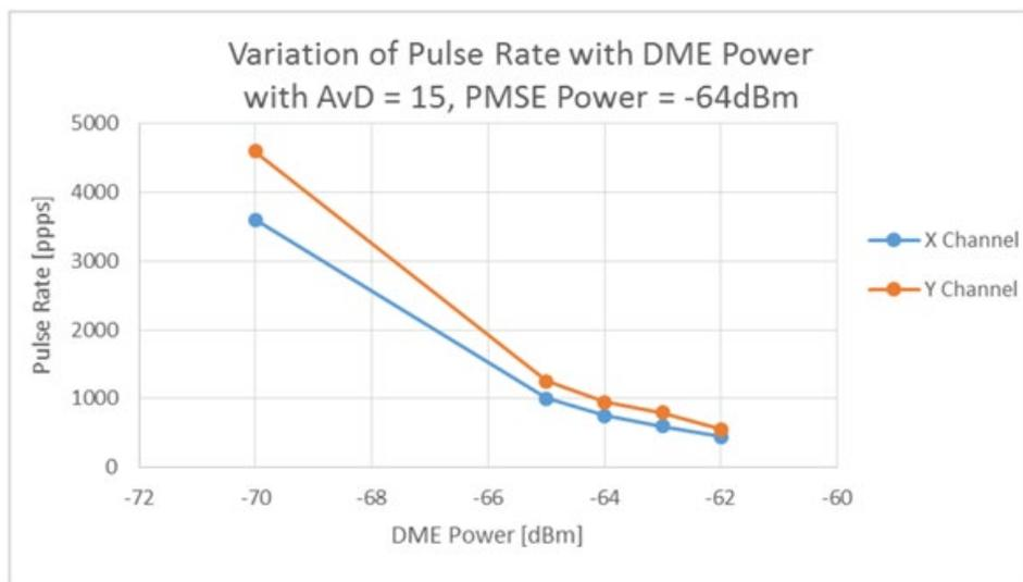
**Figure 67: Trade-off of DME Power and Pulse Rate into PMSE**
