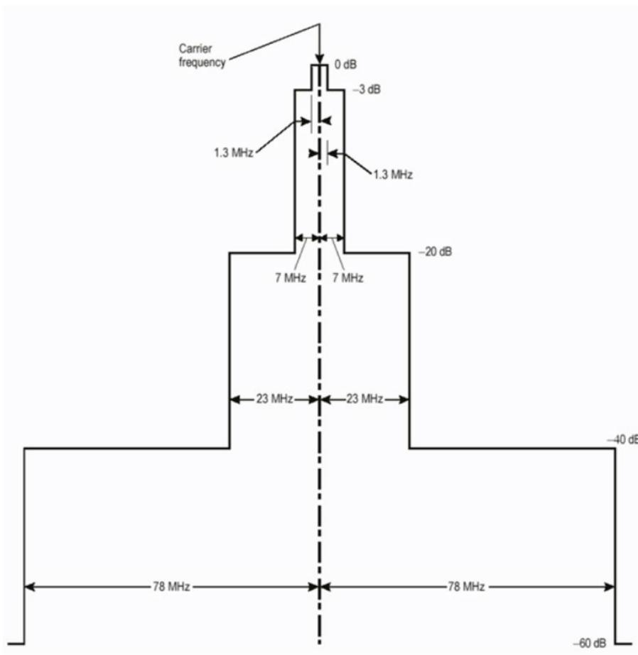
**Figure 71: Out-of-band emissions of SSR airborne transponder**
