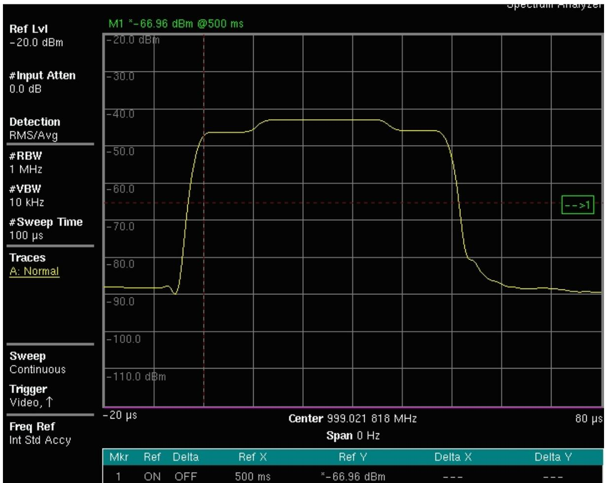
**Figure 30: DME ground station pulse shape measurement at the airport**
