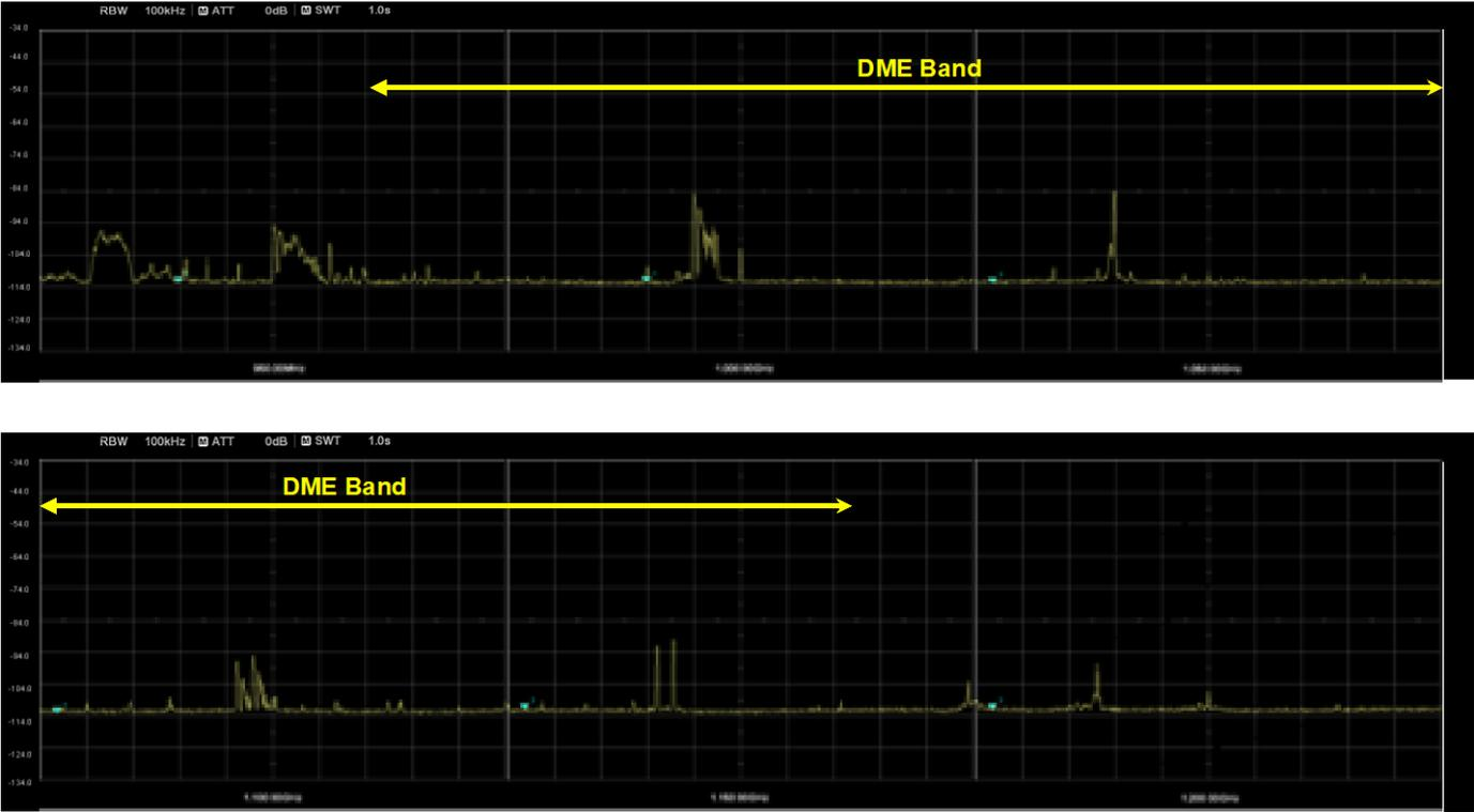
Figure 47: Spectrum scans of the DME band
