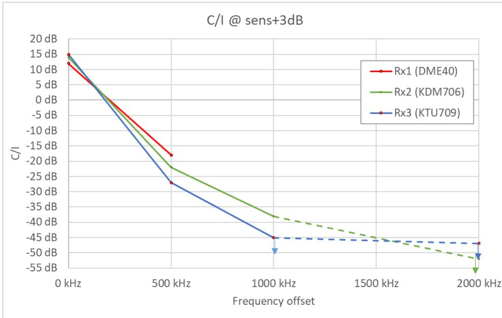
Figure 122: ASOP C/I for different offsets at wanted levels 3 dB above sensitivity
