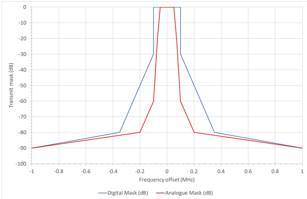
**Figure 98: PMSE Transmit Spectrum Masks The digital mask was used in this study**
