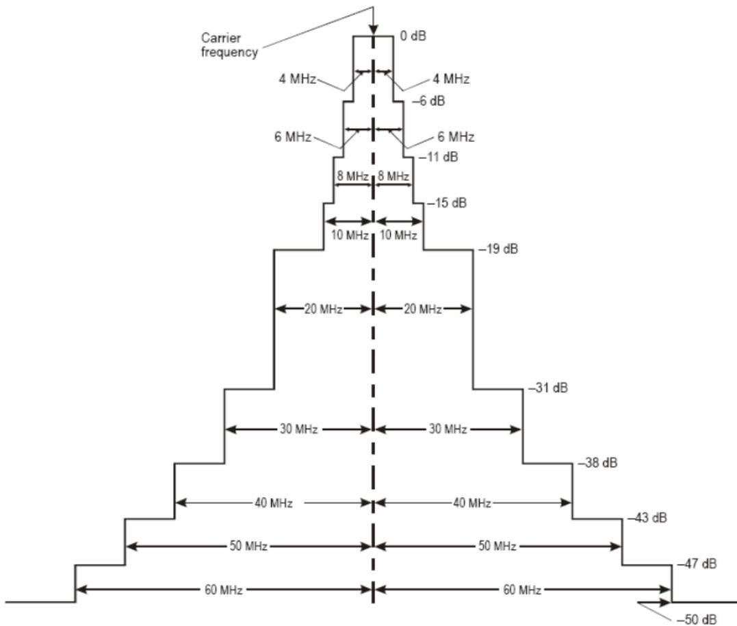
**Figure 72: Out-of-band emissions of SSR interrogator ground station**
