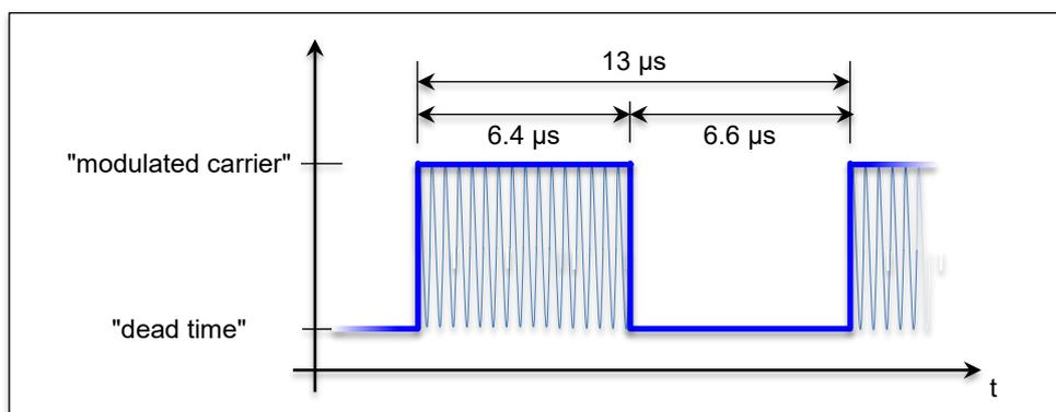
**Figure 81: JTIDS/MIDS pulse, basic characteristics**
