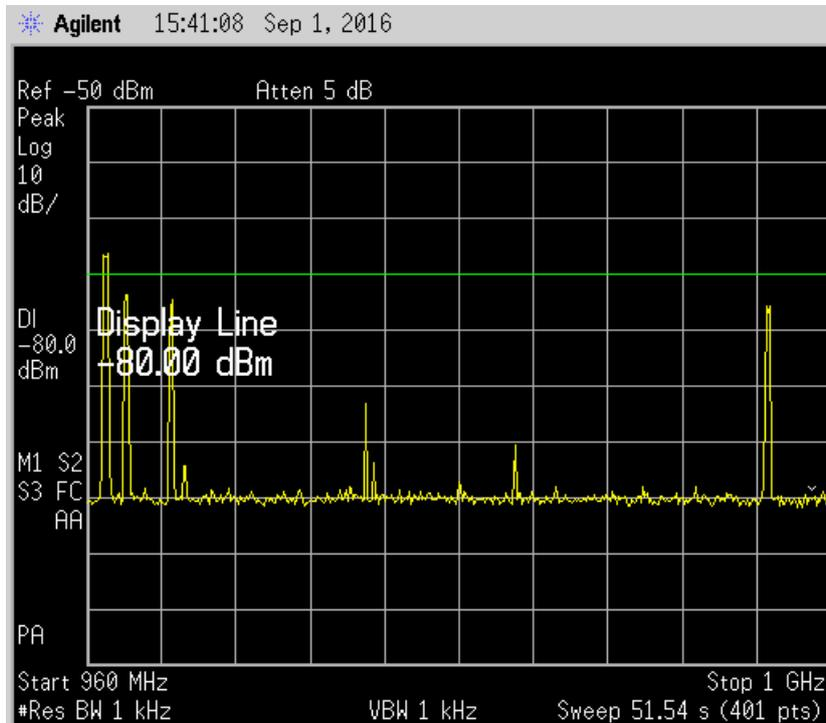
Figure 59: Spectrum scan of the DME band with microphones on
