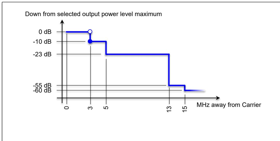
**Figure 82: JTIDS/MIDS pulse, power spectral mask requirement (in-band)**
