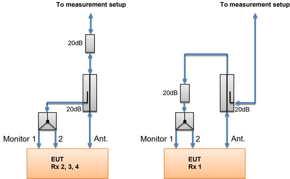
**Figure 125: Setup for the monitor function of the EUTs**
