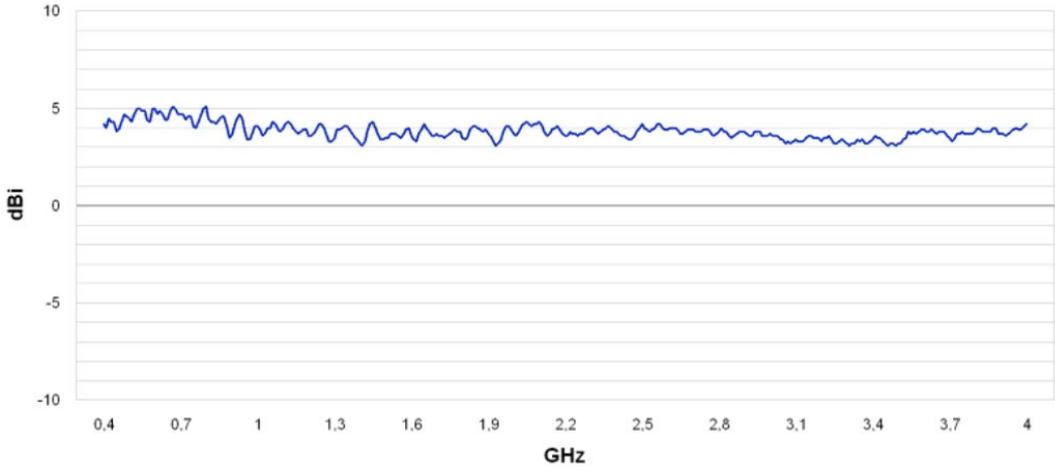
**Figure 29: Log periodic measurement antenna and gain over the measurement band**
