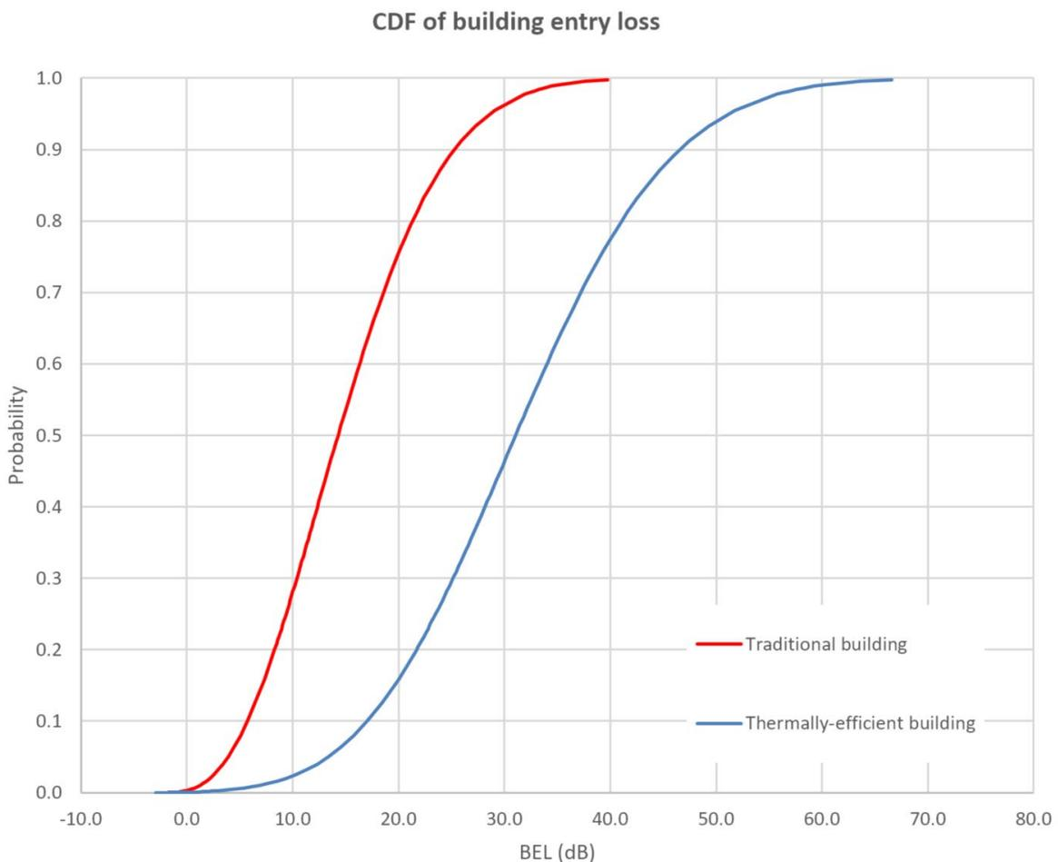
**Figure 69: Cumulative distribution function of building entry loss at 960 MHz**
