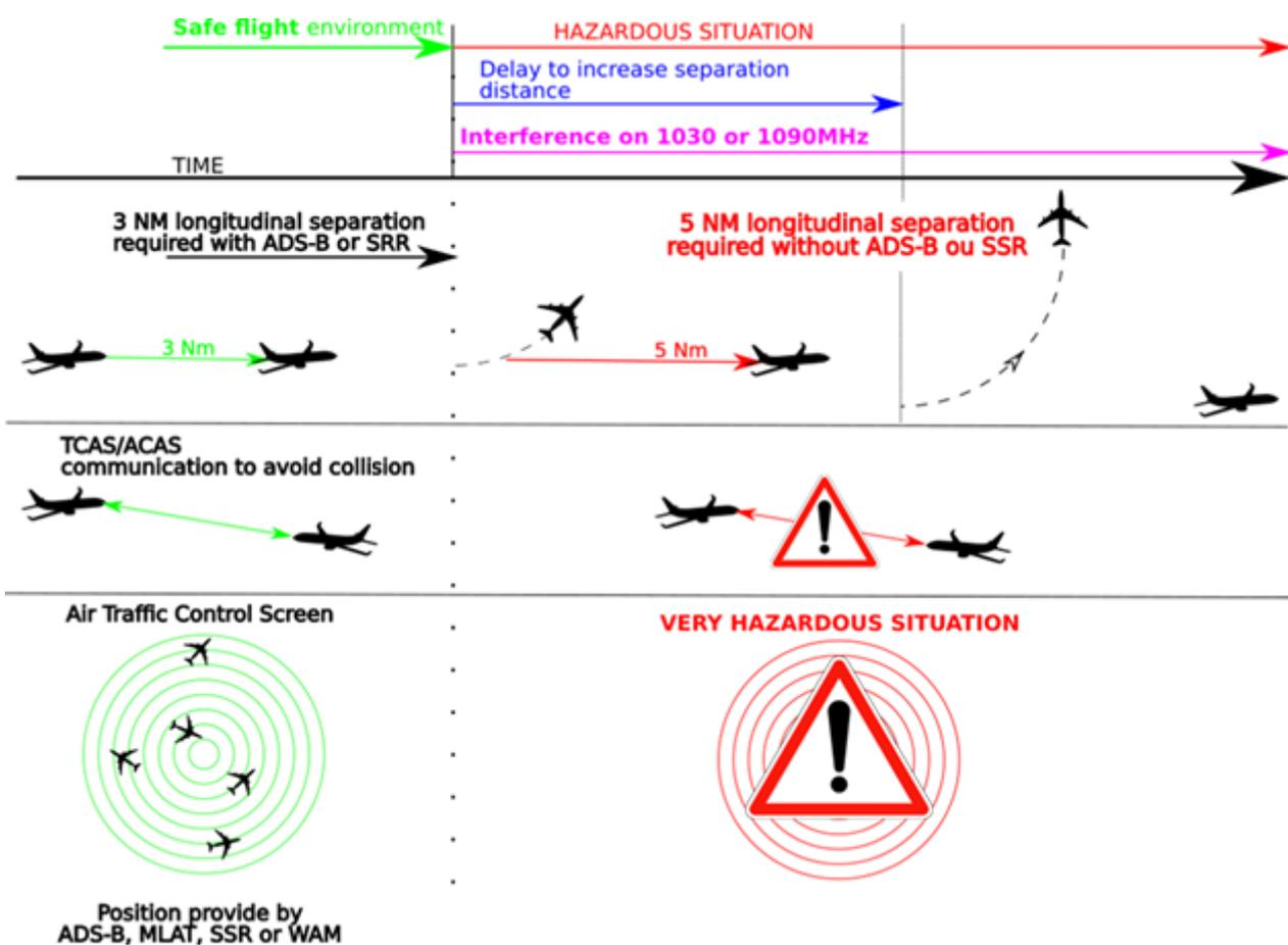
**Figure 2: Safety impact in case of interference to the frequencies 1030 MHz and 1090 MHz**
