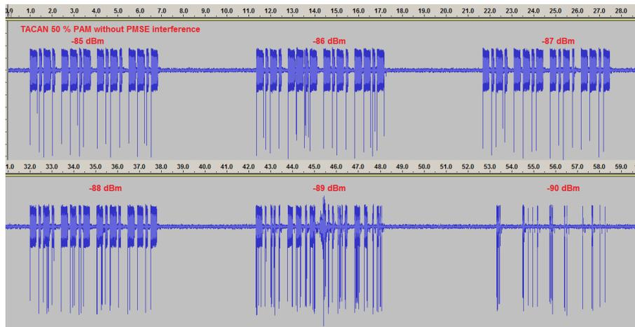
**Figure 133: KTU-709 TACAN identification without PMSE interference**
