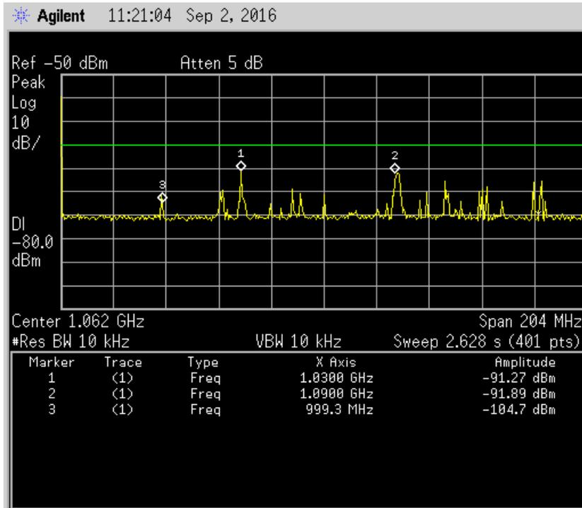
Figure 58: Spectrum scan of the DME band
