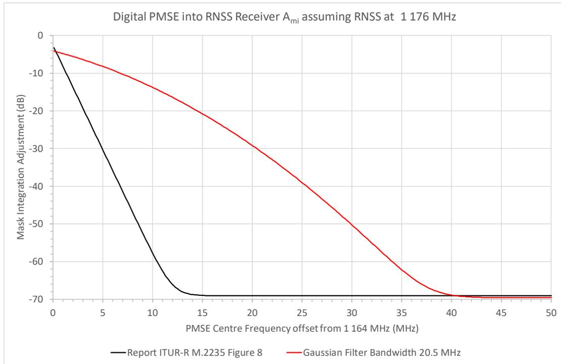
**Figure 80: Integration of PMSE Digital Mask with RNSS Receiver Mask**
