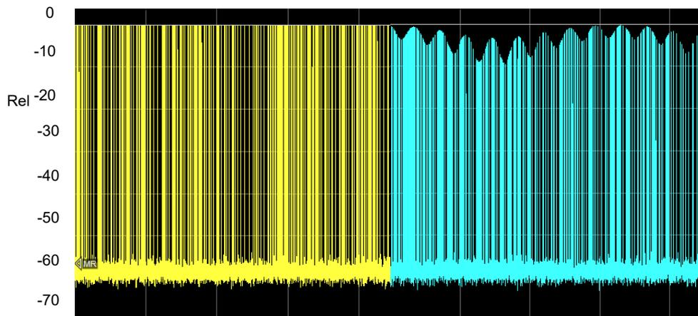
**Figure 112: DME (left) and TACAN with PAM (right) amplitude vs. time**
