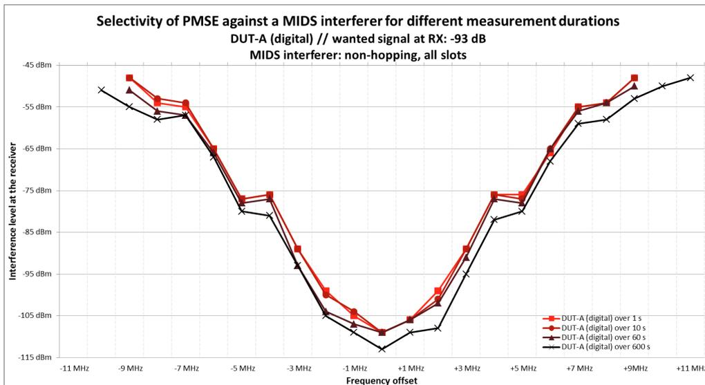
**Figure 91: Selectivity of PMSE depending on measurement duration**
