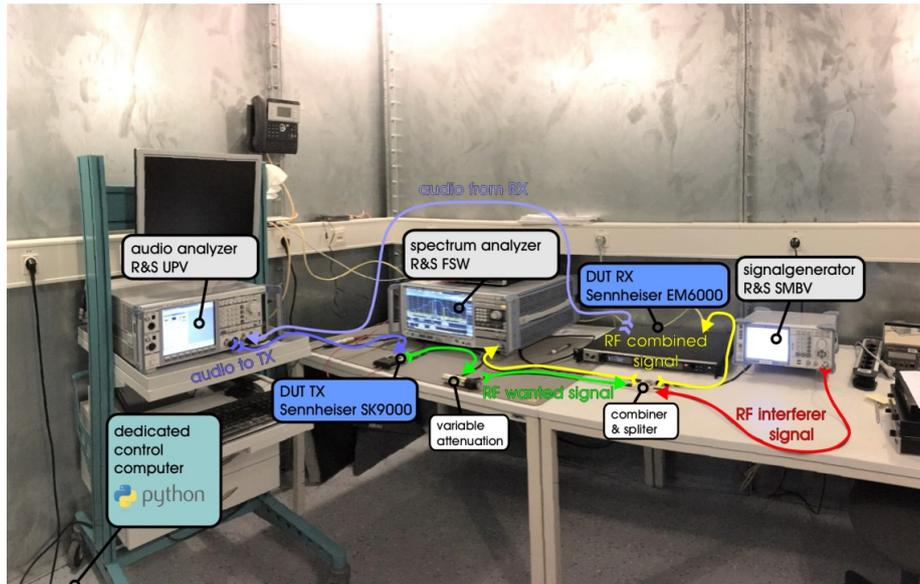
**Figure 85: Test chamber**
