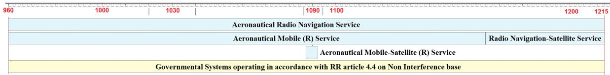
**Figure 7: Allocation of services and uses transmit centre frequencies in the band 960- 1215 MHz (2)**
