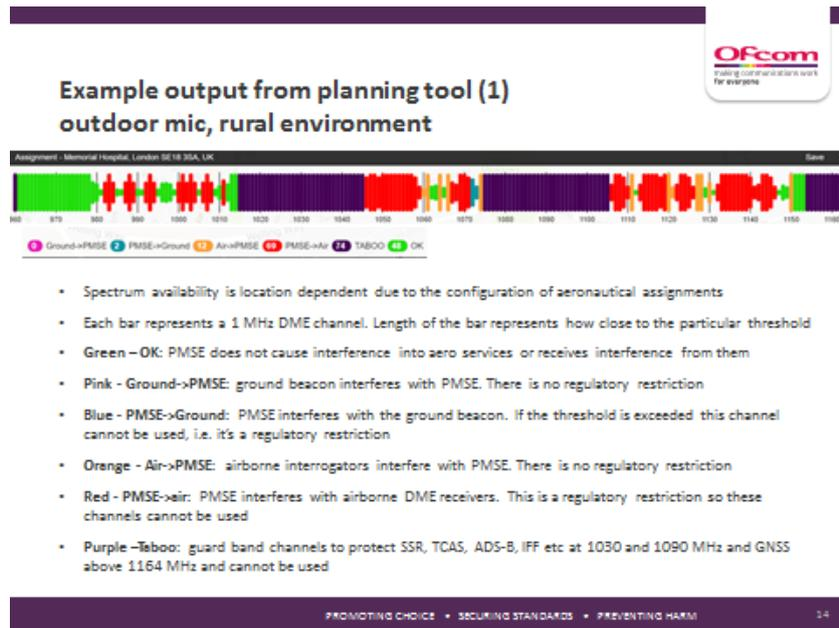
**Figure 6: Example output from planning tool (outdoor microphone, rural environment)**
