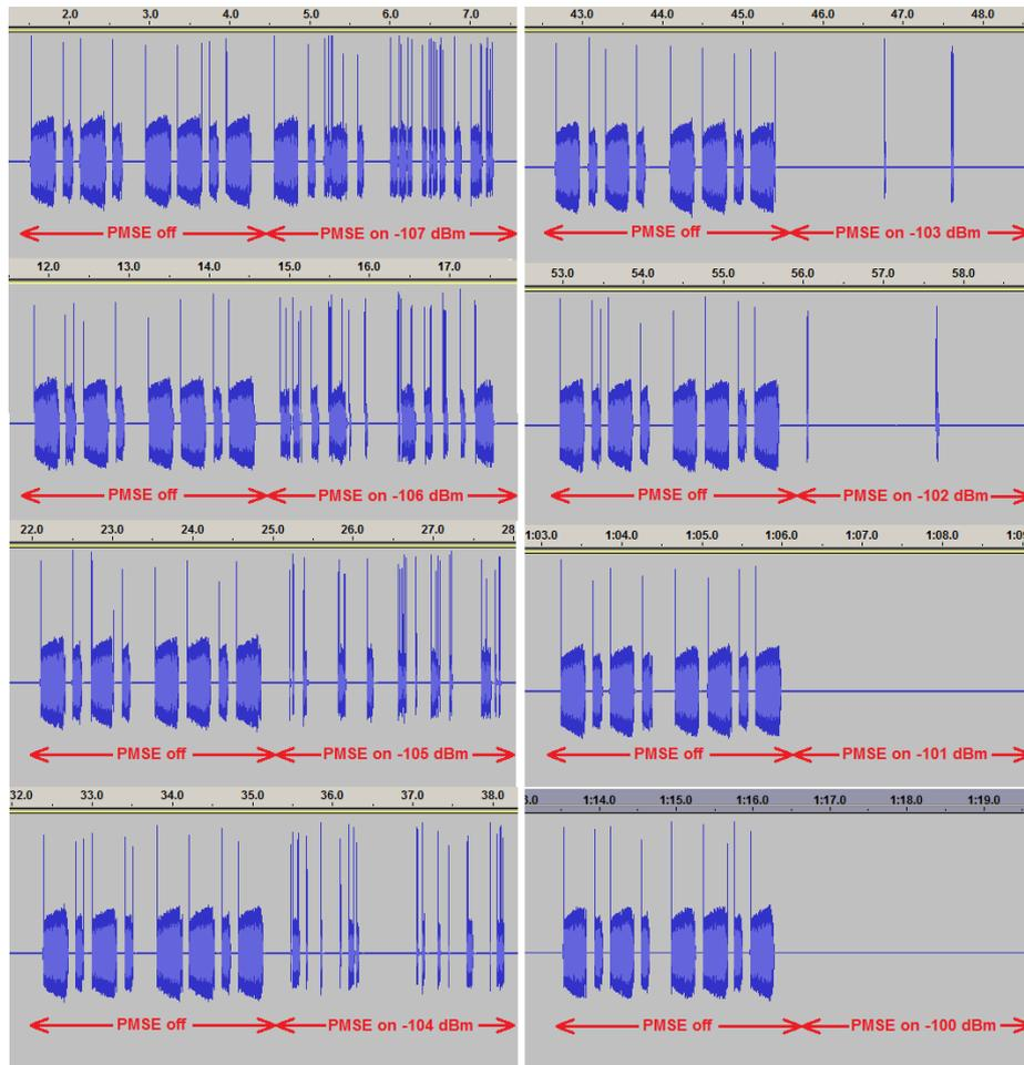
**Figure 134: KTU-709 PMSE on DME interference requiring a S/I of 20 dB**
