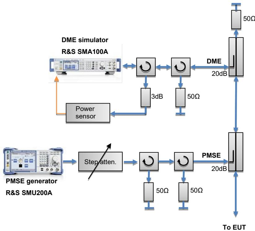
**Figure 124 Measurement setup for ground transponders as EUT**
