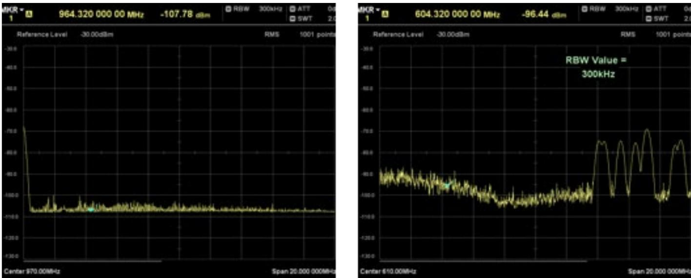
**Figure 46: Spectrum scans of the lower DME band and the UHF TV (PMSE) band**
