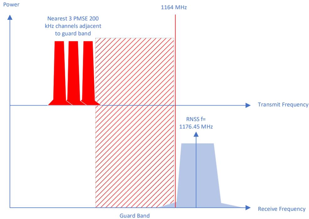
**Figure 103: PMSE Channels, guard band and RNSS receive frequency**
