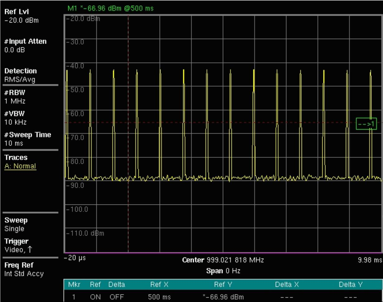
Figure 31: DME ground stations pulse spacing measurement at the airport
