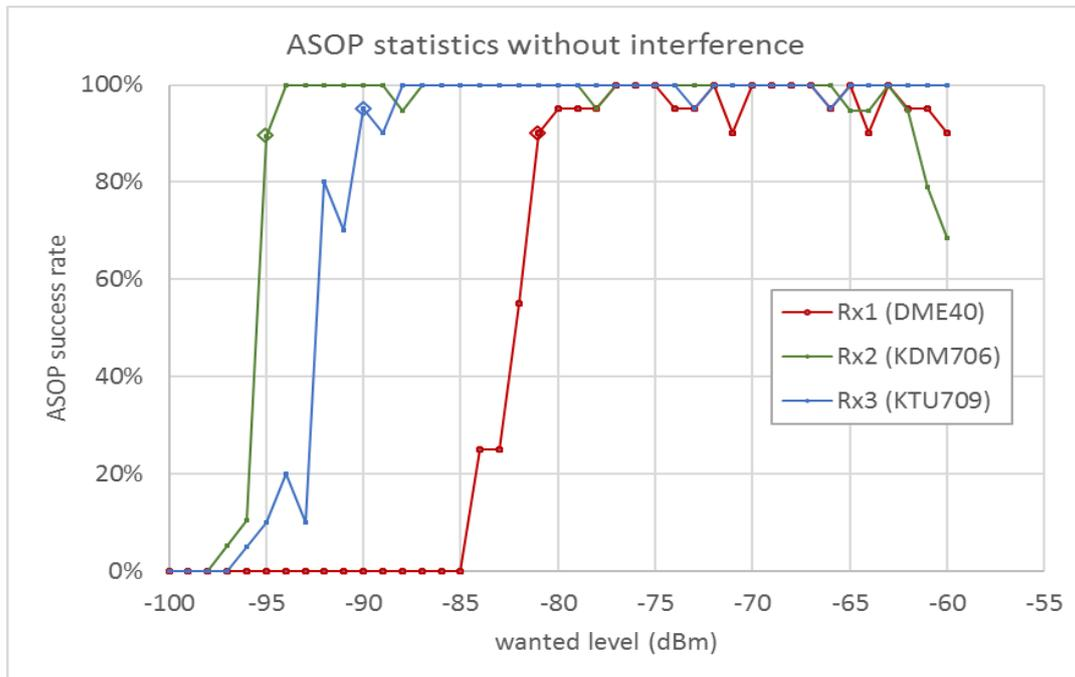
**Figure 119: Non-interfered ASOP statistics for selected failure criterion**
