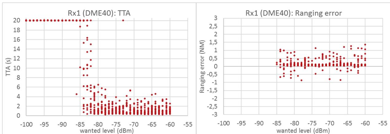
**Figure 116: TTA (Time To Acquire) and ranging error for the non-distorted Rx1 (measurement timeout was 20 s)**
