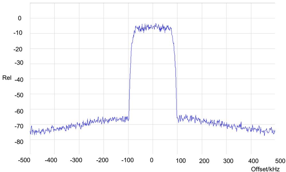
**Figure 114: Interfering PSME signal generated with SMU200A signal generator**
