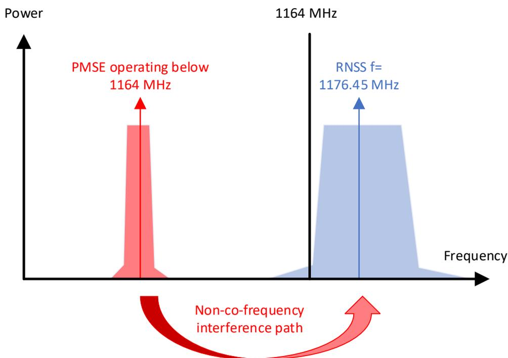
**Figure 97: PMSE in 960-1164 MHz Adjacent Band Sharing Scenario with RNSS operating above 1164 MHz**
