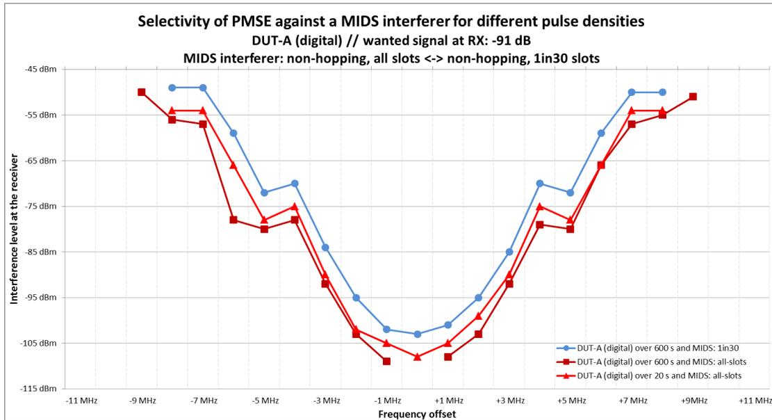
**Figure 92: Selectivity of the DUT-A (digital) depending on pulse density**
