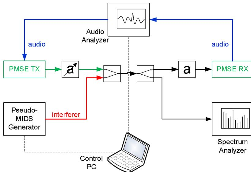
**Figure 84: Test setup block diagram**
