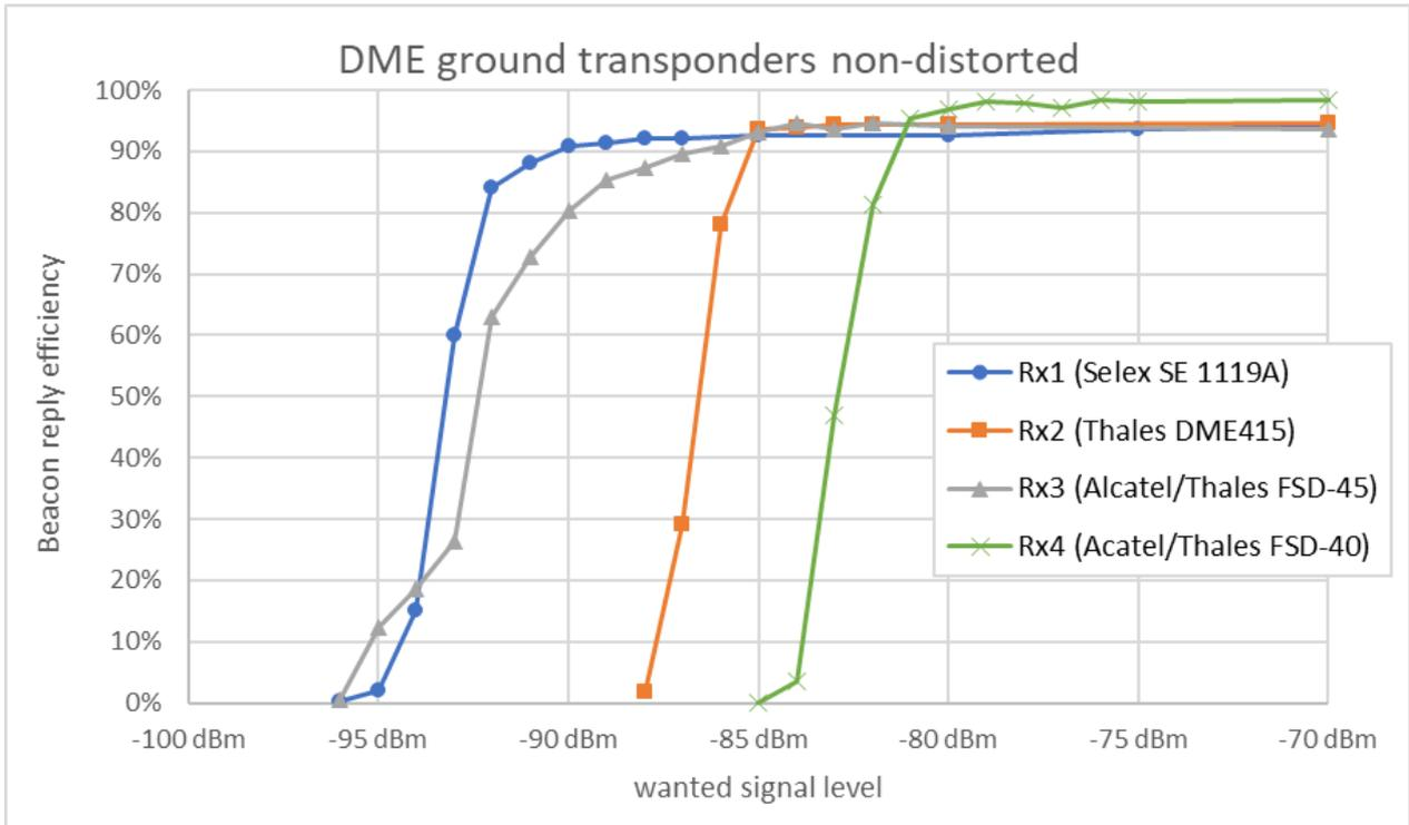
Figure 126: Beacon reply efficiency at low signal levels
