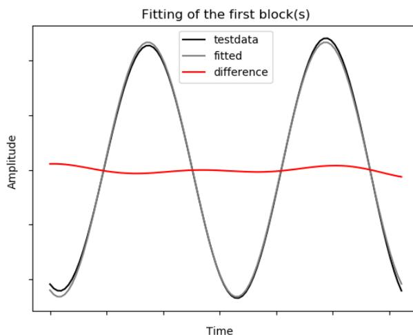
**Figure 83: Fitting of recorded sine tone**
