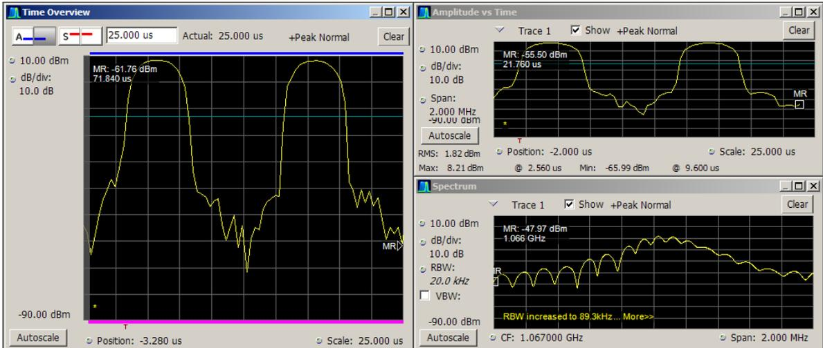
Figure 106: Measured pulse form KTU-709 (Bendix)
