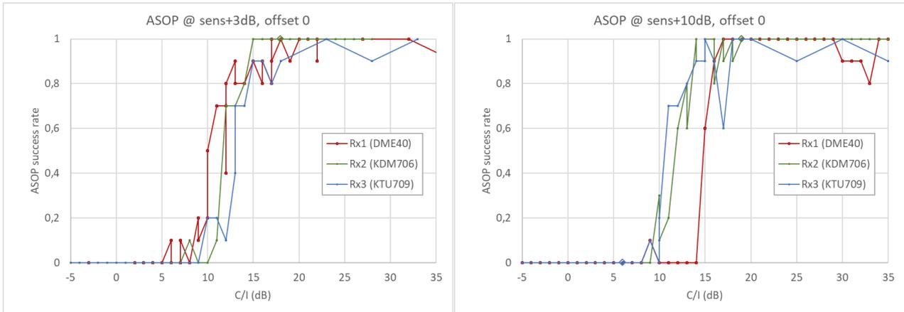
**Figure 120: ASOP success rate at different wanted signal levels when interfered by a co-channel PMSE signal**
