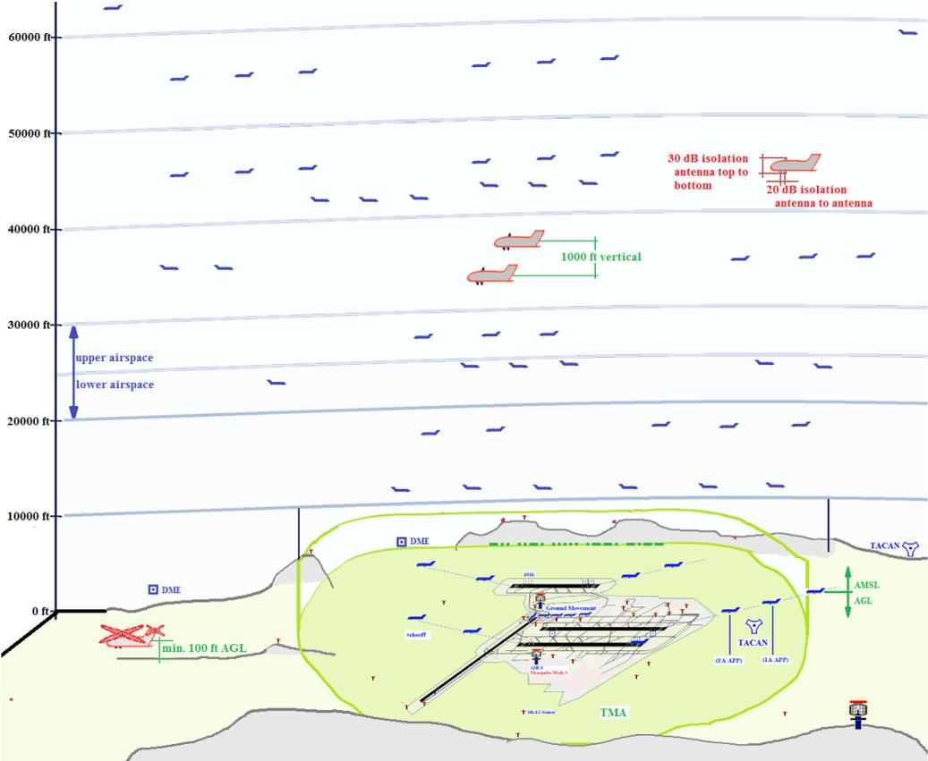
**Figure 10: Upper- and Lower airspace ATC operation, Flight Level and altitude for aircraft to be considered in the various phases of a flight [2]**
