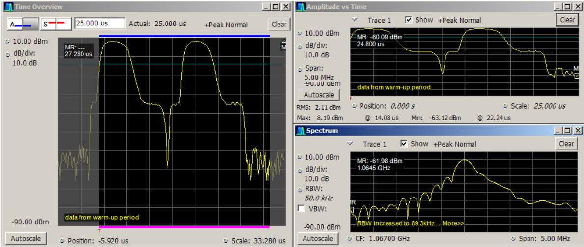
Figure 105: Measured pulse form DME-40 (Collins)
