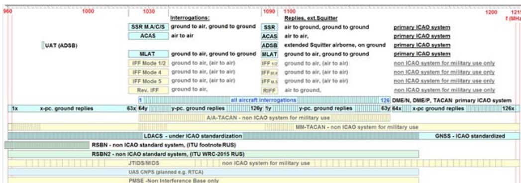
**Figure 8: Transmit centre frequencies in the band 960- 1215 MHz**
