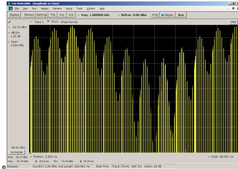
**Figure 131: Example of PAM during a morse code identification (SDX-2000).**
