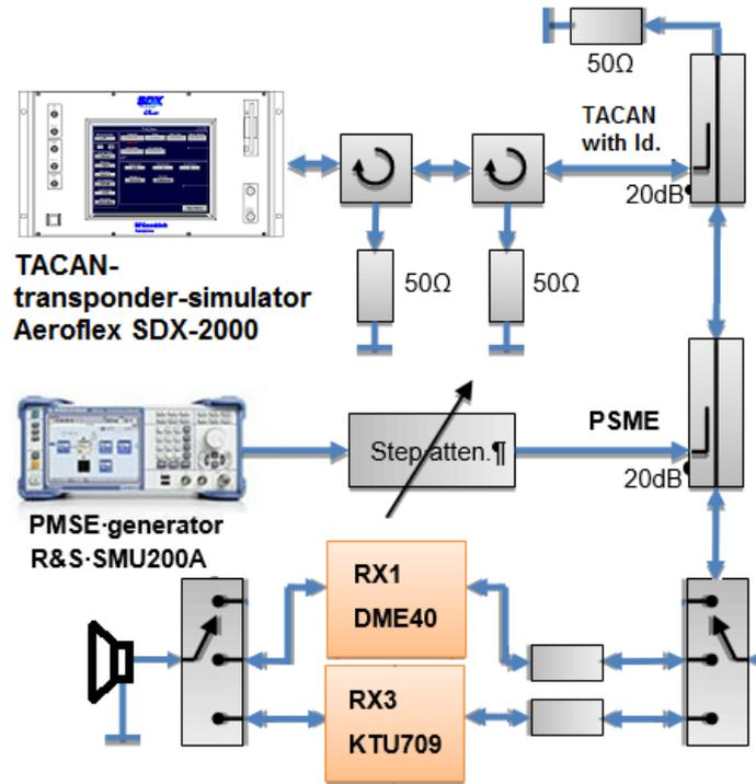
**Figure 132: Test setup for PMSE on TACAN-Identification tests**
