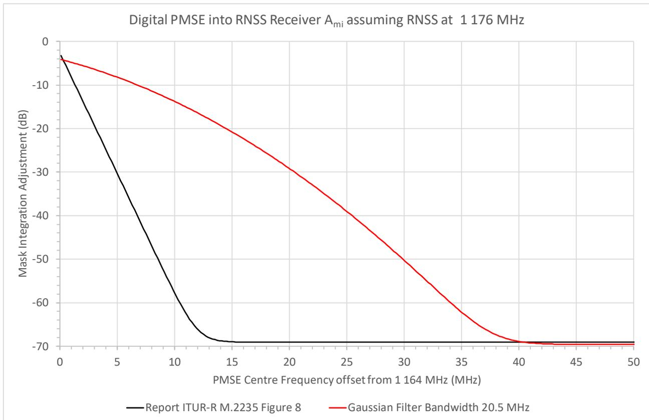
**Figure 102: Integration of PMSE Digital Mask with RNSS Receiver Masks**
