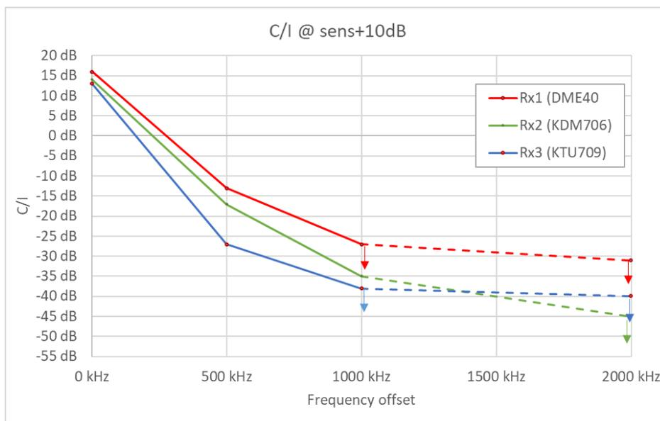
Figure 123: ASOP C/I for different offsets at wanted levels 10 dB above sensitivity
