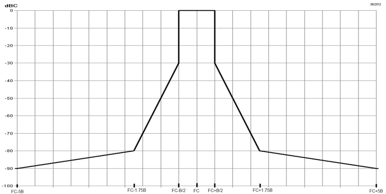
**Figure 66: Spectrum mask for digital systems below 2 GHz (measurement bandwidth is 1 kHz)**
