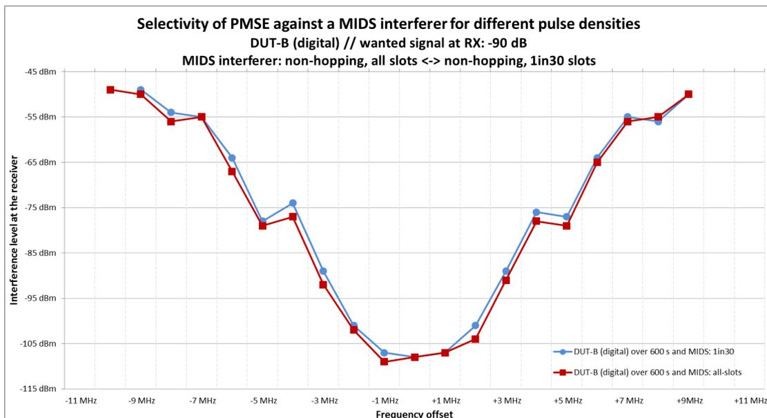
**Figure 93: Selectivity of the DUT-B (digital) depending on pulse density**
