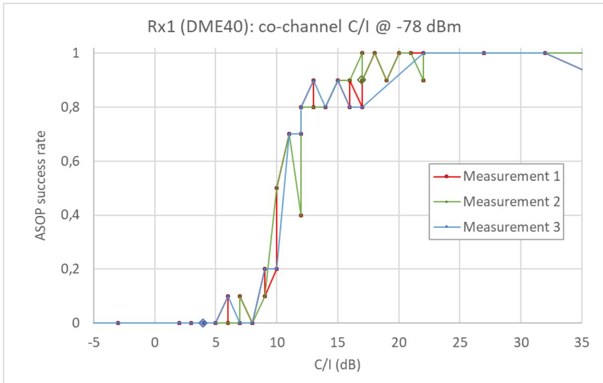
**Figure 121: Co-channel C/I for the DME40 interrogator at three different measurement days**
