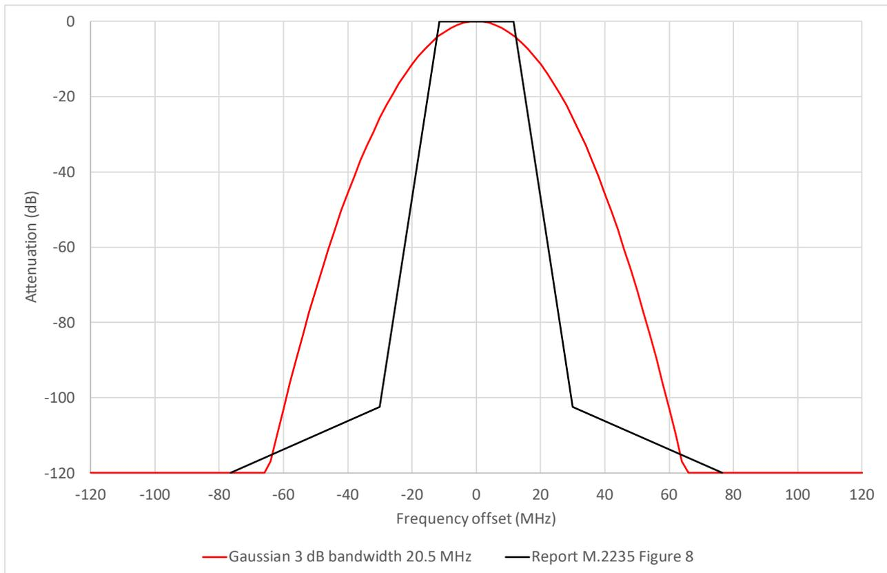
**Figure 100: RNSS Receive Filter Masks**
