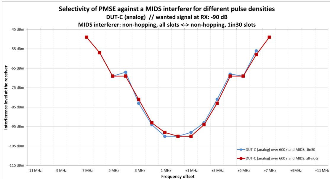
**Figure 94: Selectivity of the DUT-C (analog) depending on pulse density**
