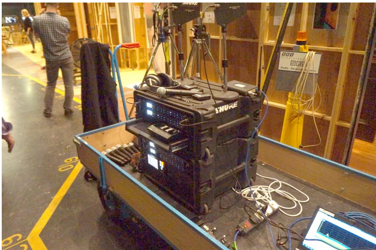
**Figure 37: Test receiver with two antennas for diversity reception**
