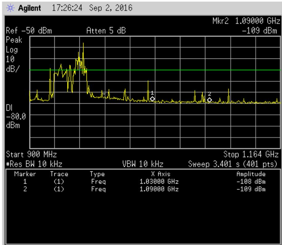
**Figure 60: Spectrum scan of the DME band measured inside window**
