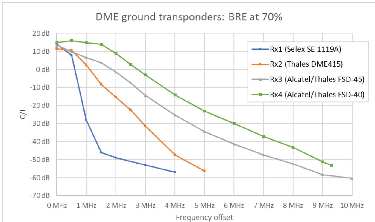
**Figure 129: C/I for a minimum beacon reply efficiency of 70%**
