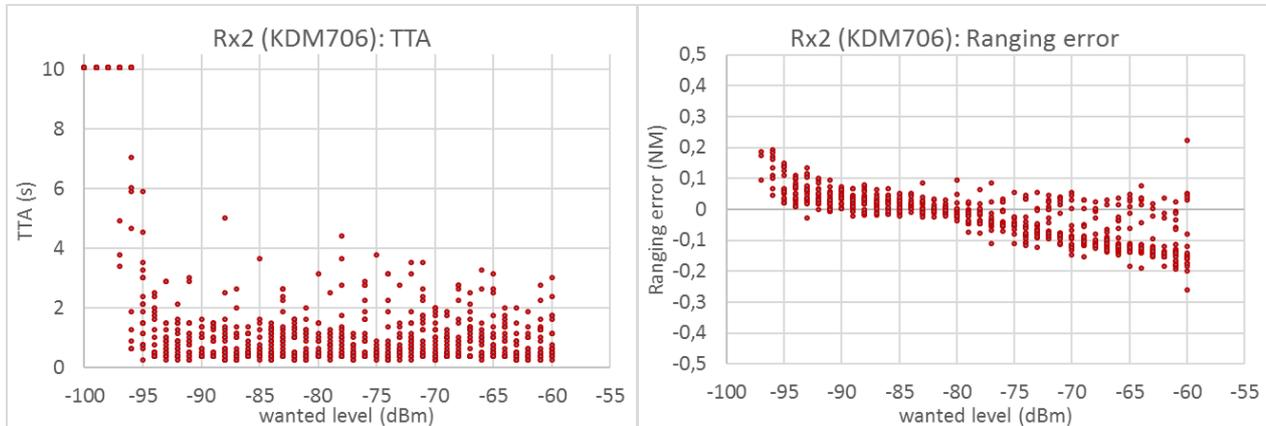
**Figure 117: TTA and ranging error for the non-distorted Rx2 (measurement timeout was 10 s)**
