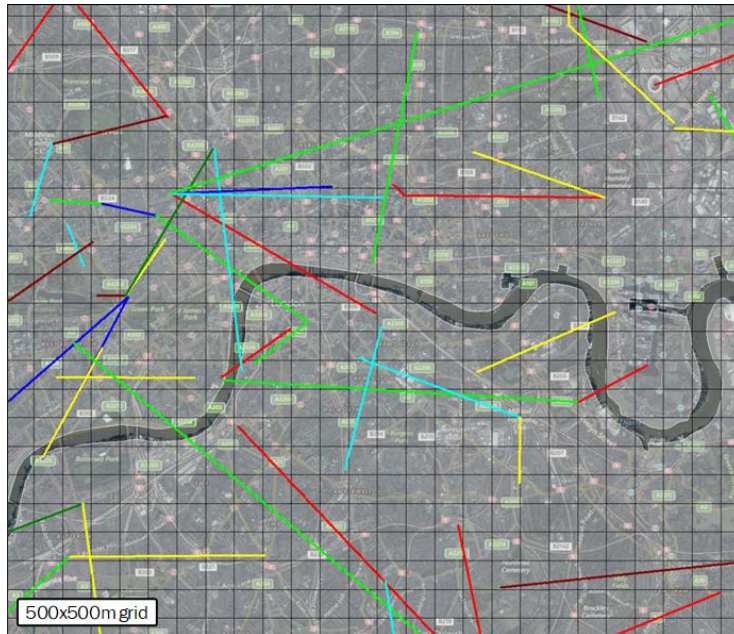
Figure 25: P-P links at 26 GHz in Central London [Source: Ofcom WTR, 2018, Bing Maps]
