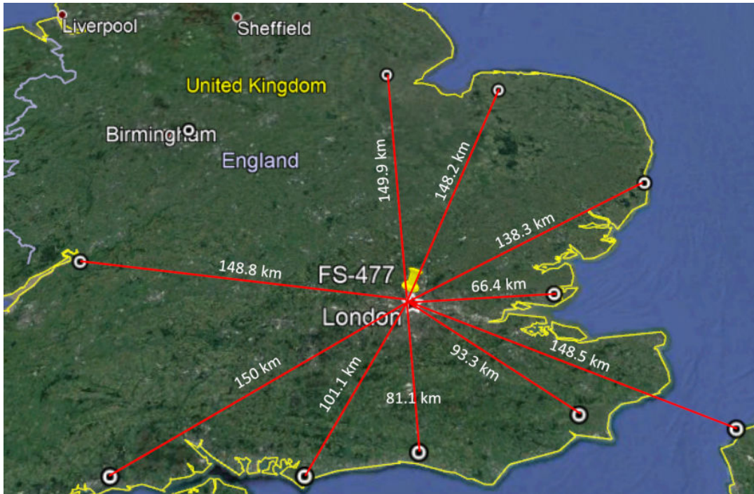
Figure 30: Geographic location of WAS/RLANs that overlap frequencies with UK FS 477 at the perimeter of 150 km radius
