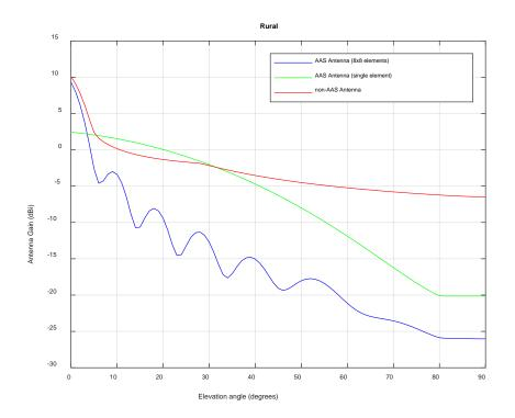
Figure 7: Antenna gains for different elevation angles above the horizon with a mechanical downtilt of 2.5 degrees for non-AAS and 10 degrees for AAS
