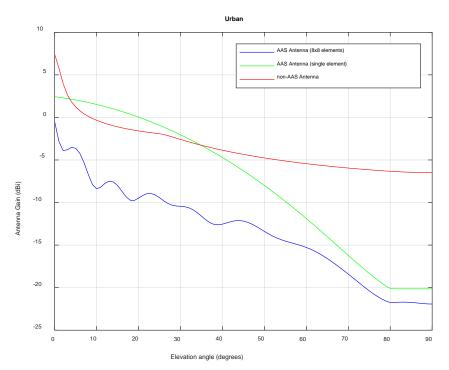
Figure 6: Antenna gains for different elevation angles above the horizon with a mechanical downtilt of 5 degrees for non-AAS and 10 degrees for AAS
