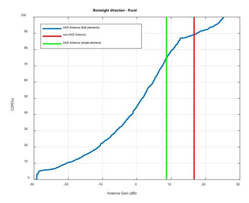
Figure 9: Comparison between antenna gain for AAS and non-AAS system in rural scenarios
