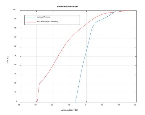
Figure 3: Comparison between antenna gain for AAS and non-AAS system below the horizon in urban scenarios (red curve - AAS antenna 8x8 elements and blue curve – single non-AAS antenna)
