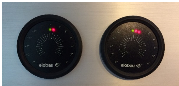
b) Mast auto levelling system control
