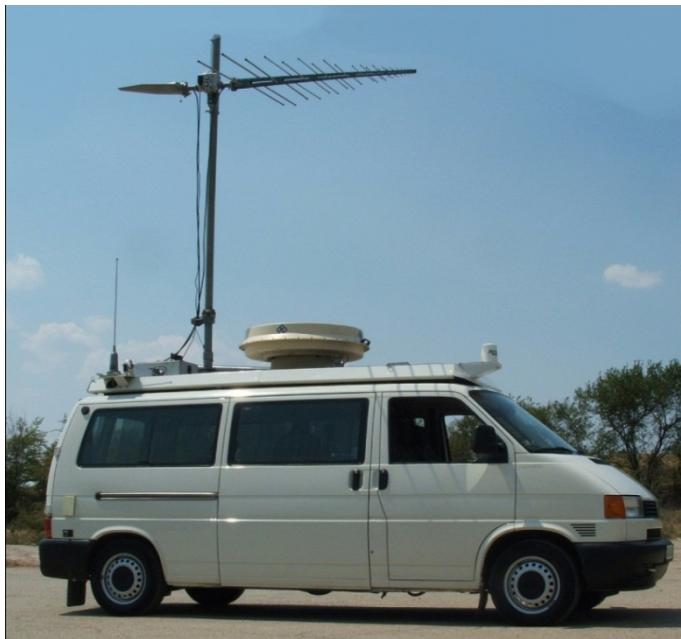
Figure 12: Inboard antenna mast with two directive antennas
