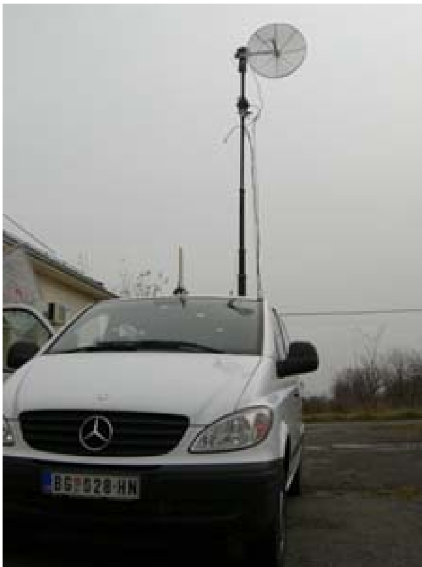
Figure 7: Special antennas for monitoring the wireless broadband IEEE 802.11 transmitters (Serbia)
