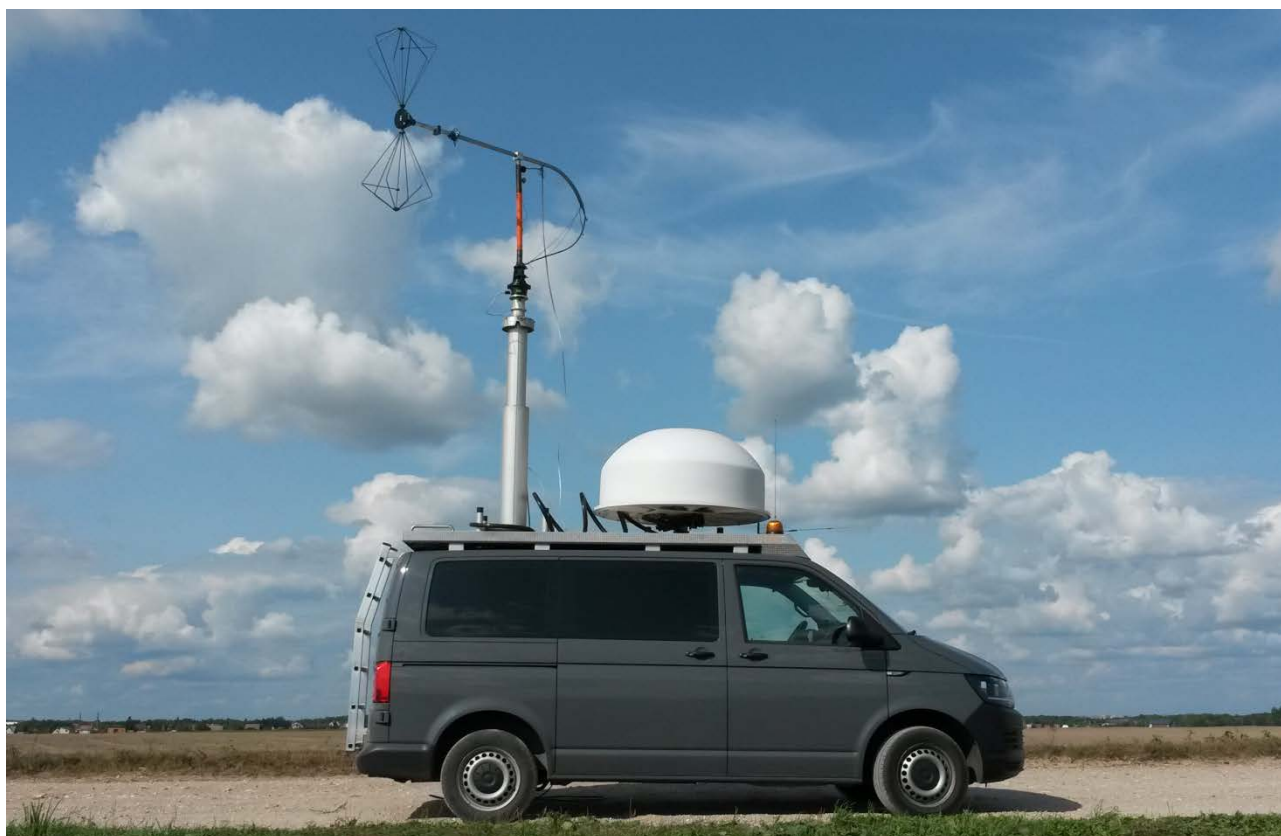
Figure 19: Universal setup: DF/monitoring/measurement antenna on a mast with a possibility to replace with any other measurement antenna (Lithuania)
