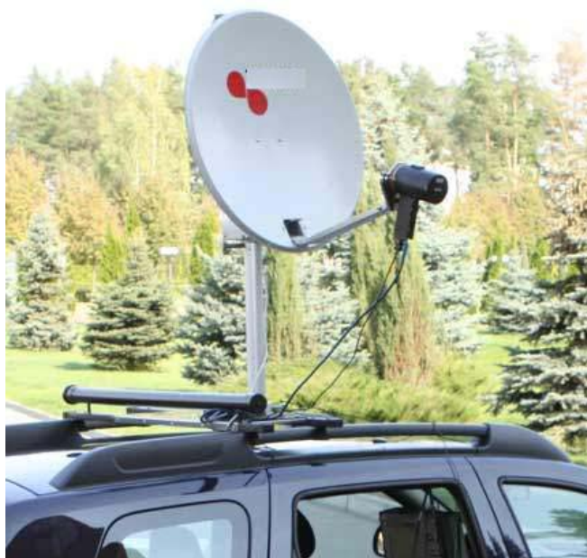
Figure 8: Measuring antenna, mounted on arm support on the roof of the vehicle
