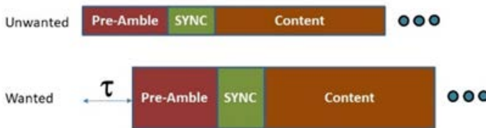
Figure 11: Harmful interference through false synchronisation
