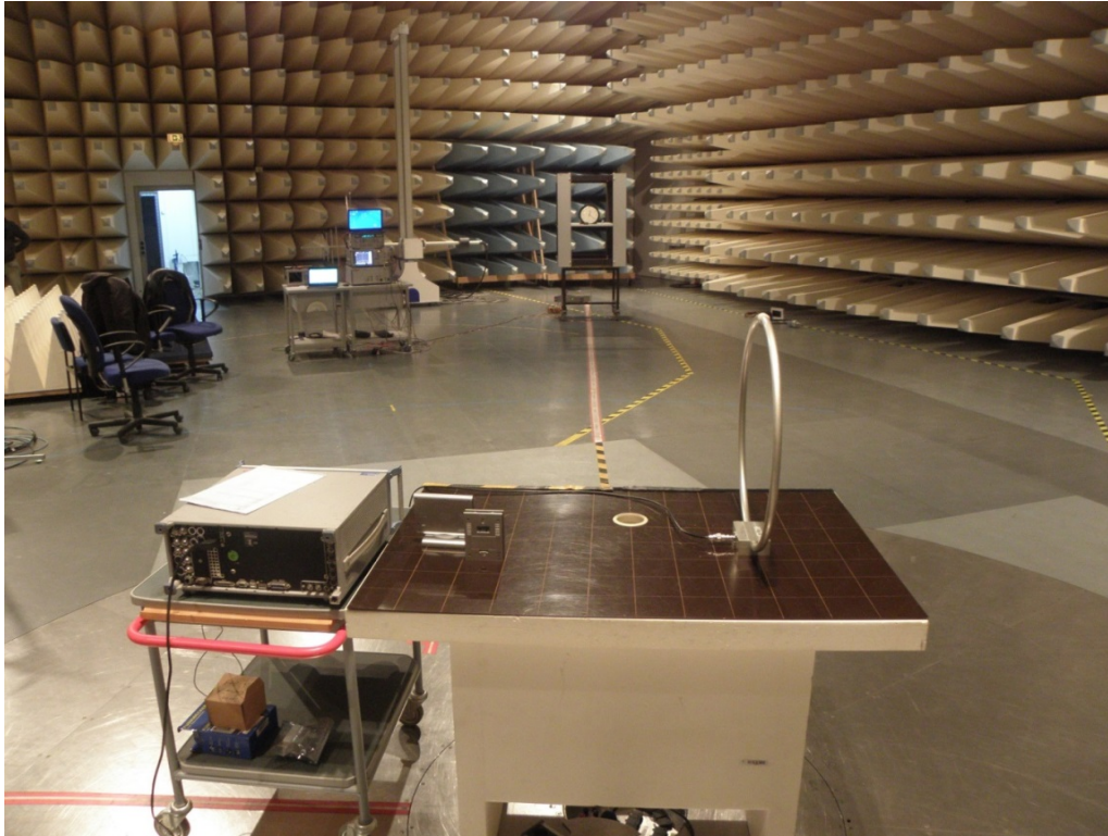
Figure 43: Measurement setup. Front: Wanted DCF77 signal generation Background: Helmholtz coil with DUT
