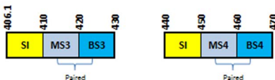
Figure 1: Illustrative mobile service allocations in the 400 MHz range: Simplex (SI) and paired Mobile station (MS) Base station (BS) use
