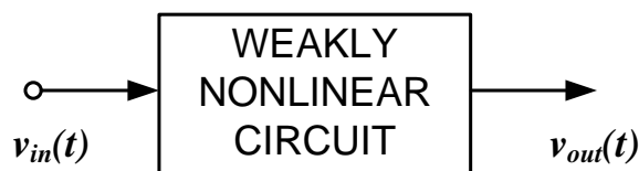
Figure 13: Weakly nonlinear circuit model for Volterra-Series analysis
