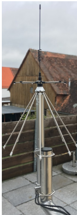
Figure 18: Wideband discone Antenna
