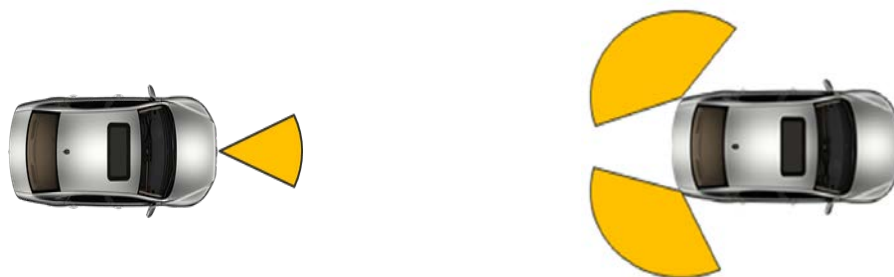
Figure 27: Representation of the mounting positions of a front-looking long range radar system (left) and a rear looking short range radar system (right)
