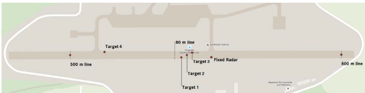
Figure 26: Display of the runway and the test-setup during the field test
