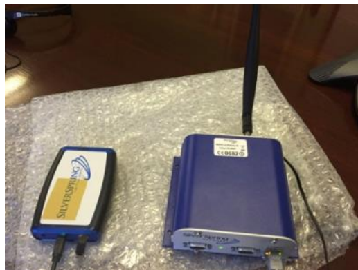
Figure 56: SSN Field Service Unit and Bridge
