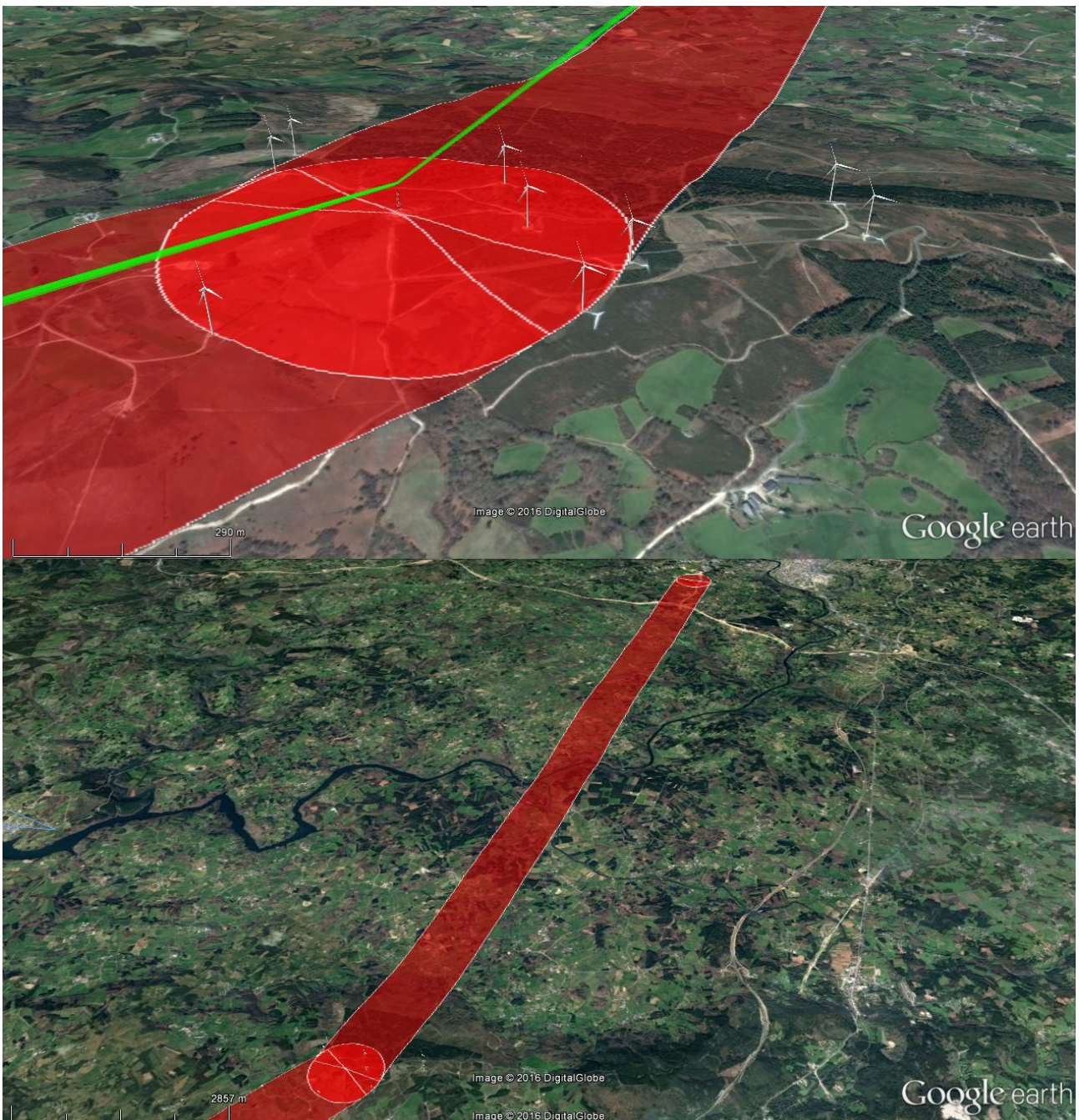
Figure 39: Above: in green, representation of the 2nd Fresnel ellipsoid of each radio link; in red, coordination area for each radio link. Below, coordination area for the whole extension of one of the fixed radio links [28]
