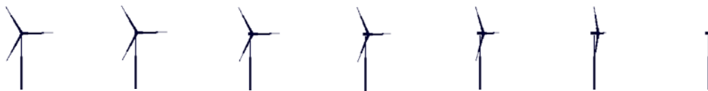
Figure 17: Example a turbine projection, shown for different rotor axis direction, and the same rotor position
