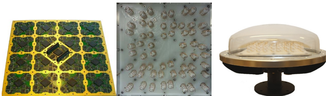
Figure 2: MBR transmitter/receiver board and antenna board with helical antennas
