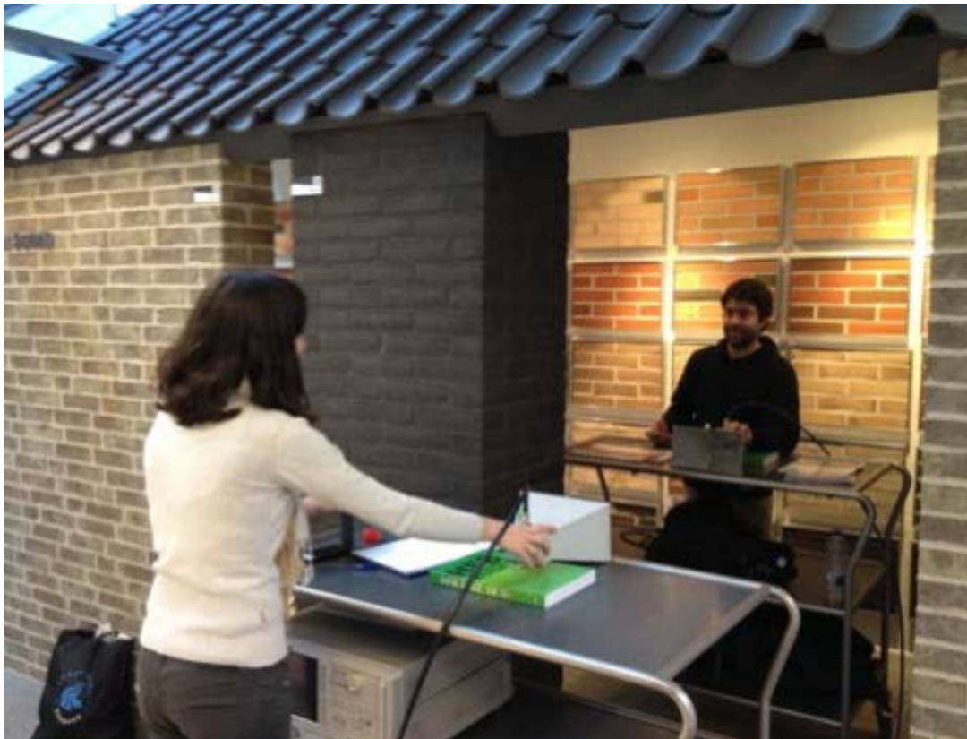
Figure 70: Measurement of the "reference Loss" without any material between the antennas
