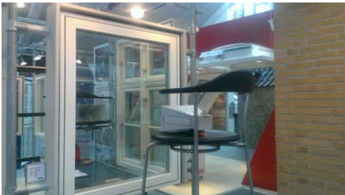
Figure 69: Measurement of the insertion Loss of a coated window at "Middelfart Bygge Centrum"
