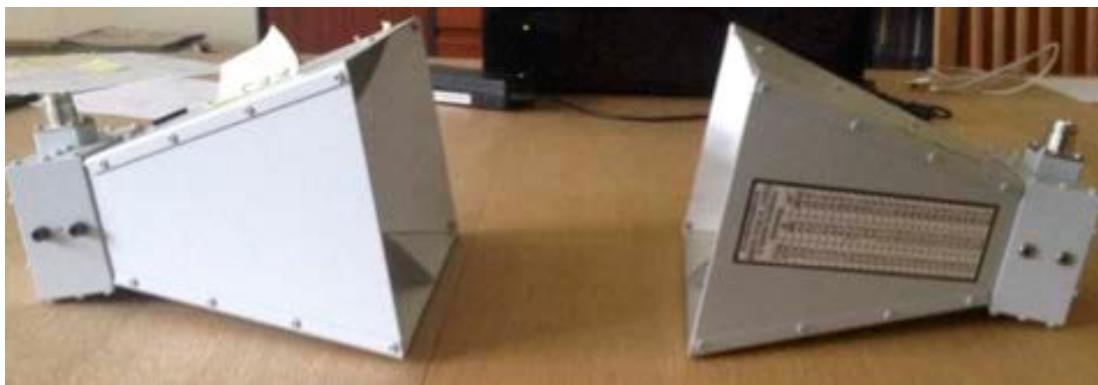
Figure 67: Horn antennas ensure a focused measurement beam reducing surrounding reflections
