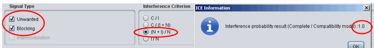
Figure 102: Probability of interference considering the impact of unwanted emissions and the receiver blocking response
