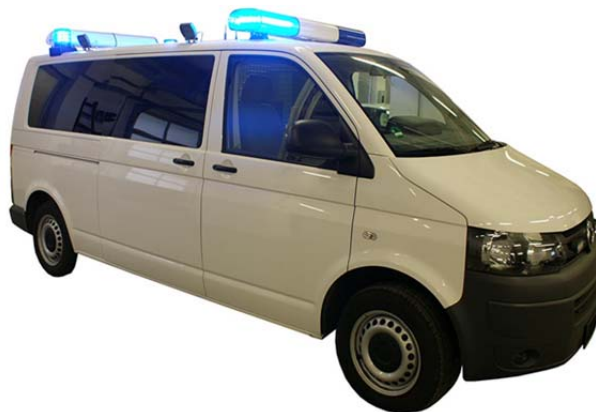
Figure 10: Typical mobile enforcement vehicle, RSU antennas are mounted on top of the roof in the back of the vehicle
