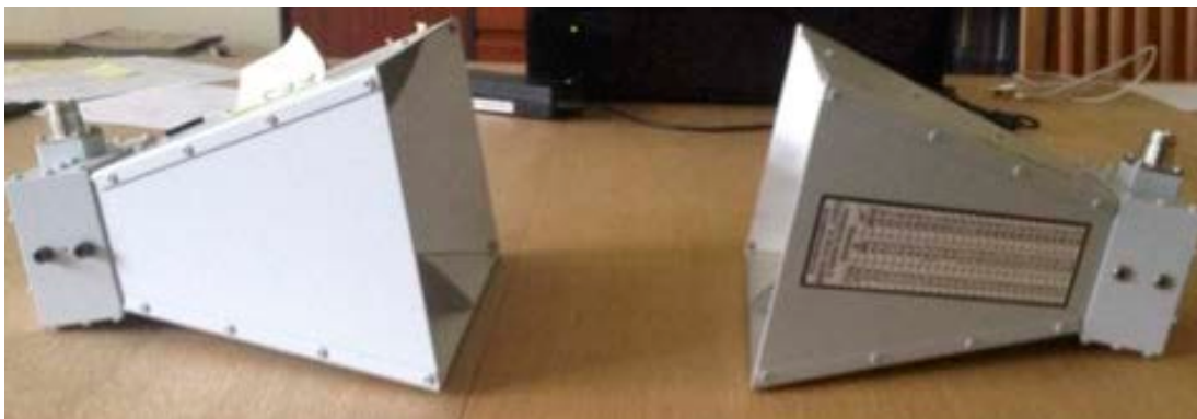
Figure 51: Horn antennas ensure a focused measurement beam reducing surrounding reflections
