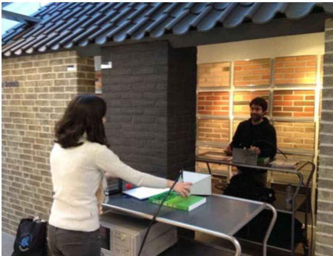
Figure 54: Measurement of the "reference Loss" without any material between the antennas
