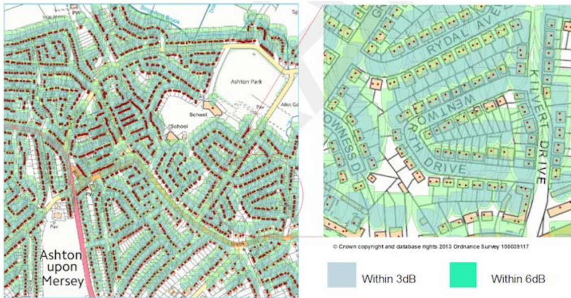
Figure 30: Sample suburban area mapping with 3 dB and 6 dB minimum coupling footprints overlaid
