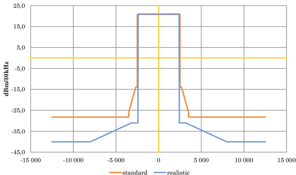
**Figure 3: UMTS/LTE emission masks, at antenna connector**
