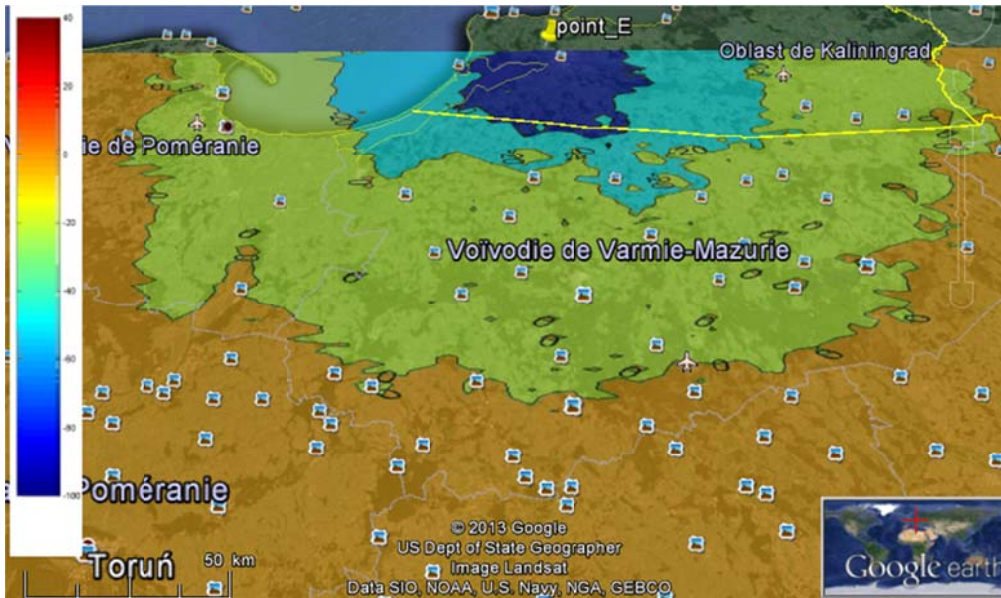
Figure 21: Iso additional required pathloss to protect case E telemetry station (Poland cross-border)
