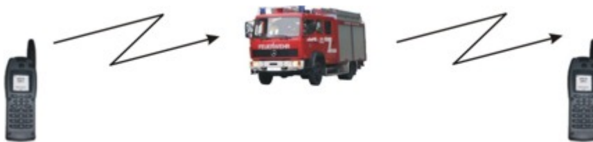
Figure 12: Network range extension for direct communications
