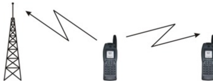
Figure 11: Simultaneous connection to the WAN and to direct communications
