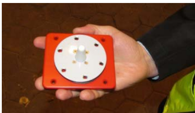
Figure 19: Aircraft OBU (prototype) and aircraft antenna (hand sized)
