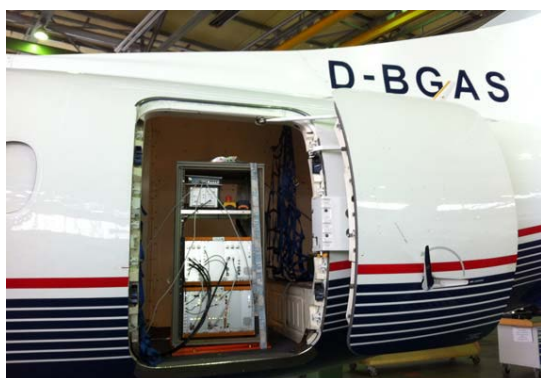
Figure 19: Aircraft OBU (prototype) and aircraft antenna (hand sized)
