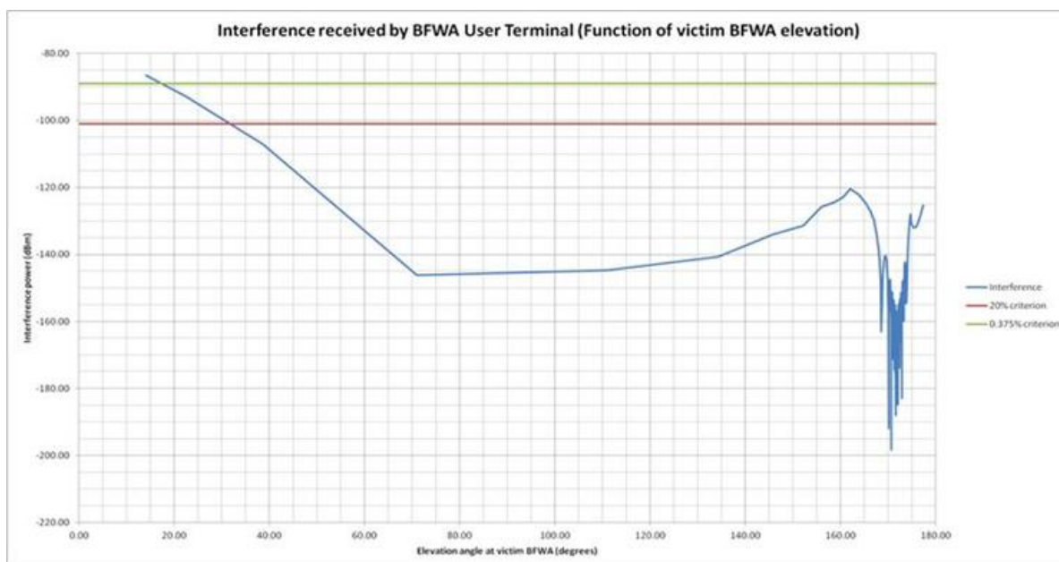
Figure 167: Interference received at worst case location BFWA User Terminal (65 km offset from DA2GC Ground Station) with reference to BFWA User Terminal elevation angle.
