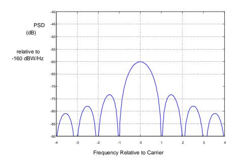
Figure A 1.1: Spectrum of GPS C/A-Code Signal
