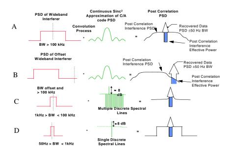
Figure A 1.2: Model of Correlation for varying Interfering Bandwidth
