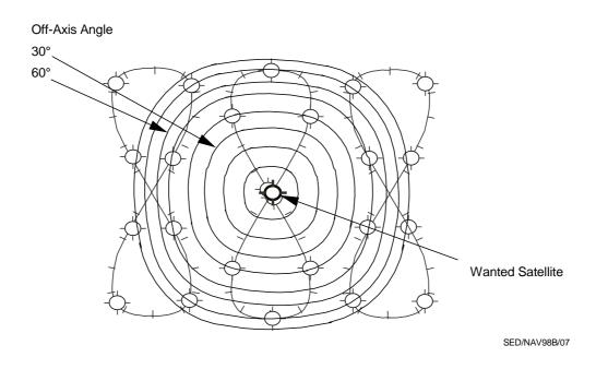
Figure A 2.3 : MES Interference from E-NSS-1 for worst-case MSS location
