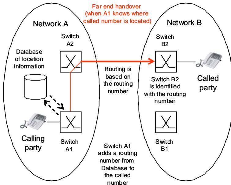
**Figure 5: Routing between networks when location information is shared**
