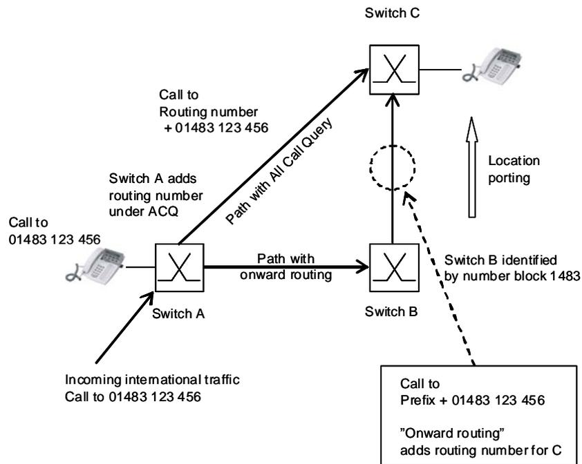
**Figure 3: Alternative methods of providing location portability within a network**
