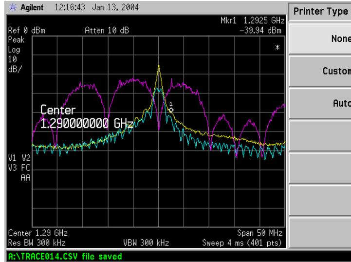
Figure 40: Spectrum of WPR and interferer, WPR at null E
