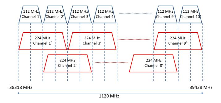
Figure 3: Channel arrangement and identifiers with channel width of 224 MHz (upper half of band)
