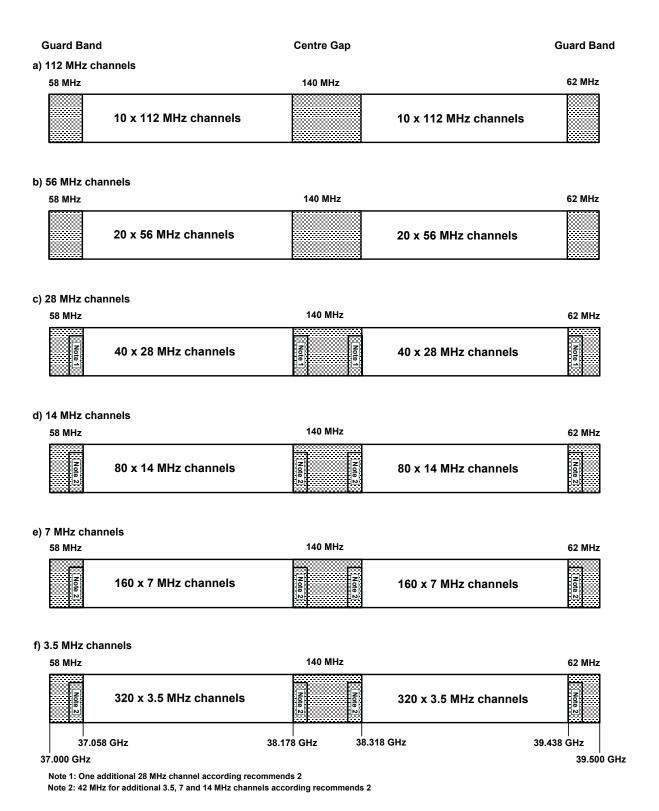
Figure 1: Occupied spectrum 37.0-39.5 GHz band
