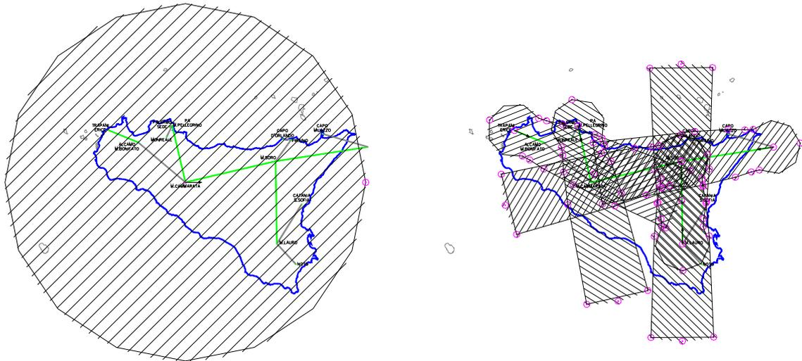
**Figure 87: Respected area to protect a P-P type 2 receiver in Sicily in the case of co-channel sharing (on the left) and in the case of  $\Delta f = 17.5$  MHz (on the right)**
