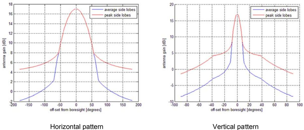
**Figure 14: ITU-R Recommendation F.1336-3 sector antenna patterns, 17 dBi maximum gain, 65 degrees 3 dB beamwidth. Average (blue) and peak (red) side lobe patterns**
