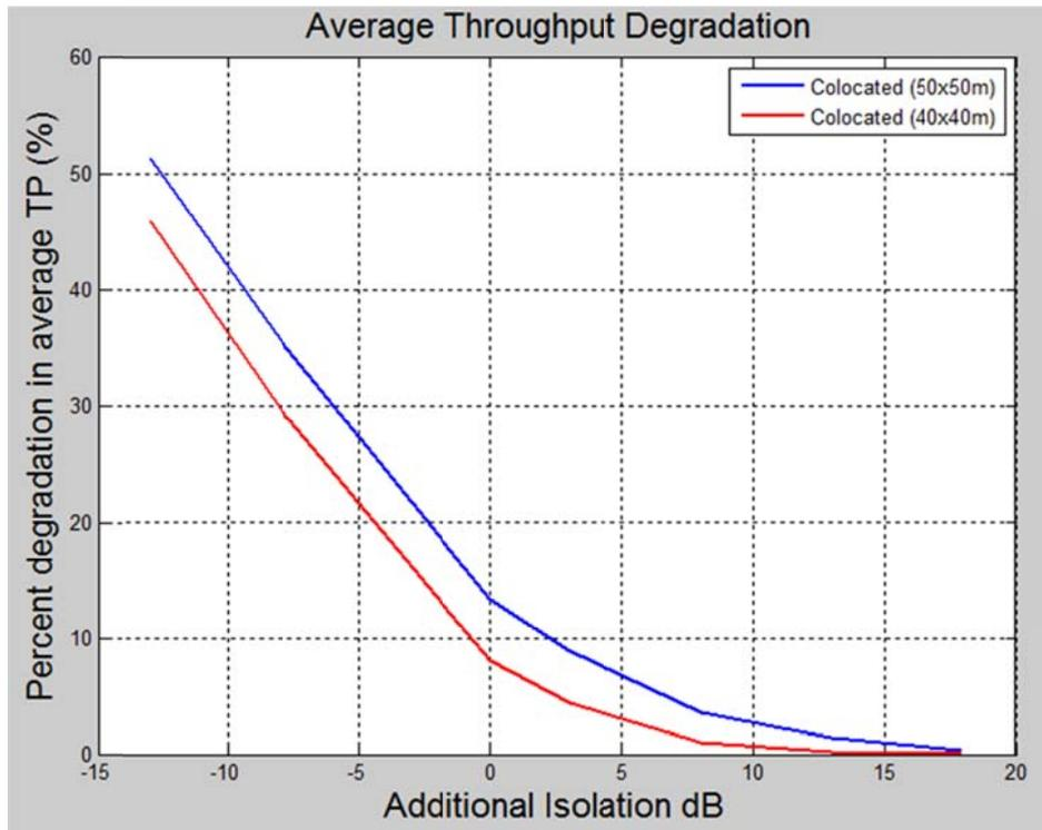
Figure 72: Average throughput degradation (Micro – pico scenario)
