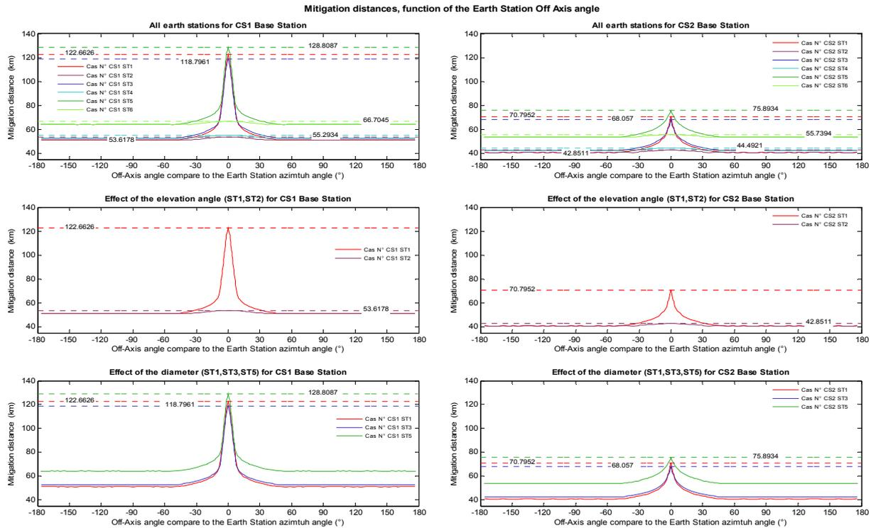
**Figure 73: Influence of the FSS ES and BWA CS parameters on the mitigation area**
