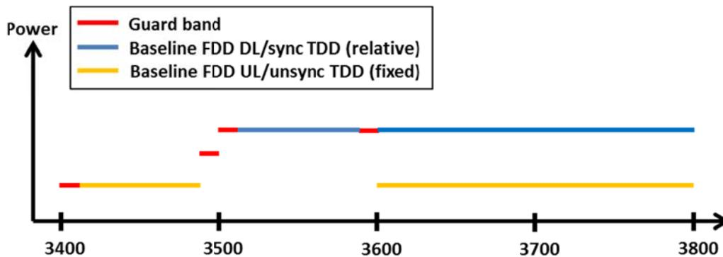
**Figure 28: Schematic description of baseline and guard band power levels for a mixed FDD and TDD allocation. In the case of synchronised TDD, it is assumed that all blocks are synchronised.**
