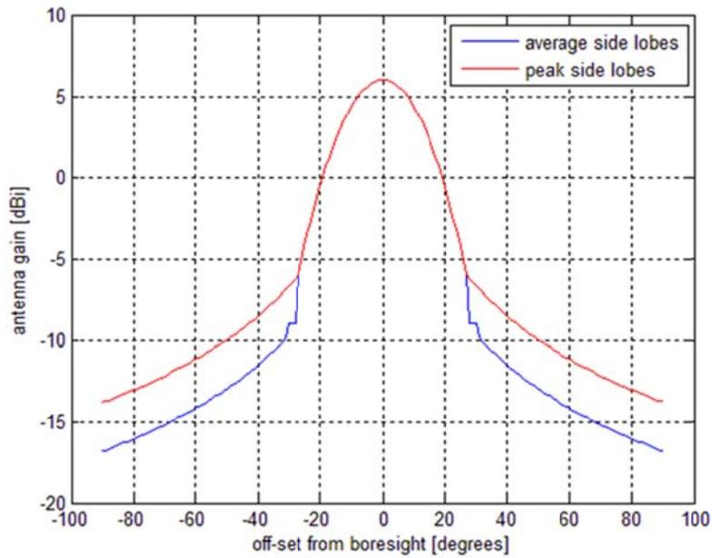
**Figure 13: ITU-R Recommendation F.1336-3 omni antenna patterns, vertical dimension, for 6 dBi maximum gain. Average (blue) and peak (red) side lobes**
