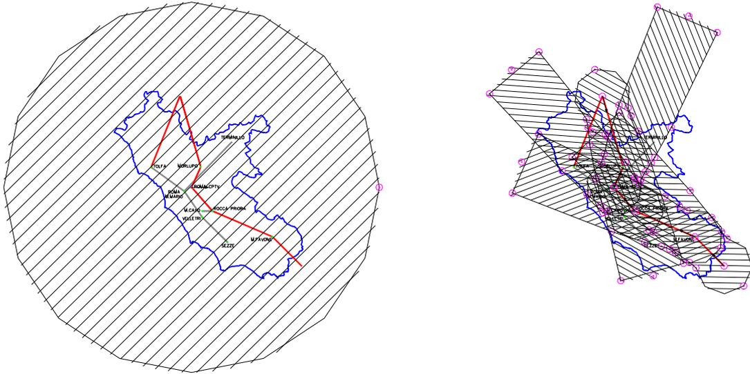
**Figure 85: Respected area to protect a P-P type 2 interfered receiver near Rome (Lazio region) in the case of co-channel sharing (on the left) and in the case of  $\Delta f = 17.5$  MHz (on the right)**
