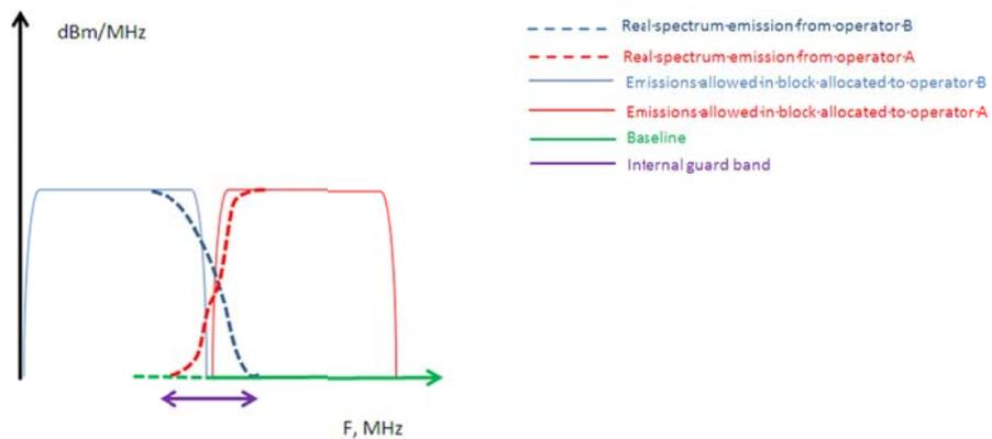
**Figure 37: Licensing approach with no frequency separation between the block edges of two adjacent unsynchronised TDD networks**
