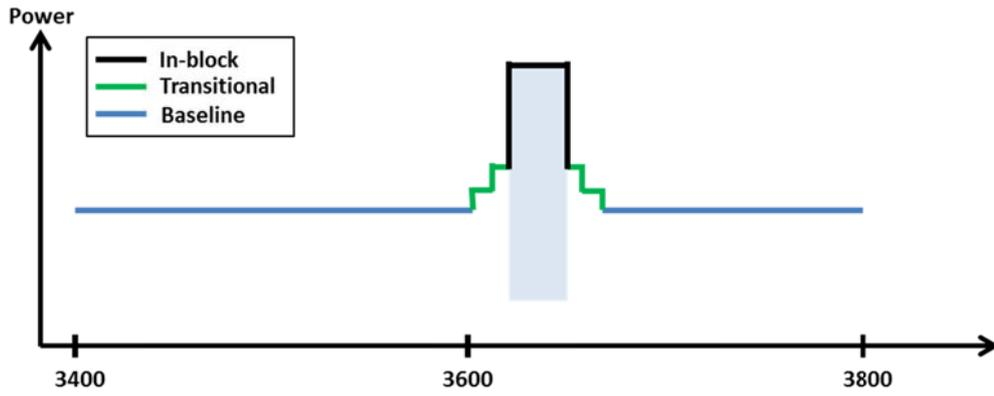
Figure 33: Combined BEM elements for a TDD block in a TDD only allocation with synchronisation between all the operators
