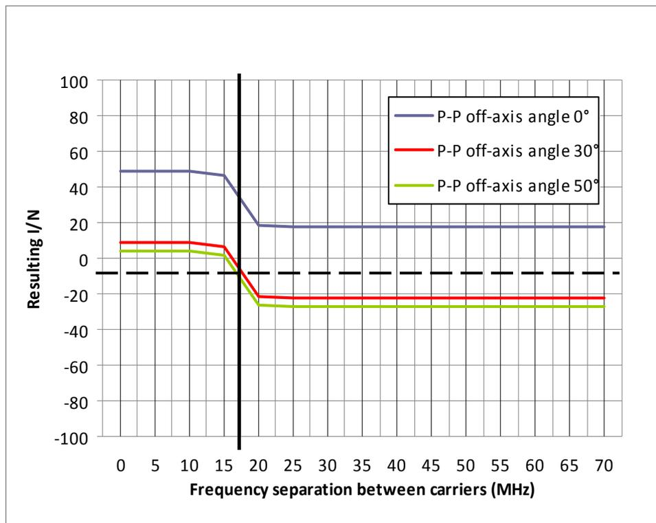
**Figure 83: Interference from a P-P link to a UE with a 2 km separation distance**
