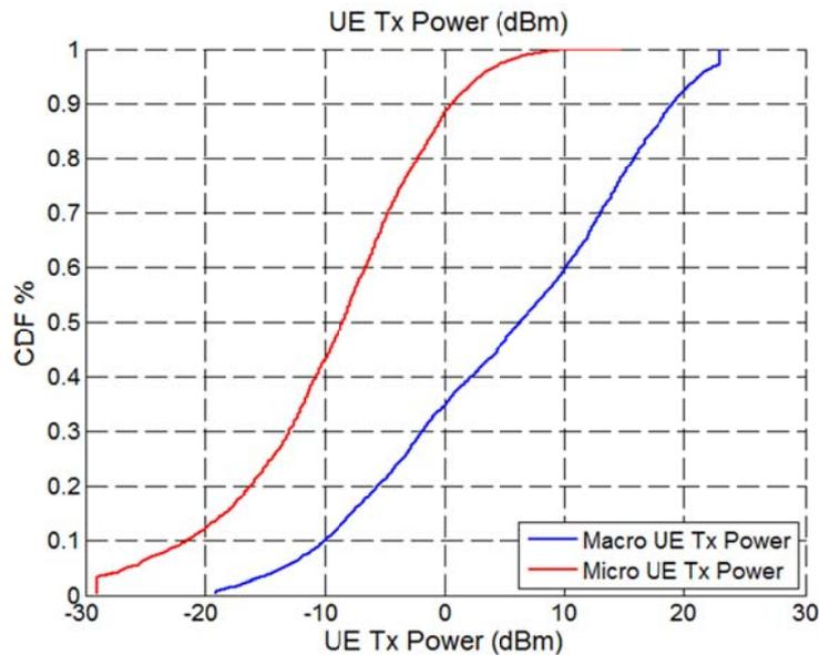
**Figure 59: Uplink transmit power of the UEs**
