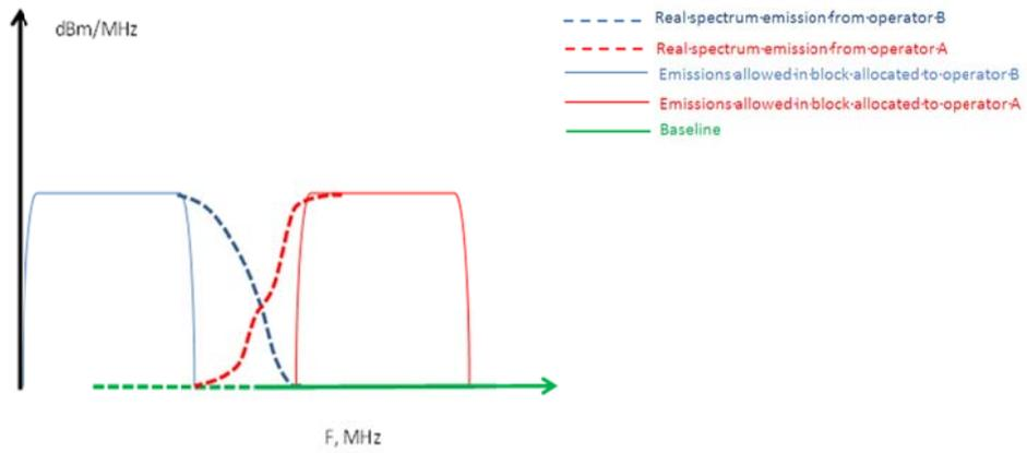
**Figure 38: Licensing approach with separation between the block edges of the two adjacent operators**
