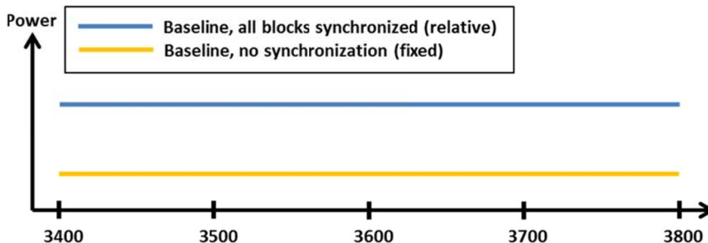
**Figure 49: Schematic description of baseline levels for a TDD-only allocation. In the case of synchronised TDD, it is assumed that all blocks are synchronised.**
