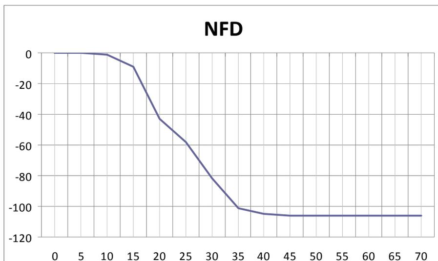
**Figure 16: NFD function used in the sharing studies with BWA interfering a P-P type 2 system**
