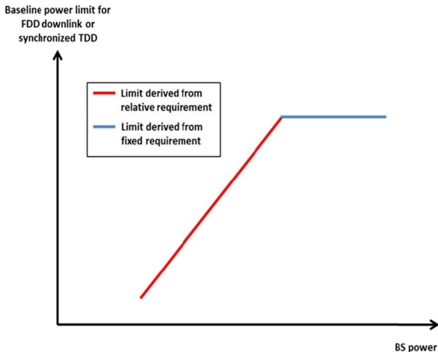
**Figure 26: Combining the relative and the fixed limit for the baseline applying to FDD DL spectrum and to synchronised TDD spectrum**
