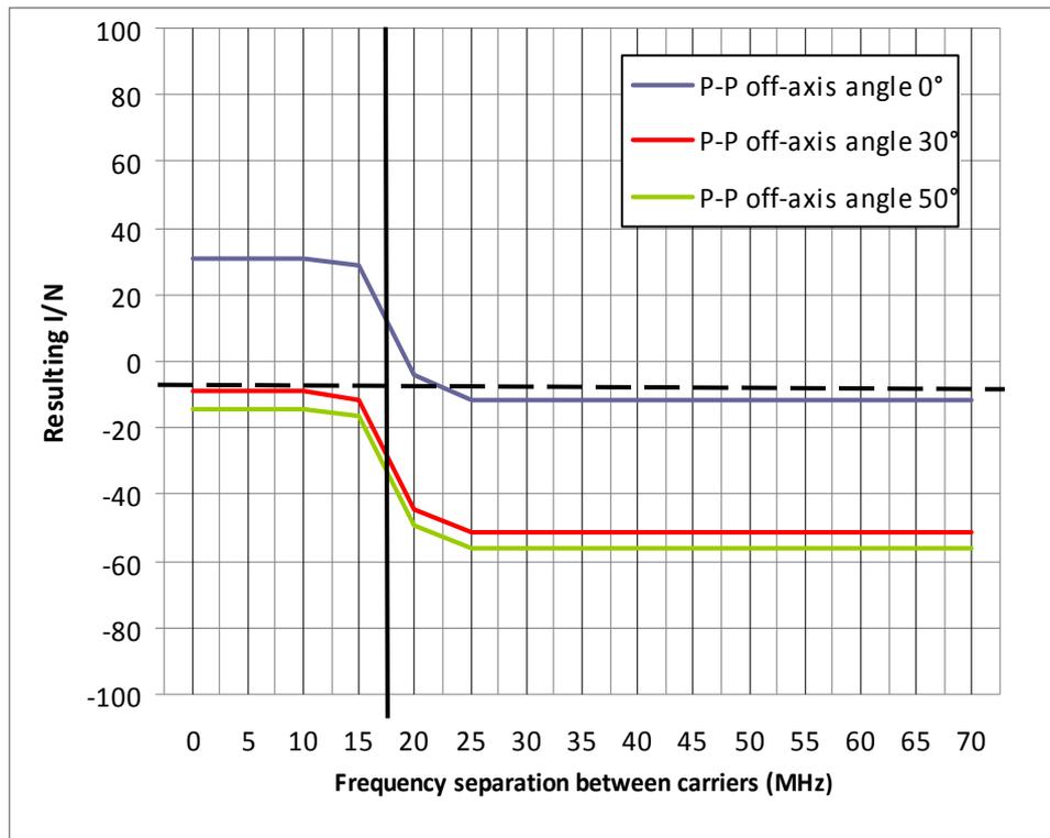
**Figure 82: Interference from a P-P link to a MFCN macrocell BS with a 20 km separation distance. P-P is in the back lobe of the MFCN BS sector antenna**
