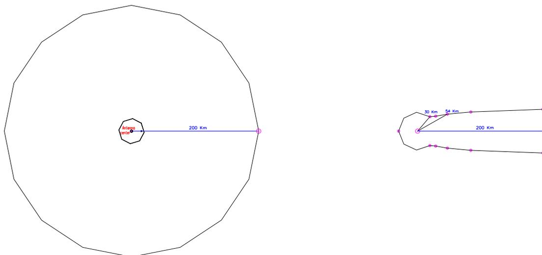
**Figure 84: Respected area to protect a P-P type 2 interfered receiver from an interfering MFCN macrocell BS in the case of co-channel sharing (on the left) and in the case of  $\Delta f = 17.5$  MHz (on the right)**
