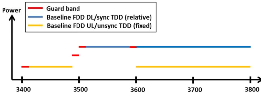
**Figure 50: Schematic description of baseline and guard band power levels for a mixed FDD and TDD allocation. In the case of synchronised TDD, it is assumed that all blocks are synchronised.**
