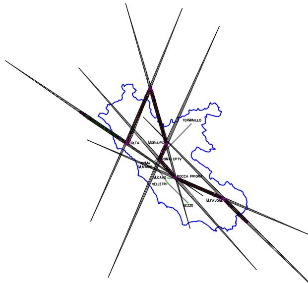
**Figure 89: Respected area to protect a P-P type 2 receiver near Rome (Lazio region) in the case in the case of  $\Delta f = 22.5$  MHz**
