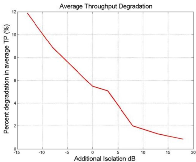
**Figure 64: Average throughput degradation - additional isolation - case 2 (50% indoor UEs)**
