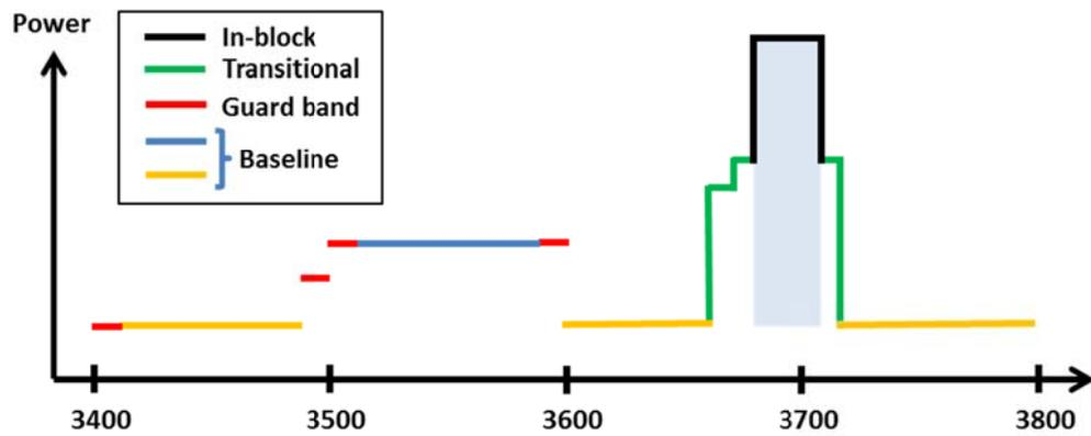
Figure 34: Combined BEM elements for a TDD block in an FDD and TDD allocation without synchronisation
