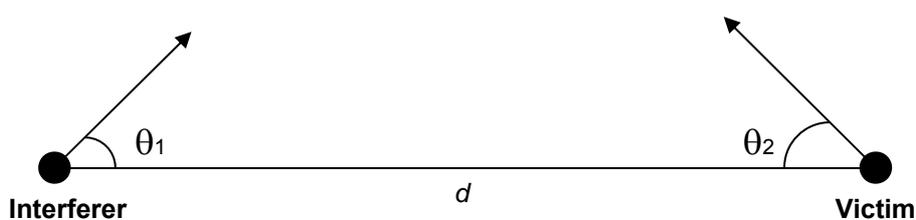
**Figure 74: Explanation of angles between interferer and victim**
