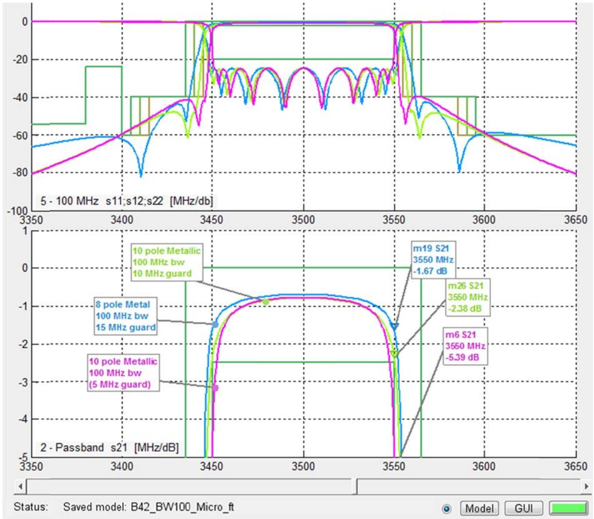
Figure 43: Micro base station 100 MHz bandwidth
