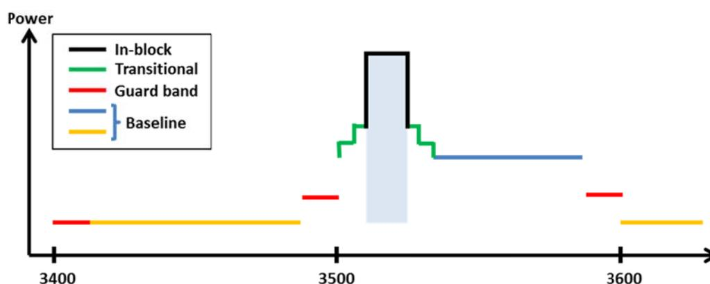
**Figure 5: Combined BEM elements for an FDD block starting at 3510 MHz**
