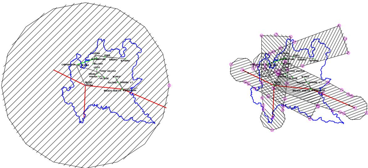
**Figure 86: Respected area to protect a P-P type 2 receiver near Milan (Lombardia region) in the case of co-channel sharing (on the left) and in the case of  $\Delta f = 17.5$  MHz (on the right)**
