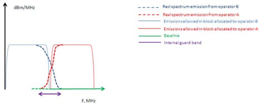
**Figure 7: Licensing approach with no frequency separation between the block edges of two adjacent unsynchronised TDD networks**
