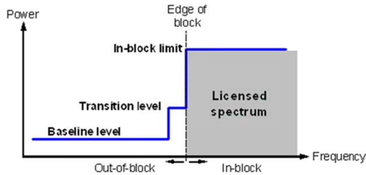
**Figure 47: Illustration of a general block-edge mask**
