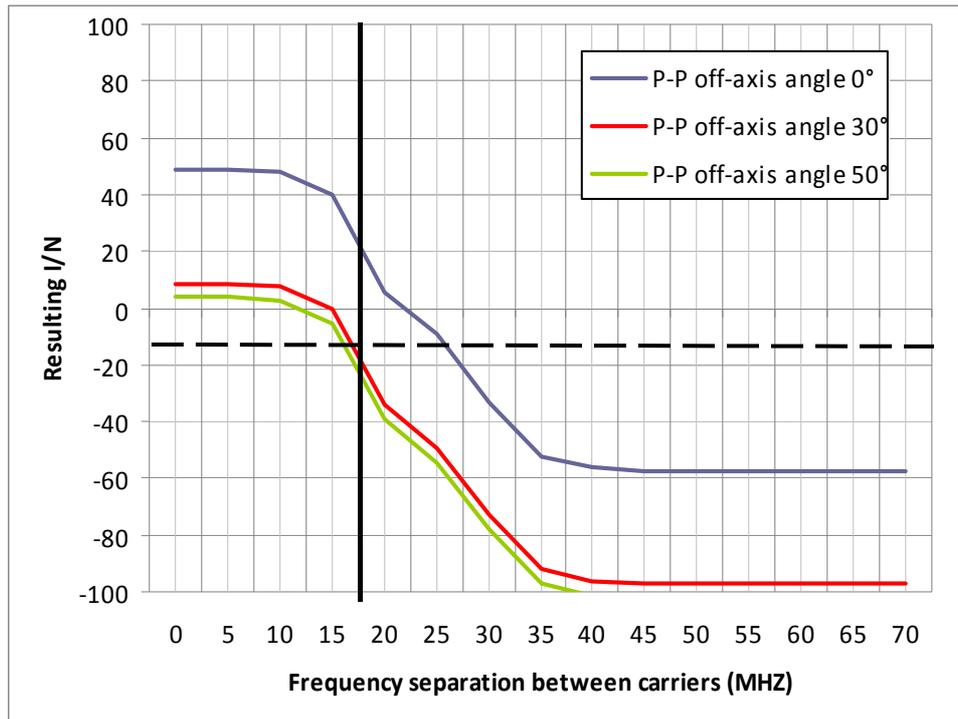
**Figure 78: Interference from a UE to a P-P receiving site with a 2 km separation distance.**
