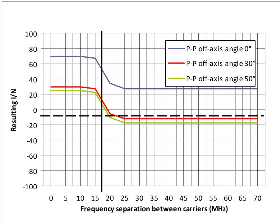
Figure 80: Interference from P-P link to an MFCN macrocell BS with a 2 km separation distance. P-P is in the main lobe of the MFCN BS sector antenna.
