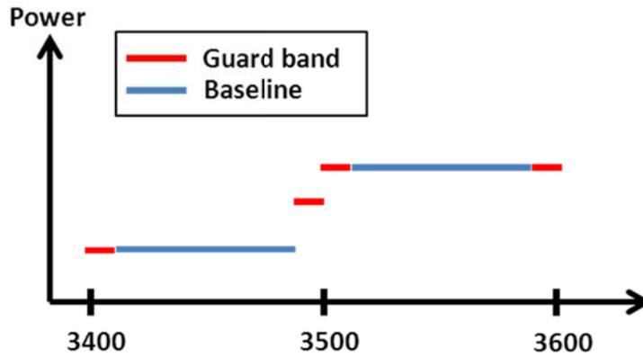
Figure 31: Guard bands in an FDD allocation
