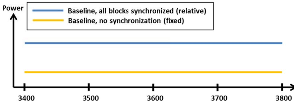
**Figure 27: Schematic description of baseline levels for a TDD-only allocation. In the case of synchronised TDD, it is assumed that all blocks are synchronised.**
