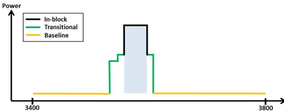
Figure 32: Combined BEM elements for a TDD block in a TDD only allocation without synchronisation, 10 MHz transitional region below and 5 MHz transitional region above
