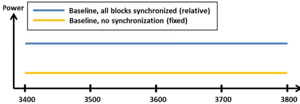
**Figure 3: Schematic description of baseline levels for a TDD-only allocation. In the case of synchronised TDD, it is assumed that all blocks are synchronised.**
