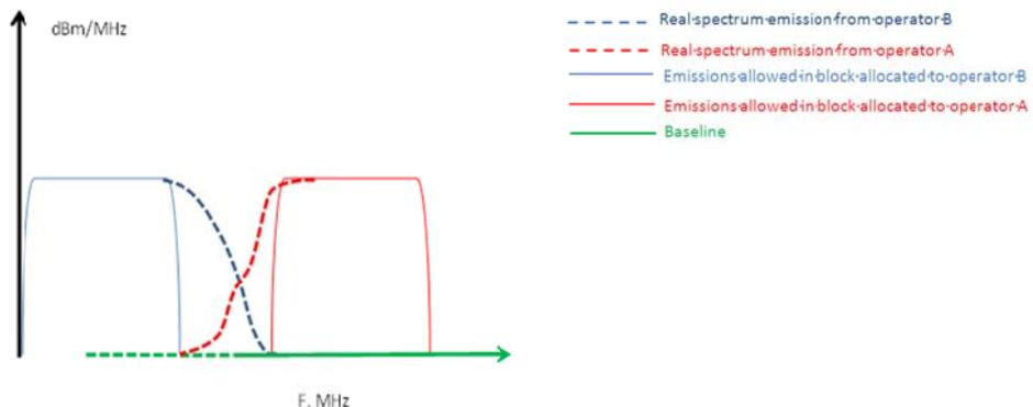
**Figure 8: Licensing approach with separation between the block edges of the two adjacent operators**
