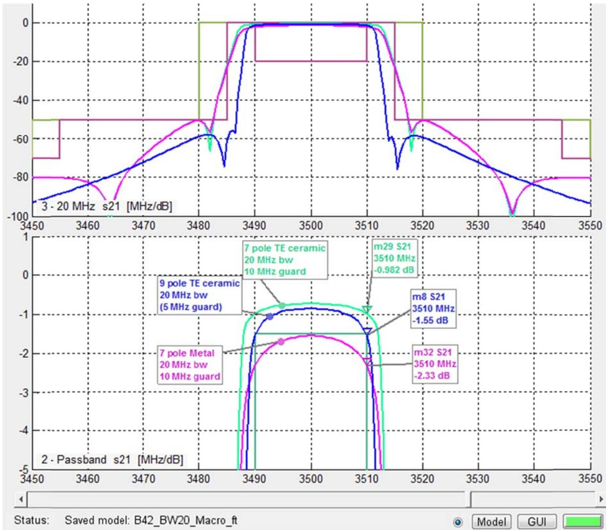
Figure 40: Macro base station, 20 MHz bandwidth
