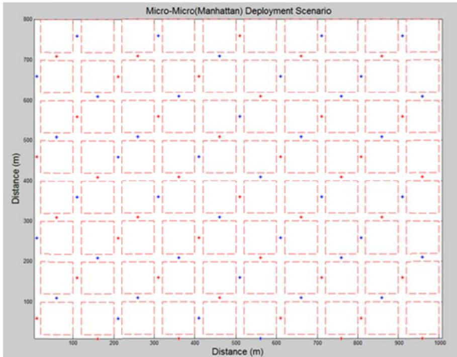
**Figure 22: Micro – micro deployment scenario (Manhattan)**
