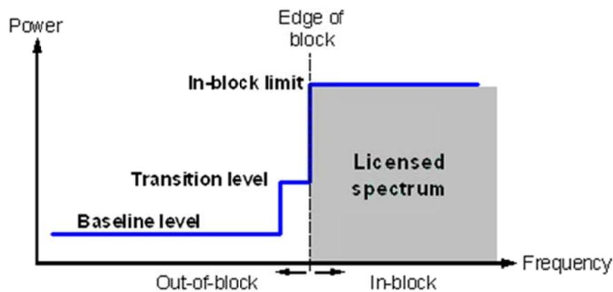
**Figure 25: Illustration of a general block-edge mask**
