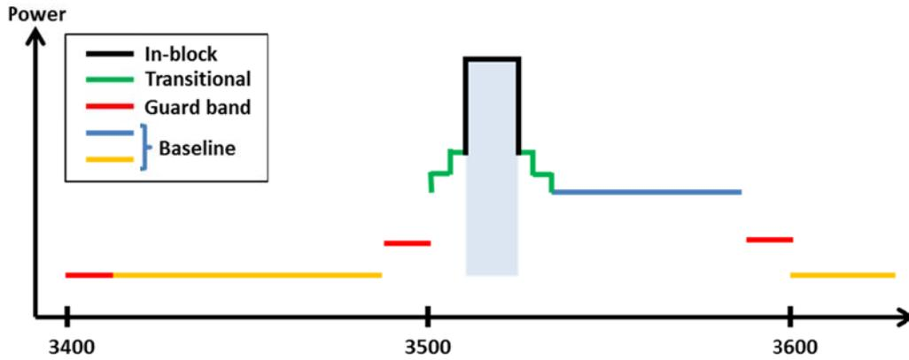
**Figure 51: Combined BEM elements for an FDD block starting at 3510 MHz**
