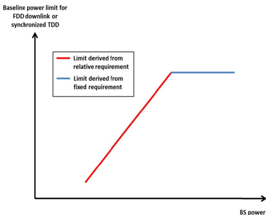
**Figure 2: Combining the relative and the fixed limit for the baseline applying to FDD DL spectrum and to synchronised TDD spectrum**
