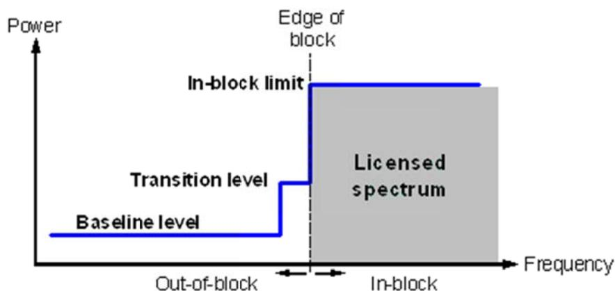
**Figure 1: Illustration of a general block-edge mask**
