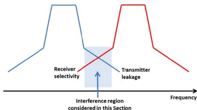
**Figure 17: Interference as a result of limited ACLR and ACS**
