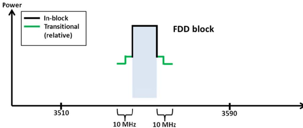
**Figure 30: In-block and transitional regions for an FDD block**
