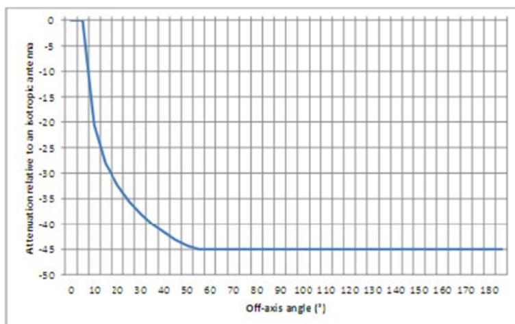
**Figure 15: P-P systems antenna diagram with 39 dBi antenna gain modelled with the Recommendation ITU-R F.699.5. This is a typical antenna 3 meter diameter**
