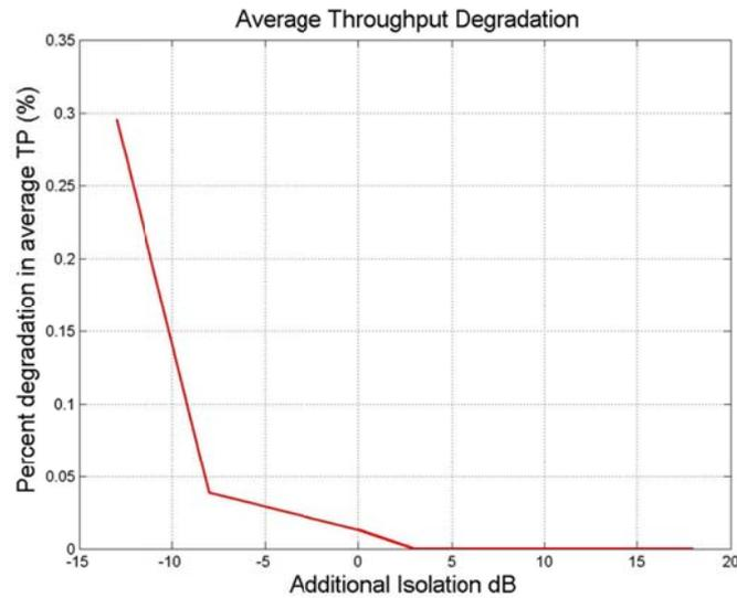
**Figure 63: Average throughput degradation - additional isolation - case 1 (100% indoor UEs)**
