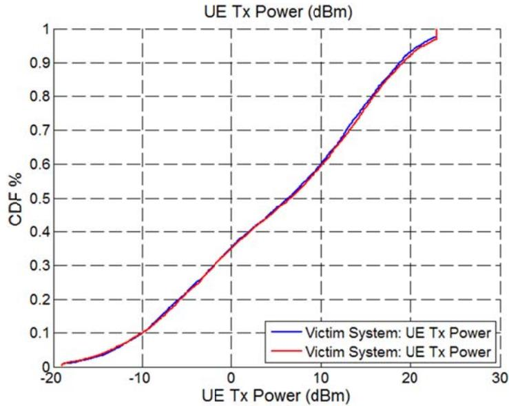
**Figure 57: Uplink transmit power of the UEs**
