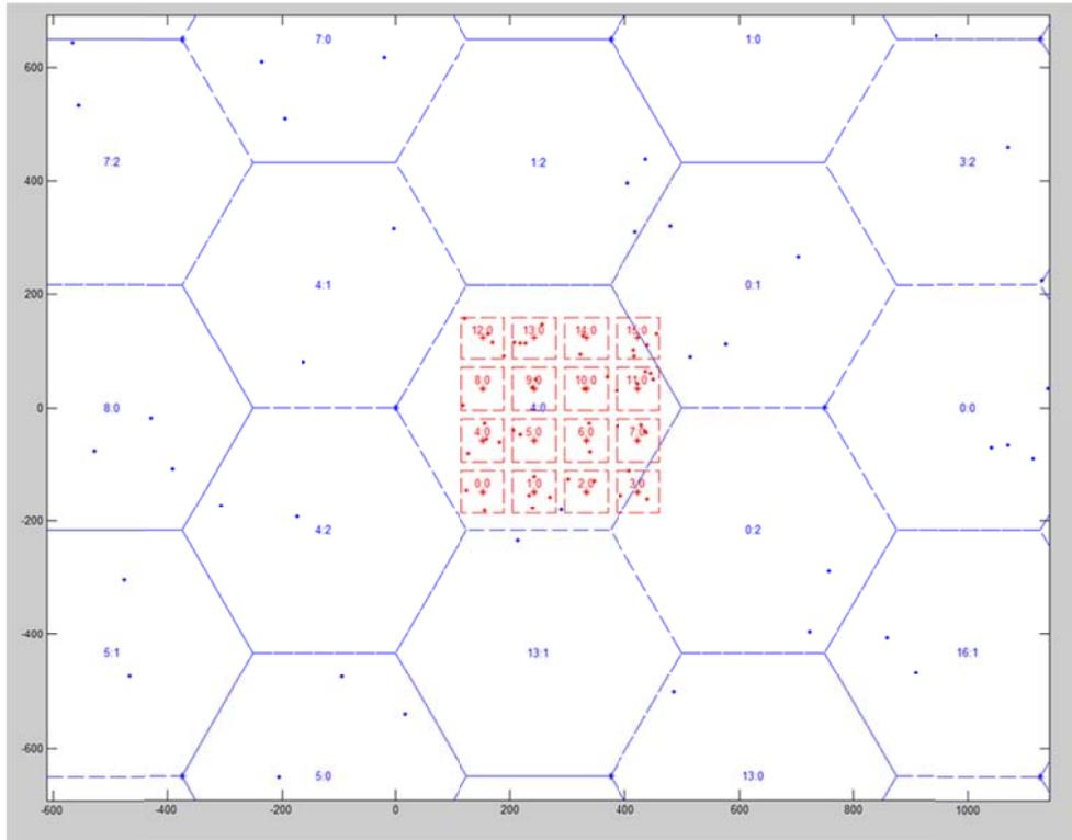
**Figure 62: Deployment for macro-to-indoor micro scenario**
