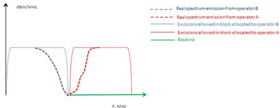
**Figure 52: Licensing approach with no frequency separation between the block edges of two adjacent unsynchronised TDD networks**
