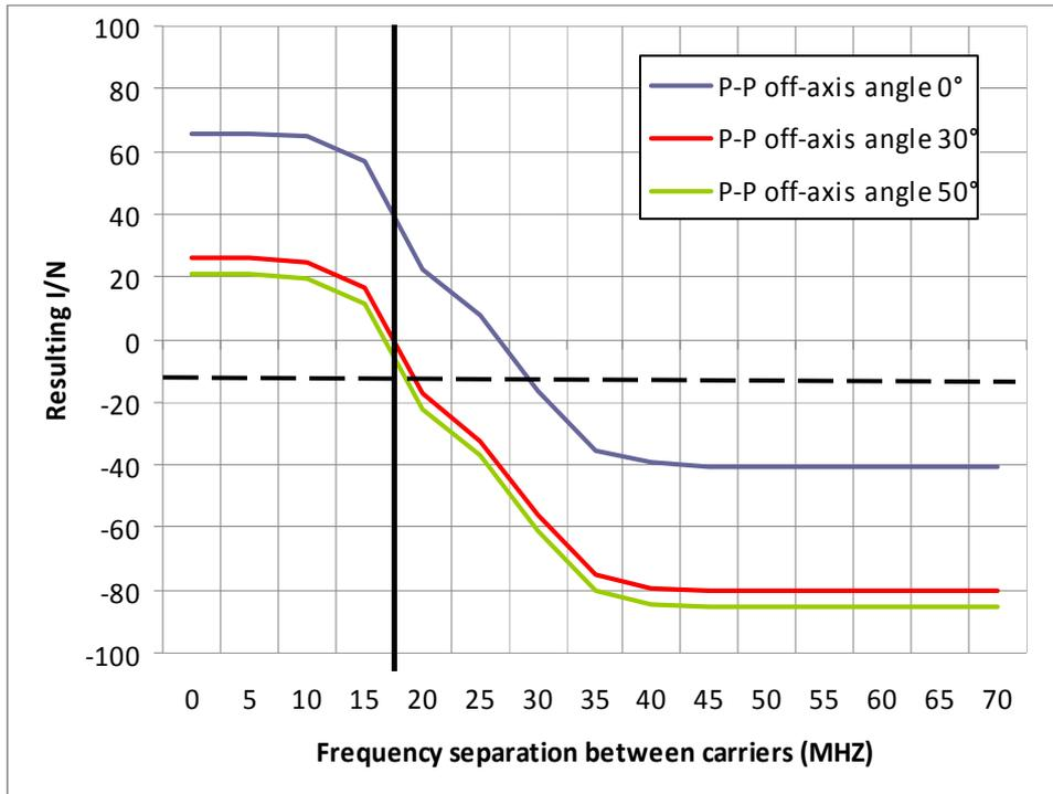
**Figure 76: Interference from an MFCN macrocell BS to a P-P receiving site with a 20 km separation distance. P-P is in the main lobe of the MFCN BS sector antenna**
