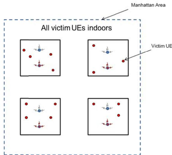
**Figure 23: Configuration for the non-co-located cases 1 & 2**
