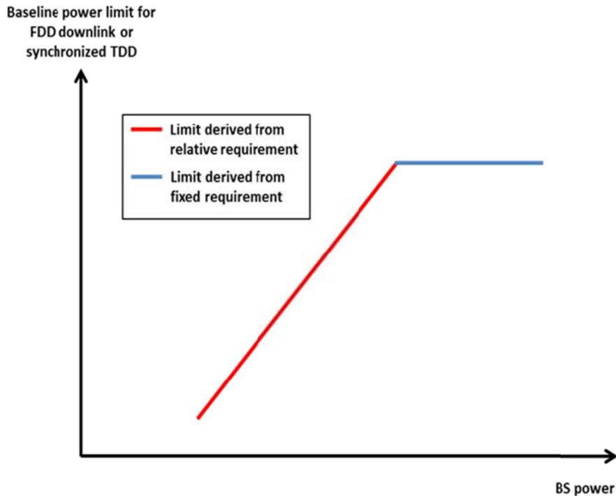
**Figure 48: Combining the relative and the fixed limit for the baseline applying to FDD DL spectrum and to synchronised TDD spectrum**
