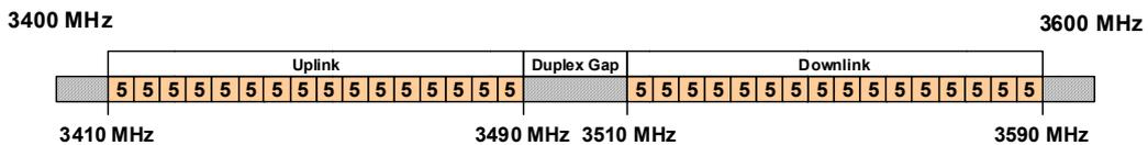
**Figure 45: Frequency arrangement for the 3400-3600 MHz band based on FDD**
