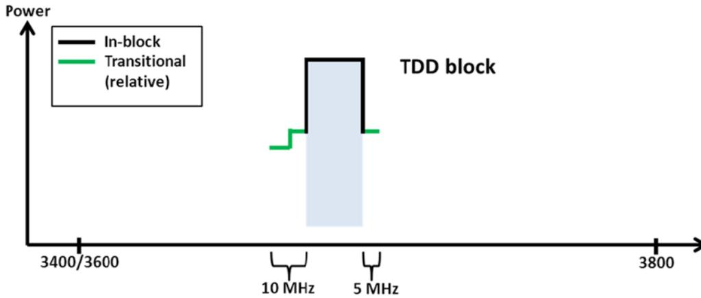
**Figure 29: In-block and transitional regions for a TDD block with 10 MHz transitional region below and 5 MHz transitional region above**
