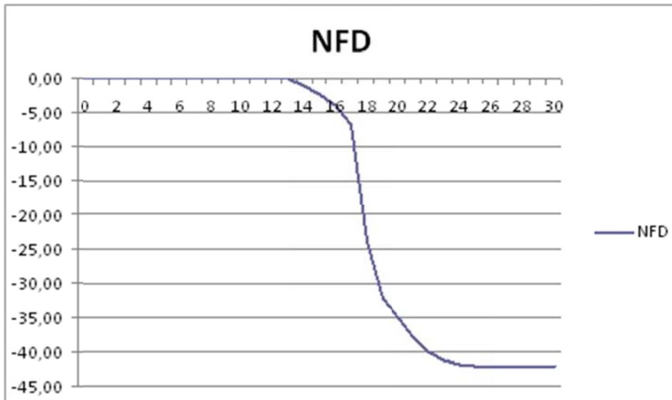
**Figure 79: NFD function used in the sharing studies with P-P type 2 (30 MHz) interfering MFCN macrocell BS**
