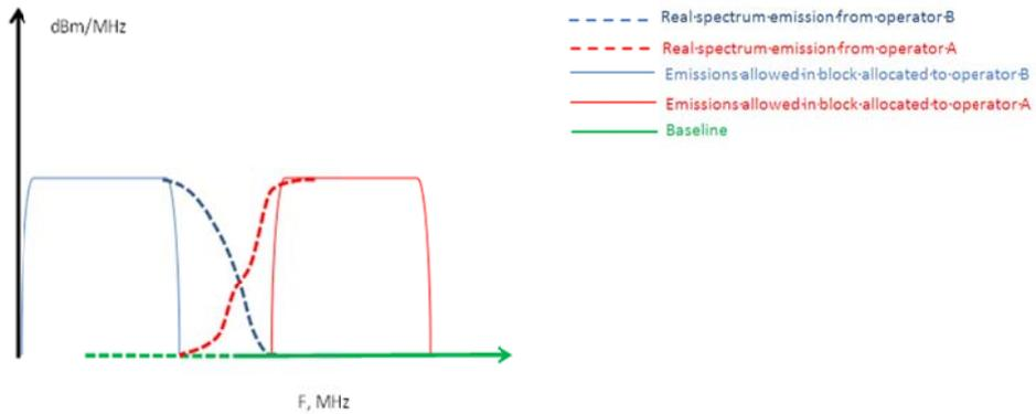
**Figure 54: Licensing approach with separation between the block edges of the two adjacent operators**
