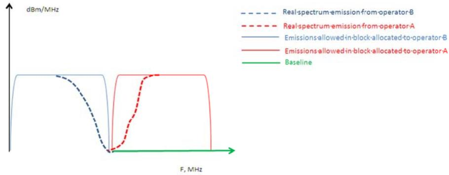
**Figure 6: Licensing approach with no frequency separation between the block edges of two adjacent unsynchronised TDD networks**
