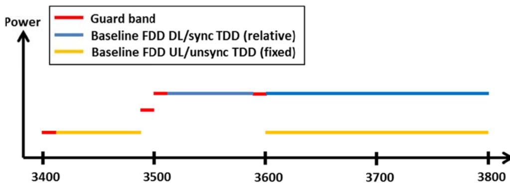
**Figure 4: Schematic description of baseline and guard band power levels for a mixed FDD and TDD allocation. In the case of synchronised TDD, it is assumed that all blocks are synchronised.**
