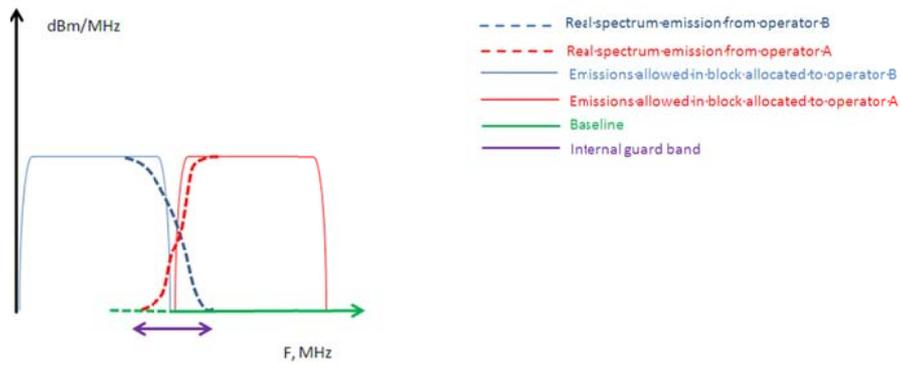
**Figure 53: Licensing approach with no frequency separation between the block edges of two adjacent unsynchronised TDD networks**
