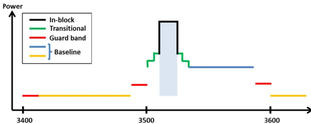
Figure 35: Combined BEM elements for an FDD block starting at 3510 MHz
