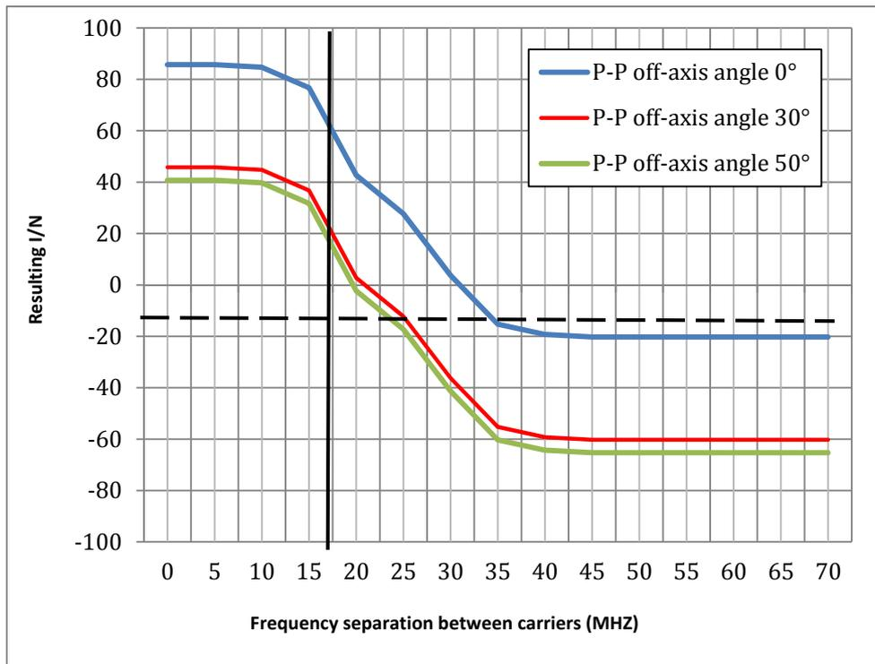
**Figure 75: Interference from an MFCN macrocell BC to a P-P receiving site with a 2 km separation distance. P-P is in the main lobe of the MFCN BS sector antenna**
