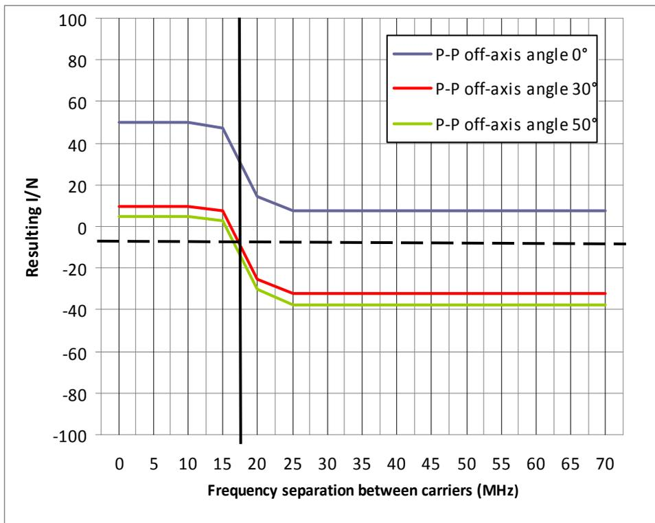
Figure 81: Interference from a P-P link to an MFCN macrocell BS with a 20 km separation distance. P-P is in the main lobe of the MFCN BS sector antenna
