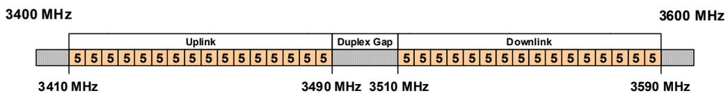
**Figure 11: Frequency arrangement for the 3400-3600 MHz band based on FDD**
