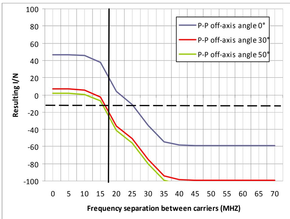
**Figure 77: Interference from an MFCN macrocell BS to a P-P receiving site with a 20 km separation distance. P-P is in the back lobe of the MFCN BS sector antenna ( $G_t=-2\text{dBm}$ )**
