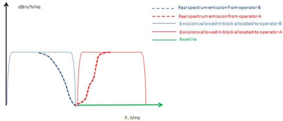
**Figure 36: Licensing approach with no frequency separation between the block edges of two adjacent unsynchronised TDD networks**
