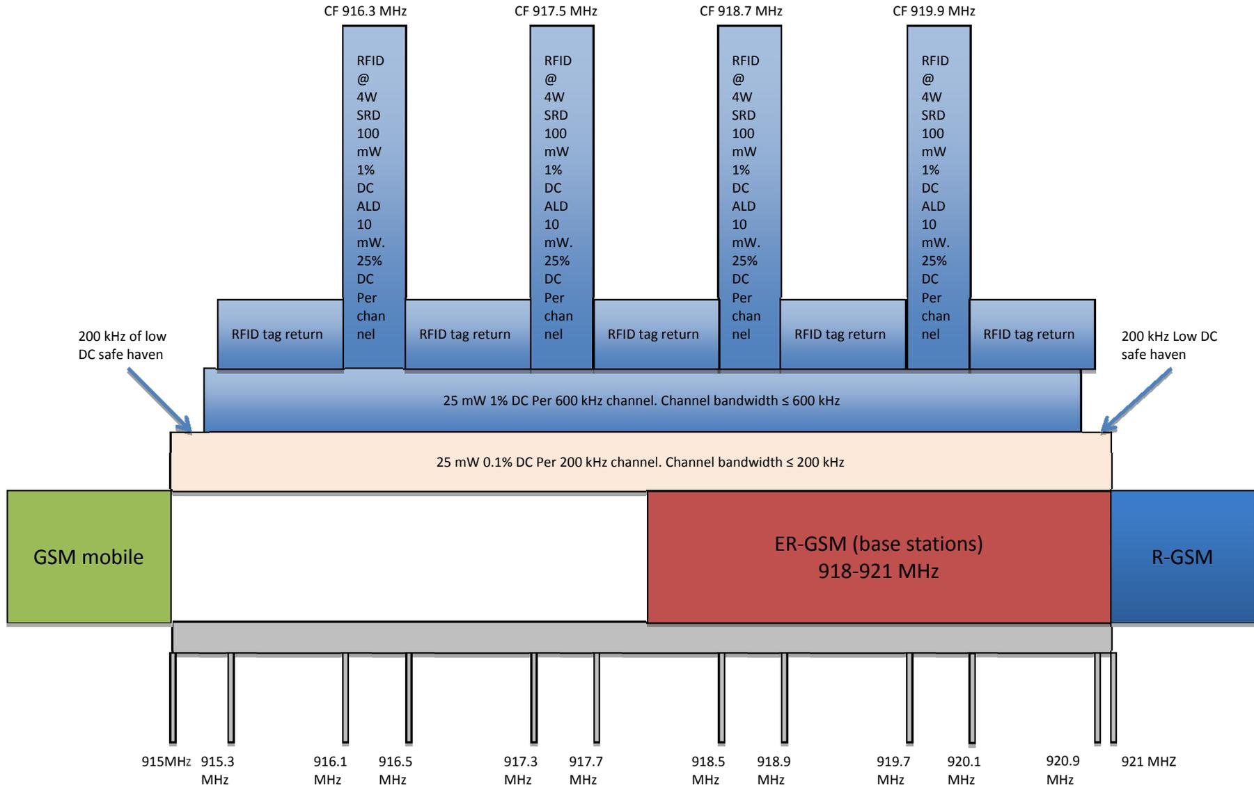
Figure 4: Band plan for 915-921 MHz
