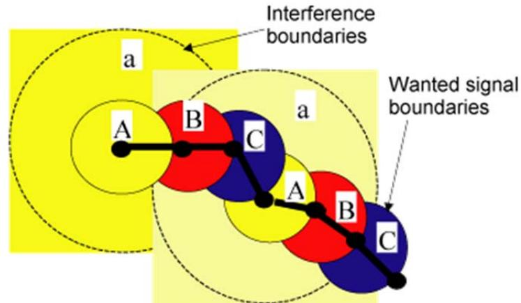
**Figure 12: Mesh node interference (each colour represents a different frequency channel)**
