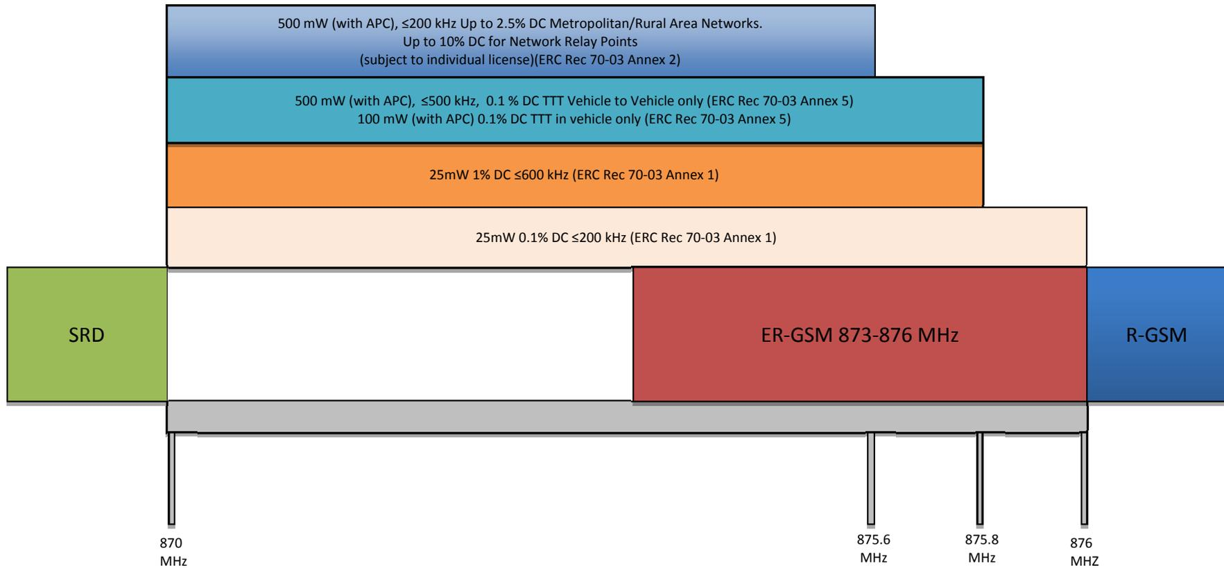
Figure 3: Band plan for 870-876 MHz
